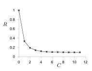
Figure 13.12. The rate R of the concatenated Hamming code as a function of the number of concatenations, C.
