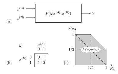
Figure 15.3. Multiple access channels. (a) A general multiple access channel with two transmitters and one receiver. (b) A binary multiple access channel with output equal to the sum of two inputs. (c) The achievable region.
