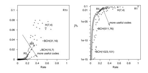
Figure 1.18. Error probability  $p_{\rm b}$  versus rate R for repetition codes, the (7, 4) Hamming code and BCH codes with block lengths up to 1023 over a binary symmetric channel with f = 0.1. The righthand figure shows  $p_{\rm b}$  on a logarithmic scale.
