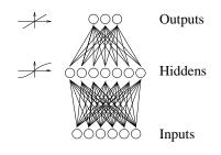
Figure 44.1. A typical two-layer network, with six inputs, seven hidden units, and three outputs. Each line represents one weight.
