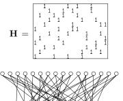
Figure 11.8. A low-density parity-check matrix and the corresponding graph of a rate-1/4low-density parity-check code with blocklength N = 16, and M = 12 constraints. Each white circle represents a transmitted bit. Each bit participates in j = 3constraints, represented by  $\pm$ squares. Each constraint forces the sum of the k = 4 bits to which it is connected to be even. This code is a (16, 4) code. Outstanding performance is obtained when the block length is increased to  $N \simeq 10\,000$ .
