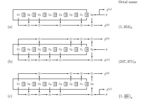
Figure 48.1. Linear feedback shift registers for generating convolutional codes with rate 1/2. The symbol  $\langle \underline{D} \rangle$  indicates a copying with a delay of one clock cycle. The symbol  $\oplus$  denotes linear addition modulo 2 with no delay.
