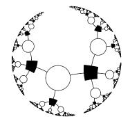
Figure 47.11. Local topology of the graph of a Gallager code with column weight j = 3 and row weight k = 4. White nodes represent bits,  $x_l$ ; black nodes represent checks,  $z_m$ ; each edge corresponds to a 1 in **H**.
