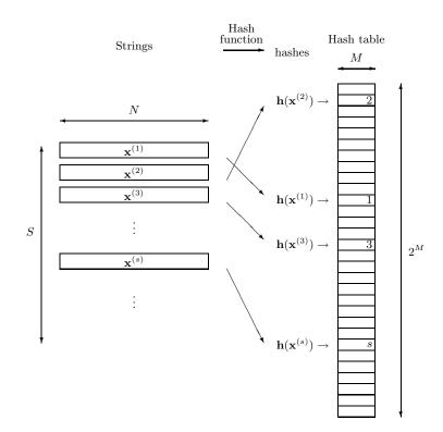
Figure 12.4. Use of hash functions for information retrieval. For each string  $\mathbf{x}^{(s)}$ , the hash  $\mathbf{h} = \mathbf{h}(\mathbf{x}^{(s)})$ is computed, and the value of *s* is written into the **h**th row of the hash table. Blank rows in the hash table contain the value zero. The table size is  $T = 2^M$ .
