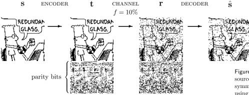
2) between these two triplets are called the *syndrome* of the received vector. If the syndrome is zero – if all three parity checks are happy – then the received vector is a codeword, and the most probable decoding is given by reading out its first four bits. If the syndrome is non-zero, then the noise sequence for this block was non-zero, and the syndrome is our pointer to the most probable error pattern.
