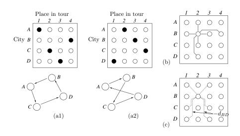
Figure 42.10. Hopfield network for solving a travelling salesman problem with K = 4 cities. (a1,2) Two solution states of the 16-neuron network, with activites represented by black = 1, white = 0; and the tours corresponding to these network states. (b) The negative weights between node B2 and other nodes; these weights enforce validity of a tour. (c) The negative weights that embody the distance objective function.
