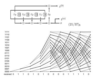
Figure 48.6. The trellis for a k = 4 code painted with the likelihood function when the received vector is equal to a codeword with just one bit flipped. There are three line styles, depending on the value of the likelihood: thick solid lines show the edges in the trellis that match the corresponding two bits of the received string exactly; thick dotted lines show edges that match one bit but mismatch the other; and thin dotted lines show the edges that mismatch both bits.
