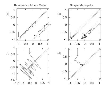
Figure 30.2. (a,b) Hamiltonian Monte Carlo used to generate samples from a bivariate Gaussian with correlation  $\rho = 0.998$ . (c,d) For comparison, a simple random-walk Metropolis method, given equal computer time.
