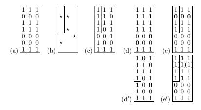
horizontally then with H(7, 4) vertically. The block length of the concatenated code is 27. The number of source bits per codeword is four, shown by the small rectangle.
