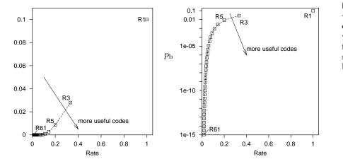
Figure 1.12. Error probability  $p_{\rm b}$  versus rate for repetition codes over a binary symmetric channel with f = 0.1. The right-hand figure shows  $p_{\rm b}$  on a logarithmic scale. We would like the rate to be large and  $p_{\rm b}$  to be small.
