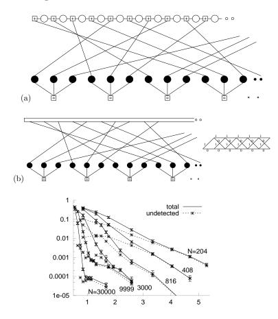
Figure 49.1. Factor graphs for a repeat-accumulate code with rate 1/3. (a) Using elementary nodes. Each white circle represents a transmitted bit. Each  $\pm$  constraint forces the sum of the 3 bits to which it is connected to be even. Each black circle represents an intermediate binary variable. Each  $\equiv$  constraint forces the three variables to which it is connected to be equal.
