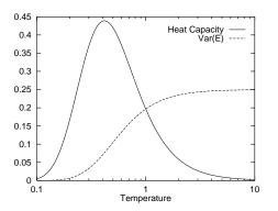
Figure 31.6. Schottky anomaly – Heat capacity and fluctuations in energy as a function of temperature for a two-level system with separation  $\epsilon = 1$  and  $k_{\rm B} = 1$ .
