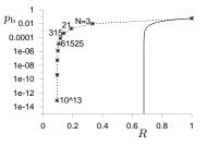
Figure 13.14. The bit error probabilities versus the rates R of the concatenated Hamming codes, for the binary symmetric channel with f = 0.0588. The solid line shows the Shannon limit for this channel.
