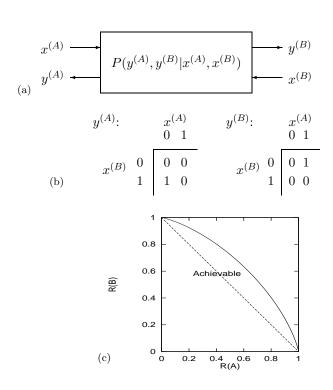
Figure 15.9. (a) A general two-way channel. (b) The rules for a binary two-way channel. The two tables show the outputs  $y^{(A)}$  and  $y^{(B)}$  that result for each state of the inputs. (c) Achievable region for the two-way binary channel. Rates below the solid line are achievable. The dotted line shows the 'obviously achievable' region which can be attained by simple time-sharing.
