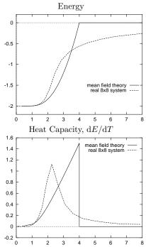
Figure 33.3. Comparison of approximating distribution's properties with those of a real  $8 \times 8$  fragment. Notice that the variational free energy of the approximating distribution is indeed an upper bound on the free energy of the real system. All quantities are shown 'per spin'.
