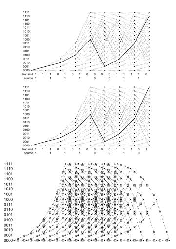
Figure 48.7. Two paths that differ in two transmitted bits only.
