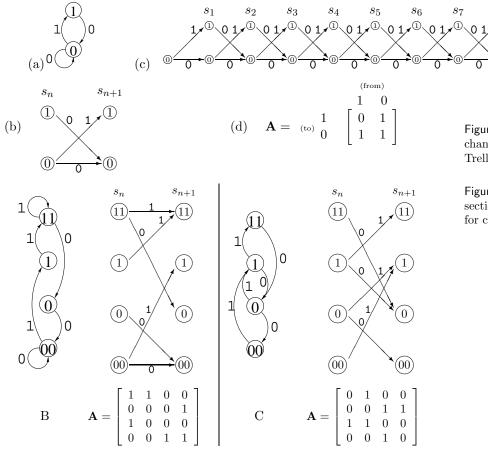
Figure 17.2. (a) State diagram for channel A. (b) Trellis section. (c) Trellis. (d) Connection matrix.
