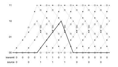
Figure 48.5. The source sequence for the systematic recursive code (00111000) produces the same path through the trellis as (00100000) does in the nonsystematic nonrecursive case.
