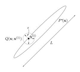
Figure 29.11. Metropolis method in two dimensions, showing a traditional proposal density that has a sufficiently small step size  $\epsilon$ that the acceptance frequency will be about 0.5.
