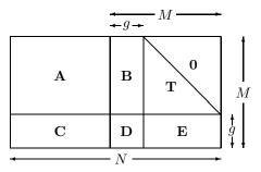
Figure 47.19. The parity-check matrix in approximate lower-triangular form.
