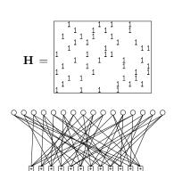
Figure 47.1. A low-density parity-check matrix and the corresponding graph of a rate-1/4low-density parity-check code with blocklength N = 16, and M = 12 constraints. Each white circle represents a transmitted bit. Each bit participates in j = 3constraints, represented by  $\boxdot$ squares. Each constraint forces the sum of the k = 4 bits to which it is connected to be even.
