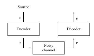
Figure 1.6. The 'system' solution for achieving reliable communication over a noisy channel. The encoding system introduces systematic redundancy into the transmitted vector  $\mathbf{t}$ . The decoding system uses this known redundancy to deduce from the received vector  $\mathbf{r}$  both the original source vector and the noise introduced by the channel.
