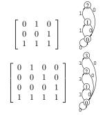
Figure 17.9. State diagrams and connection matrices for channels with maximum runlengths for 1s equal to 2 and 3.
