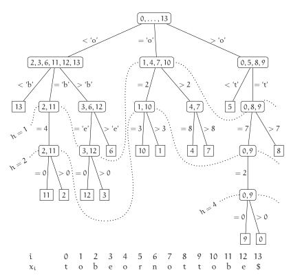
An implicit ternary tree that corresponds to the sorting process illustrated on page 55. Suffixes processed in each partition are listed inside the corresponding nodes. Outgoing edges are labeled with relation operations and pivot keys that determine the results of partitioning. The dotted curves mark transitions between sorting passes.
