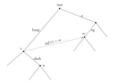
Fragment of a suffix tree for a suffix tree for a string containing 'bangslash'. In this tree, point('bangsl') is (v, 2, 's'), child(root, 'b') is the node v and child(v, 's') is the node u. The dotted line shows the suffix link of v.
