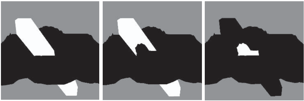
Figure 5: Rendering the front surface and the back surface and taking the difference between two images
