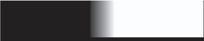
Figure 7: Lookup table (LUT) used for transitioning between two images. The gray area in the center keeps the edges from making hard noticeable transitions.
