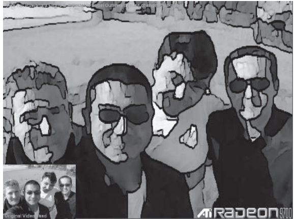
Figure 17: A 7 \times 7 Kuwahara filter plus outlines based on the Sobel edge detection filter has been applied to the image for real-time posterization. The 7 \times 7 filter's advantage over the 5 \times 5 filter is better posterization for about the same number of instructions. (See Color Plate 25.)
