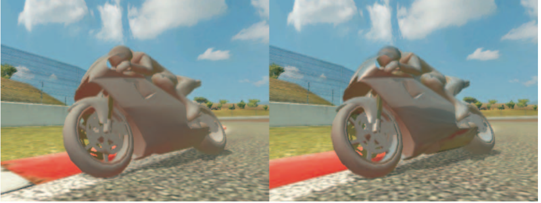
Color Plate 4. (left) Diffuse (dot3) sunlight plus radiosity hemisphere lookup. (right) With the addition of specular and Fresnel contributions, using a static cube map holding an image of typical surroundings. (See page 113.)
