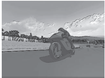
Figure 6: The complete cartoon mode uses a discrete three-level lighting shader on bike and rider.
