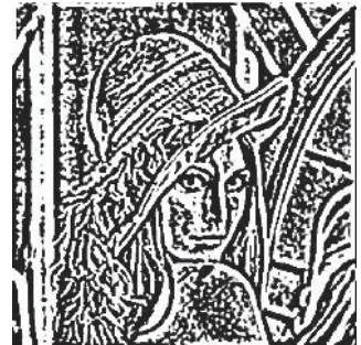
Figure 14: 17×17 Laplacian of Gaussian operation
