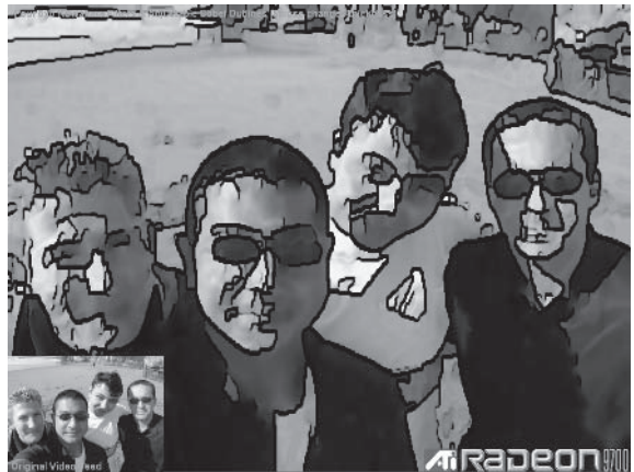
Figure 14: A 5 \times 5 Kuwahara filter plus outlines based on the Sobel edge detection filter has been applied to the image for real-time posterization. (See Color Plate 24.)
