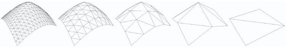
Figure 2: The same patch tessellated in different levels ranging from full geometry (level 0) to a single quad (level 4)
