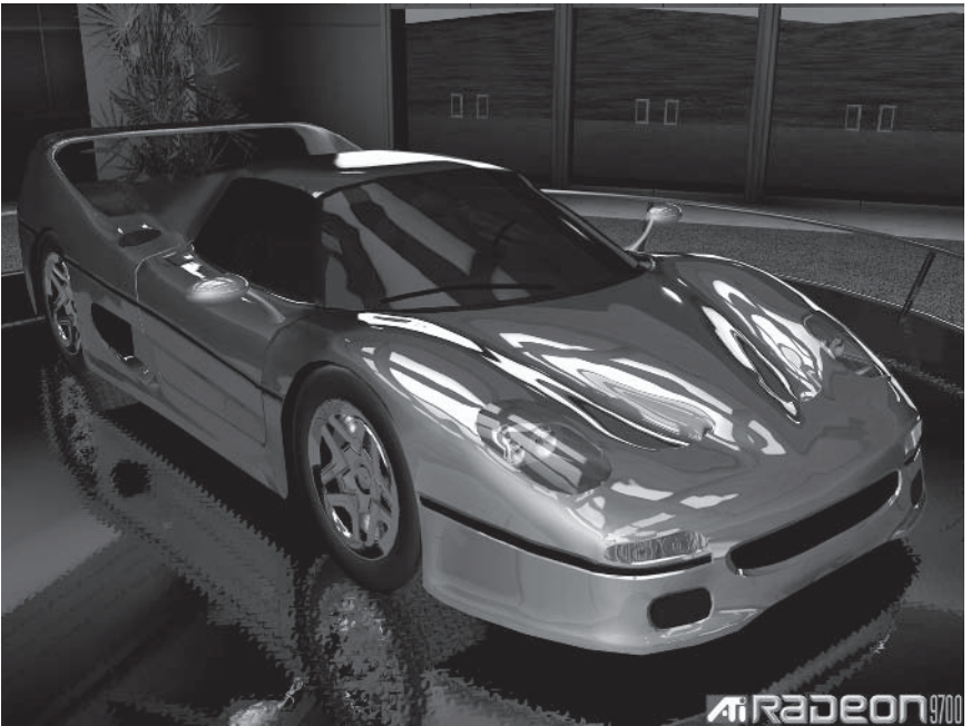
Figure 1: Two-tone, suspended microflake car paint rendered in real time using an HLSL pixel shader in DirectX 9
