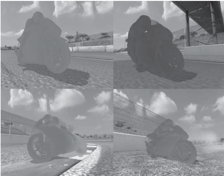
Figure 4: These images show the hemisphere lighting on its own, using a single DXT1 format radiosity map that encodes both shadow and ground color information. (See Color Plate 6.)
