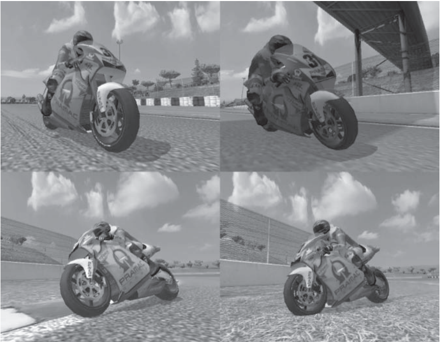
Figure 5: The complete lighting model, combining a base texture, radiosity hemisphere, Fresnel cube map, and dot3 sunlight (See Color Plate 7.)
