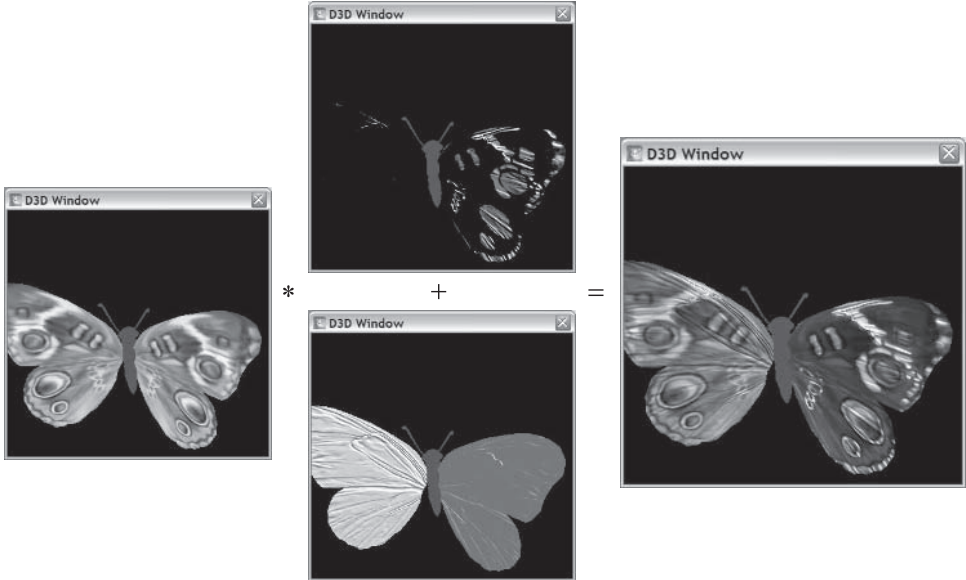
Figure 4: Combining the base texture map with scattered reflected light and diffusely reflected light
