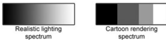
Figure 25.4: Spectra for different renderings.
