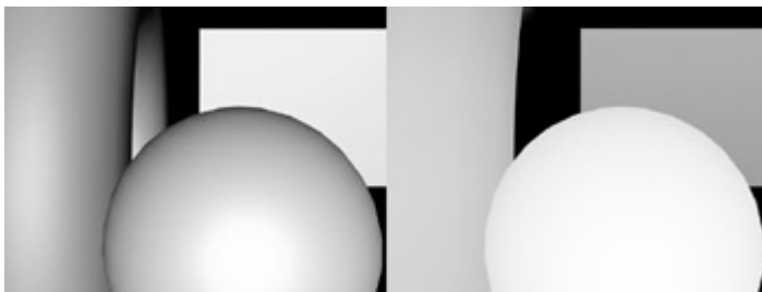
Figure 14.1: A scene and the contents of its depth buffer.
