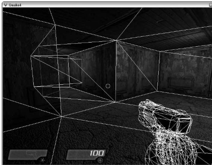
Figure 10-13: The portal brush doing its job. The game no longer has to render the second room.
