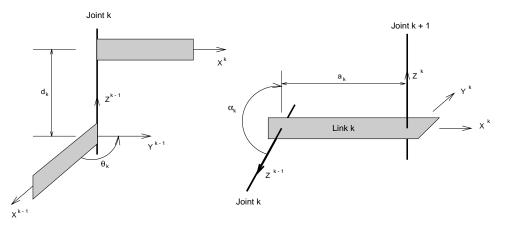
Figure 2.2: Joint and Link Parameters
