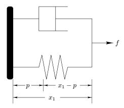
Figure 2.3: "Muscle" represented as a spring and damper
