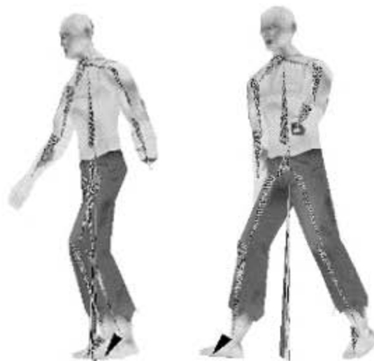
Figure 8.6 Here you can see the bones rendered on top of the model with a deactivated depth buffer. The bone between the legs is very interesting. This can be used to throw the model to the ground in a smooth animation. (Source for the free model: http://www.psionic3d.co.uk )
