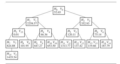
Figure 4.6 The heap array after swapping  $H_7$  and  $H_{15}$  in Figure 4.5.
