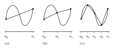
Figure 4.32 (a) A curve segment tessellated by a single line segment connecting its end points. (b) One subdivision step applied to the original tessellation. (c) Two subdivision steps applied to the original tessellation.
