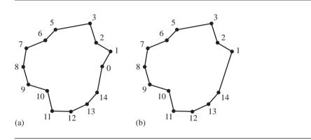
Figure 4.22 (a) The polygon of Figure 4.19(b) and (b) the polygon with  $V_0$  removed.
