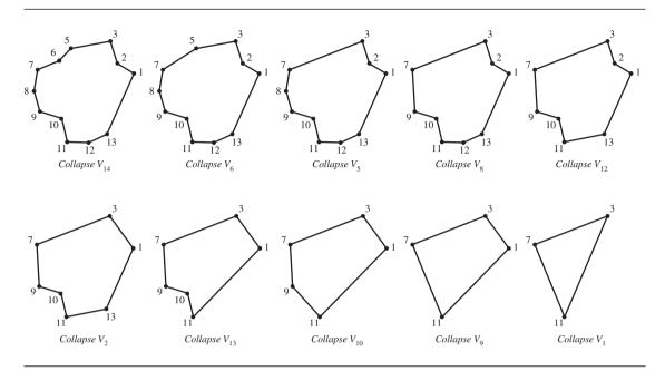
Figure 4.23 The remaining vertex collapses, occurring left to right, then top to bottom.
