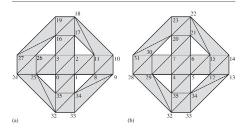
Figure 8.13 The vertex and index assignments for the outside. Two views are presented: (a) the top viewed from the top and (b) the bottom viewed from the top. Additional triangles occur on the walls that connect the top with the bottom.
