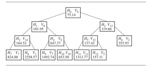
Figure 4.20 The heap after moving  $H_{13}$  to  $H_0$ , then swapping  $H_0$  with  $H_2$  and  $H_2$  with  $H_6$ .
