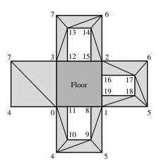
Figure 8.11 The vertex and index assignments for the end rooms. The view is of the room with the ceiling removed and the walls folded outward. The floor is dark gray, the walls are light gray, and the portal cutouts are white.
