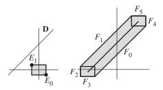
Figure 6.11 An OBB and a segment. The OBB is extruded along the segment in the direction  $\mathbf{D}$ . The faces  $F_0$  and  $F_1$  are generated by OBB edges and  $\mathbf{D}$ . The faces  $F_2$  and  $F_3$  are contributed from the OBB at one end point; the faces  $F_4$  and  $F_5$  are contributed from the OBB at the other end point.
