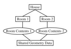
Figure 3.5 The scene graph of Figure 3.4, but with instancing at a low level (geometric data) rather than at a node level.
