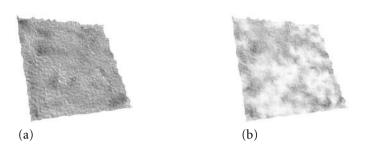
Figure 1.2 Two screen shots from the sample application for drawing a multitextured triangle mesh. The mesh has been rotated the same amount in the two images. (a) The mesh with only the mountain texture (the primary texture). (b) The mesh with the mountain texture as the primary texture and with the fog texture as the secondary texture. (See also Color Plate 1.2.)
