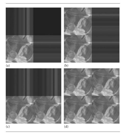
Figure 3.13 A square with vertices (-1, -1), (1, -1), (1, 1), and (-1, 1) is drawn with a texture image. The texture coordinates at the square's corners are (0, 0), (2, 0), (2, 2), and (0, 2). (a) Clamp u and clamp v. (b) Clamp u and repeat v. (c) Repeat u and clamp v. (d) Repeat u and repeat v. (See also Color Plate 3.13.)
