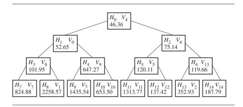
Figure 4.14 The heap after swapping  $H_0$  with  $H_1$ ,  $H_1$  with  $H_4$ , and  $H_4$  with  $H_9$ .
