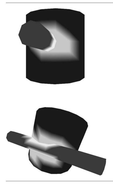
Figure 6.16 A couple of screen shots showing the triangles of intersection between two cylinders. (See also Color Plate 6.16.)
