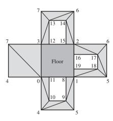
Figure 8.12 The vertex and index assignments for the connector rooms. The view is of the room with the ceiling removed and the walls folded outward. The floor is dark gray, the walls are light gray, and the portal cutouts are white.
