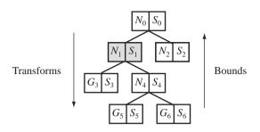
Figure 3.8 A geometric update of a simple scene graph. The light gray shaded node,  $N_1$ , is the one at which the UpdateGS call initiates.
