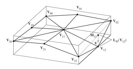
Figure 4.37 A single block with nine vertices labeled and all eight triangles drawn. The candidate vertex for disabling is  $\mathbf{V}_{12}$ , and the candidate vertical line segment for screen space height measurement is  $\langle \mathbf{M}_{12}, \mathbf{V}_{12} \rangle$ .
