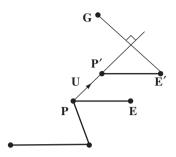
Figure 4.44 A four-node chain whose last node is the end effector **E**. The joint position **P** is to be translated in the unit-length direction **U** to minimize the distance from **E** to the goal's target **G**. The point **E**' attains the minimum distance to the goal.
