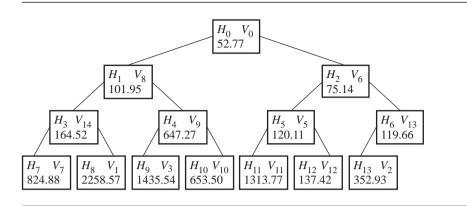
Figure 4.17 The heap after moving  $H_{14}$  to  $H_0$  and then swapping  $H_0$  with  $H_1$  and  $H_1$  with  $H_3$ .
