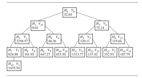
Figure 4.9 The heap array after swapping  $H_1$  and  $H_3$  in Figure 4.8.
