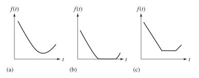
Figure 6.2 The graphs of f(t) for three different point velocities. (a) The velocity is not parallel to any box axis, and the moving point does not intersect the box. (b) The velocity is not parallel to any box axis, and the moving point does intersect the box. (c) The velocity is parallel to a box axis, and the moving point does not intersect the box.
