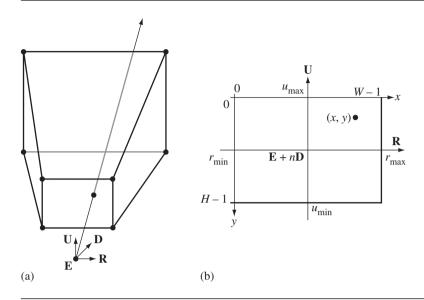
Figure 6.13 (a) A view frustum with a point selected on the near plane. The pick ray has an origin that is the eye point  $\mathbf{E}$ , in world coordinates, and a direction that is from the eye point to the selected point. (b) The viewport on the near plane with screen coordinates (x, y) listed for the selected point.
