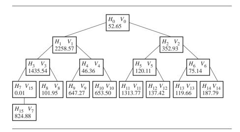
Figure 4.4 The heap array after swapping  $H_7$  and  $H_{15}$  in Figure 4.3.
