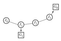
Figure 4.43 An IK system for a linear chain of four nodes.
