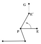
Figure 4.45 A four-node chain whose last node is the end effector **E**. The joint position **P** is to be rotated about an axis with unit-length direction **U** to minimize the distance from **E** to the goal's target **G**. For the sake of illustration, suppose that axis is out of the plane of the page. The point **E**' attains the minimum distance to the goal.
