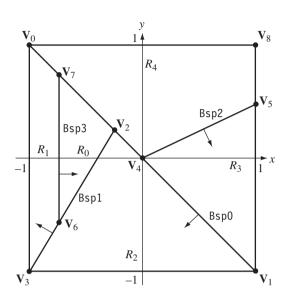
Figure 8.3 The partitioning of the world by four BSP planes. Only the square region defined by  $|x| \le 1$  and  $|y| \le 1$  is shown.
