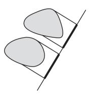
Figure 6.6 Two planar, convex objects that are not intersecting. A line is shown with the intervals of projection of the objects. The intervals are disjoint.
