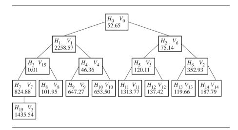
Figure 4.7 The heap array after swapping  $H_2$  and  $H_6$  in Figure 4.6.
