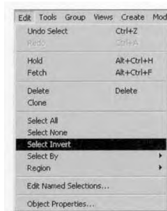
FIGURE 4.31 Select Invert is the fastest way to select and hide a large group of vertices.
