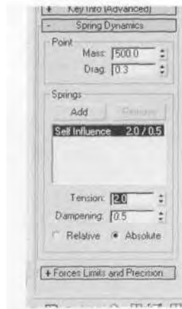
FIGURE 2.53 Self Influence must be highlighted before Tension and Dampening can be adjusted.
