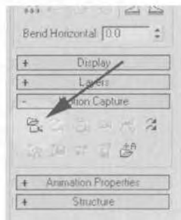
FIGURE 8.1 Click the Load Motion Capture File button to import CSM or BVH files.
