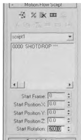
FIGURE 8.53 Entering 200 in the Start Rotation field rotates the character 200 degrees along the Z-axis.
