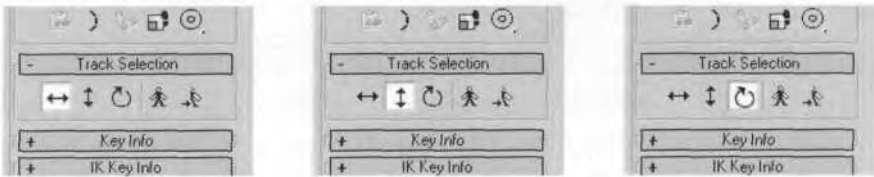
FIGURE 6.7 Choose between Body Horizontal, Body Vertical, and Body Rotate animation tracks for the COM.
