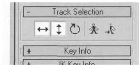
FIGURE 8.78 Using the Restrict to ZX or Restrict to YZ buttons, you can set keys for both Body Horizontal and Body Vertical animation tracks for the COM.
