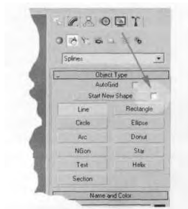
FIGURE 1.11 Uncheck the Start New Shape box to avoid the step of attaching the lines together later.
