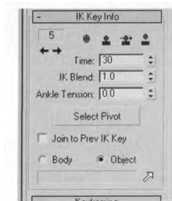
FIGURE 8.73 Lock down each foot at Frame 30, unchecking the Join to Prev IK Key box.
