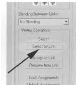
FIGURE 3.43 The Select by Link button selects all vertices assigned to a link.
