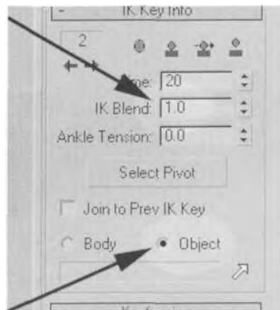
FIGURE 7.9 Keyframes for limbs are automatically converted to a planted key just by clicking on the Anchor button.
