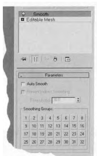
FIGURE 1.23 Applying a Smooth modifier to a mesh results in stripping its smoothing groups (at first).
