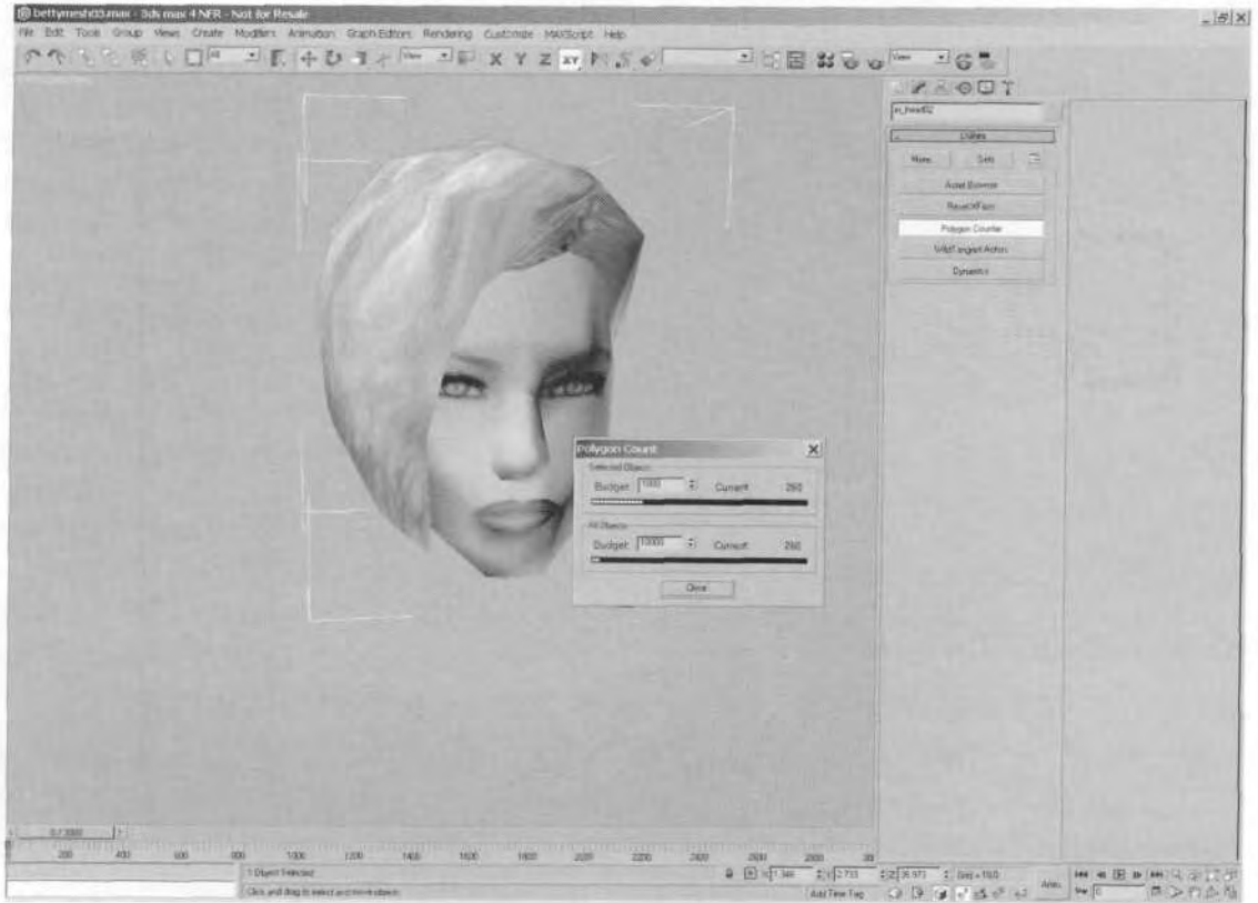
FIGURE 1.32 The Polygon Counter tool can help you stay within your face count budget.
