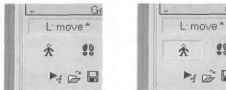
FIGURE 2.7 In order to fit your Biped to a mesh, it needs to be in FIGURE mode.
