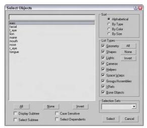
**Figure 6-3:** The Select Objects dialog box displays all objects in the current scene by name.
