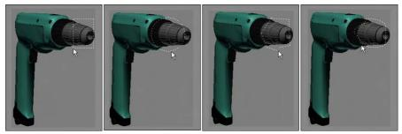
**Figure 6-4:** The drill's front is selected using the Rectangular, Circular, Fence, and Lasso selection methods.
