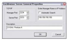
**Figure 45-8:** Manually choosing the manager's IP address
