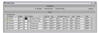
**Figure 27-4:** The Light Lister dialog box includes a comprehensive list of light settings in one place.
