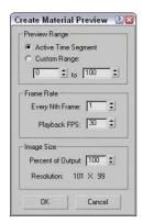
**Figure 30-12:** The Create Material Preview dialog box can render the entire range of frames or a select number of frames.
