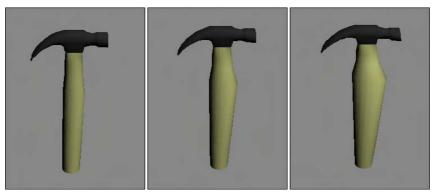
Figure 11-27: The Spherify modifier pushes all vertices outward like a sphere.
