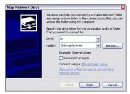
**Figure 45-5:** Mapping the Z drive to point to \\dungar\scenes\.
