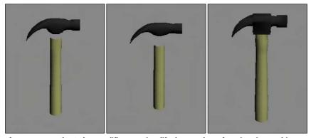
Figure 11-20: The Relax modifier can simplify the number of vertices in an object.
