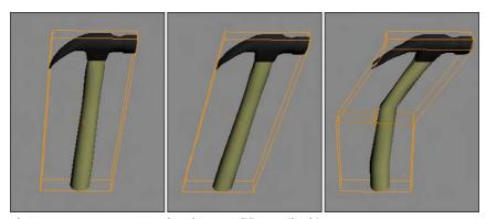
Figure 11-24: You can use the Skew modifier to tilt objects.
