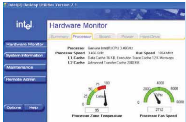
▲ Under heavy loads, Presler runs hot. Really hot. Surface of the sun hot. Here, we see it running at 95 degrees Celsius.
