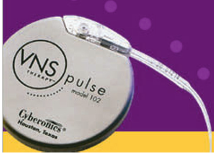
Fig. 1.2. Implantable device for Epilepsy seizures treatment [7]. Cyberonics, Inc. http://www.cyberonics.com/
