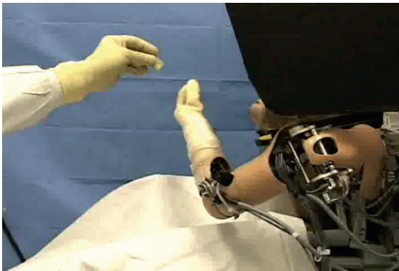
Fig. 1.1. Robotic arm controlled by monkey motor cortex signals. MotorLab, University of Pittsburgh. Prof Andy Schwartz, U. Pitt
