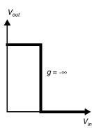
Figure 1.17 Ideal voltage-transfer characteristic.
