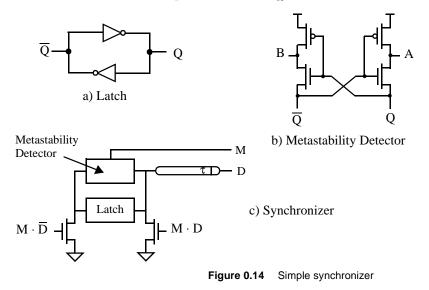
b. The circuit in part b has been proposed to detect metastability. How does it work? How would you generate a signal M that is high when the latch is metastable?
