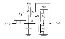
Figure 6.40 Transistor-sizing problem for level-restoring circuit.
