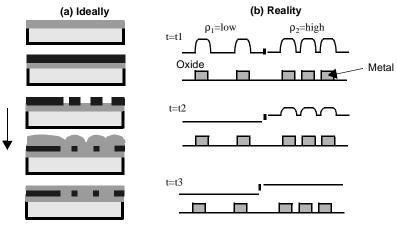
Figure 10.15 Inter-level Dielectric (ILD) thickness variation due to density (coutersy of Duane Boning).
