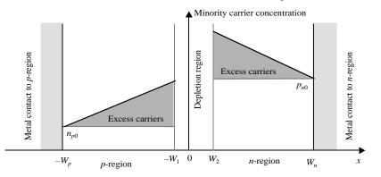
Figure 3.3 Minority carrier concentrations in the neutral region near an abrupt *pn*-junction under forward-bias conditions.
