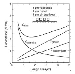
**Figure 4.7** Interconnect capacitance as a function of design rules. It consists of a capacitance to ground and an inter-wire capacitance (from [Schaper83]).
