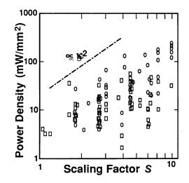
**Figure 5.40** Evolution of power-density in micro- and DSP processors, as a function of the scaling factor S ([Sakurai97]). *S* is normalized to 1 for a 4  $\mu$ m process.
