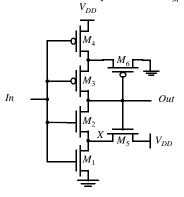
Figure 7.50 Alternate CMOS Schmitt trigger.
