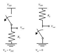
**Figure 5.2** Switch models of CMOS inverter.
