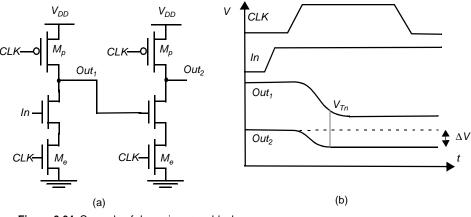
Figure 6.64 Cascade of dynamic *n*-type blocks.
