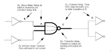
Figure E.1 Delay components.
