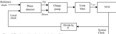
Figure 10.58 Composition of a phase-locked loop (PLL).
