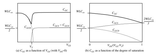
Figure 3.30 Distribution of the gate-channel capacitance as a function of  $V_{GS}$  and  $V_{DS}$  (from [Dally98]).
