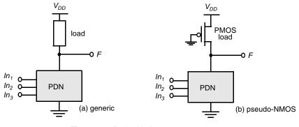
Figure 6.27 Ratioed logic gate.
