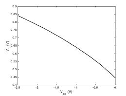
The effect of the well bias on the threshold voltage of an NMOS transistor is plotted in for typical values of  $|-2\phi_F| = 0.6$  V and  $\gamma = 0.4$  V<sup>0.5</sup>. A negative bias on the well or substrate causes the threshold to increase from 0.45 V to 0.85 V. Note also that  $V_{SB}$  always has to be larger than -0.6 V in an NMOS. If not, the sourcebody diode becomes forward biased, which deteriorates the transistor operation.
