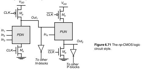
*np*-CMOS logic exploits the duality between *n*-tree and *p*-tree logic gates to eliminate the cascading problem. If the *n*-tree gates are controlled by *CLK*, and *p*-tree gates are controlled using  $\overline{CLK}$ , *n*-tree gates can directly drive *p*-tree gates, and vice-versa. Similar to Domino, *n*-tree outputs must go through an inverter when connecting to another *n*-tree gate. During the precharge phase (*CLK* = 0), the output of the *n*-tree gate, *Out1*, is charged
