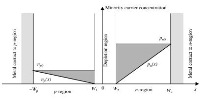
Figure 3.4 Minority carrier concentration in the neutral regions near the *pn*-junction under reverse-bias conditions.
