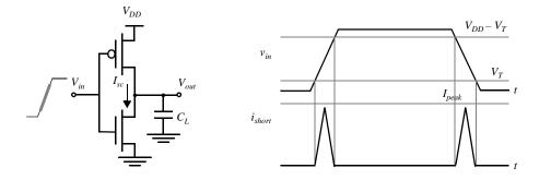
Figure 5.30 Short-circuit currents during transients.
