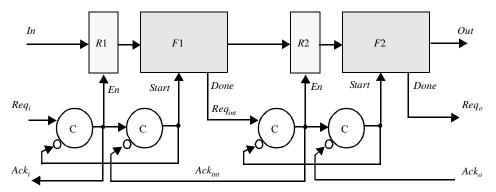
Figure 10.44 Self-timed pipelined datapath—complete composition.
