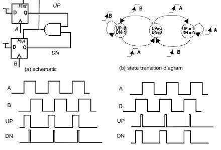
multiple of the frequency. The PFD takes two clock inputs and produces two outputs, UP and DOWN as shown in Figure 10.60.
