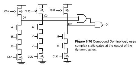
gate coupling. Care must be taken to ensure that the dynamic nodes are not affected by the coupling between the output of the static gates and the output of dynamic nodes.
