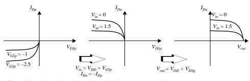
Figure 5.3 Transforming PMOS *I-V* characteristic to a common coordinate set (assuming VDD = 2.5 V).
