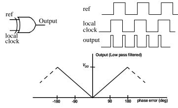
the XOR is low pass filtered and acts as a control voltage to the VCO. The output (low pass filtered) as a function of the phase error is also shown.
