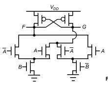
Figure 6.6 Two-input complex logic gate.
