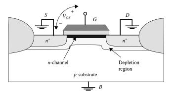
Figure 3.13 NMOS transistor for positive V<sub>GS</sub>, showing depletion region and induced channel.
