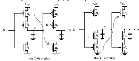
Figure 7.27 C<sup>2</sup>MOS *D*-FF during overlap periods. No feasible signal path can exist between In and D, as illustrated by the arrows.
