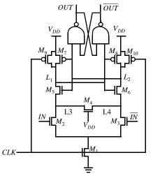
**Figure 7.38** *Positive edge-triggered* register based on sense-amplifier.
