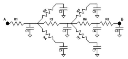
Figure 0.4 RC tree for calculating the delay
