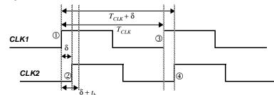
**Figure 10.6** Timing diagram to study the impact of clock skew on performance and funcationality. In this sample timing diagram,  $\delta > 0$ .
