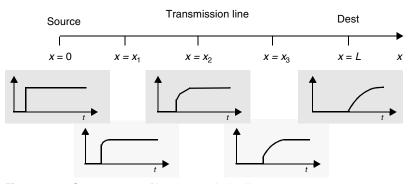
Figure 4.25 Step response of lossy transmission line.
