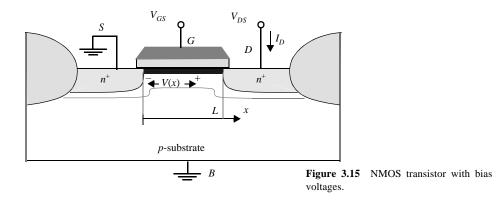
At a point x along the channel, the voltage is V(x), and the gate-to-channel voltage at that point equals  $V_{GS} - V(x)$ . Under the assumption that this voltage exceeds the threshold voltage all along the channel, the induced channel charge per unit area at point x can be computed.
