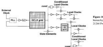
**Figure 10.24** Clock hierarchy for the Alpha 21264 Processor.
