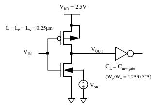
Figure 5.8 CMOS inverter with capacitive
