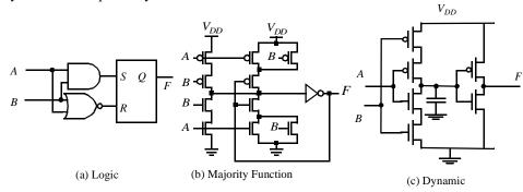
Figure 10.39 Implementations of a Muller C-element.
