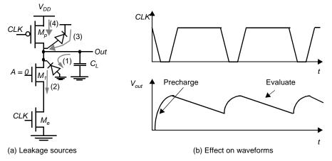
Figure 6.56 Leakage issues in dynamic circuits.
