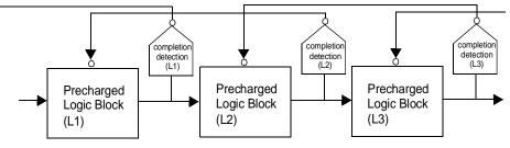
Figure 10.47 Self-resetting logic.
