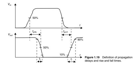
$<sup>^{2}</sup>$  The 50% definition is inspired the assumption that the switching threshold  $V_{M}$  is typically located in the middle of the logic swing.
