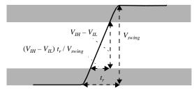
Figure 10.53 Linear approximation of signal slope.
