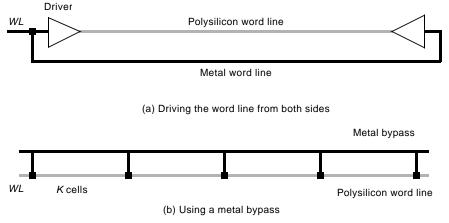
Figure 9.17 Approaches to reduce the word-line delay.
