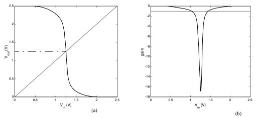
Figure 5.10 Simulated Voltage Transfer Characteristic (a) and voltage gain (b) of CMOS inverter (0.25  $\mu$ m CMOS,  $V_{DD}$  = 2.5 V).
