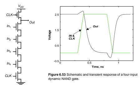
input transitions—to 0.45V, 0.5V and 0.55V, respectively. Above, we have defined the switching threshold of the dynamic gate as the device threshold. However, notice that the amount by which the output voltage drops is a strong function of the input voltage and the available evaluation time. The noise voltage needed to corrupt the signal has to be larger if the evaluation time is short. In other words, the switching threshold is really a function of the evaluation time.
