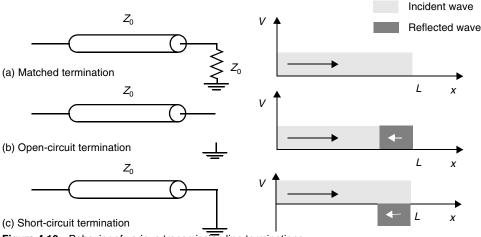
Figure 4.19 Behavior of various transmission line terminations.
