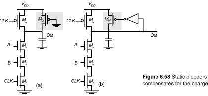
compensates for the charge-leakage.
