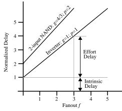
**Figure 6.18** Delay as a function of fanout for an inverter and a 2-input NAND.
