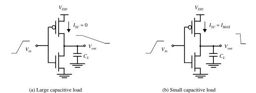
Figure 5.31 Impact of load capacitance on short-circuit current.
