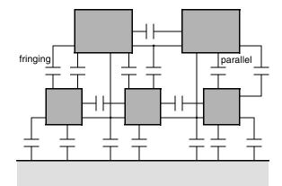
**Figure 4.6** Capacitive coupling between wires in interconnect hierarchy.
