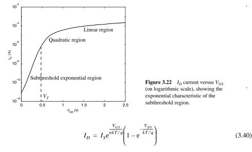
where  $I_s$  and *n* are empirical parameters, with  $n \ge 1$  and typically ranging around 1.5.
