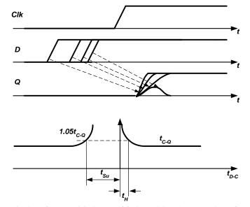
Figure E.3 Characterization of sequential elemnts: (a) determining the setup time of a register; (b) definition of setup and hold times.
