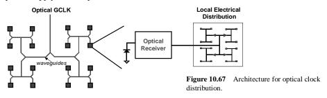
Optical clocking may an important future in high-performance systems. However, the challenges of dealing with process variations in the opto-electronic circuitry must be addressed for this to become a reality.
