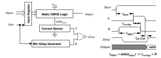
Figure 10.36 Completion-signal generation using current sensing.
