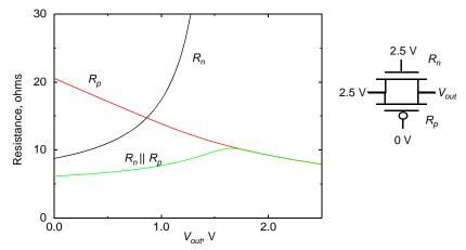
**Figure 6.48** Simulated equivalent resistance of transmission gate for low-to-high transition (for  $(W/L)_n = (W/L)_p = 0.5\mu m/0.25\mu m$ ). A similar response for overall resistance is obtained for the high-to-low transition
