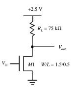
Figure 5.3 Resistive-load inverter
