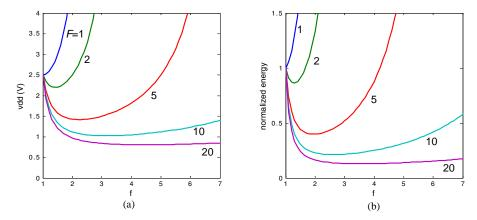
**Figure 5.29** Sizing of an inverter for energy-minimization. (a) Required supply voltage as a function of the sizing factor *f* for different values of the overall effective fanout *F*; (b) Energy of scaled circuit (normalized with respect to the reference case) as a function of *f*.  $V_{ref} = 2.5$ V,  $V_{TE} = 0.5$ V.
