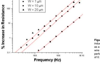
Figure 4.10 Skin-effect induced increase in resistance as a function of frequency and wire width. All simulations were performed for a wire thickness of 0.7  $\mu$ m [Sylvester97].
