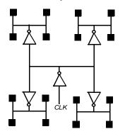
**Figure 10.18** Example of an *H*-tree clock-distribution network for 16 leaf nodes.
