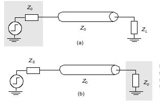
**Figure 9.26** Matched termination scenarios for wires behaving as transmission lines: (a) series termination at the source; (b) parallel termination at the destimation.
