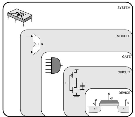
Figure 1.6 Design abstraction levels in digital circuits.
