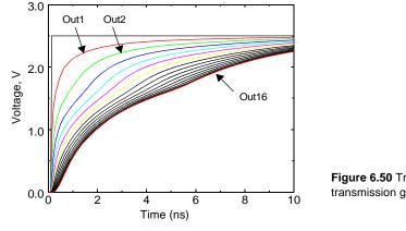
Figure 6.50 Transient response of 16 transmission gates cascaded in series.
