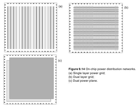
cases, power and ground are brought onto the chip via bonding pads located on the four sides of the chip. Which approach to use depends upon the number of coarse metal layers (this is, thick, high pitch topmost metal layers) one wants to allocate to power distribution.
