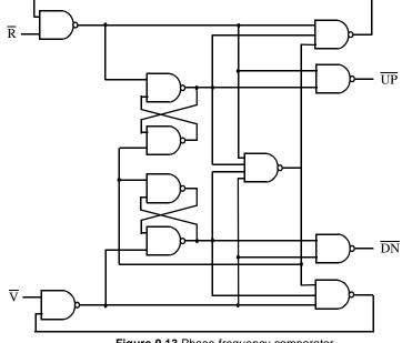
12. Explain how the phase-frequency comparator shown in Figure 0.13 works.
