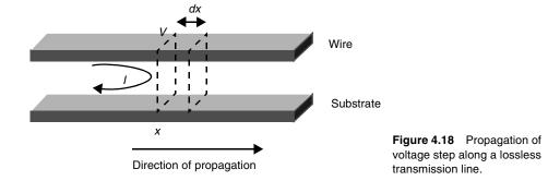
cuitry. Typical values of the characteristic impedance of wires in semiconductor circuits range from 10 to 200  $\Omega$ .
