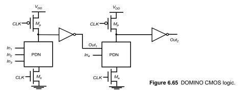
• Very high speeds can be achieved: only a rising edge delay exists, while  $t_{pHL}$  equals zero. The inverter can be sized to match the *fan-out*, which is already much smaller than in the complimentary static CMOS case, as only a single gate capacitance has to be accounted for per fan-out gate.
