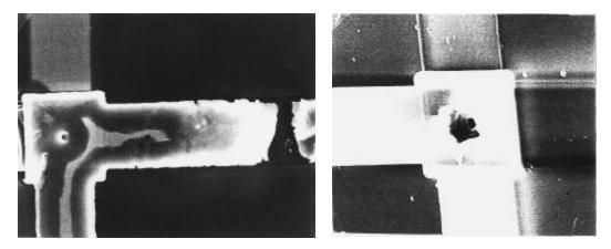
(a) Line-open failure.
