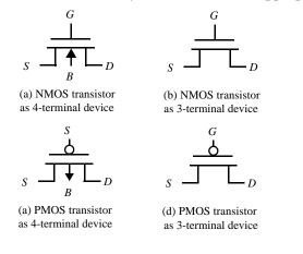
**Figure 3.12** Circuit symbols for MOS transistors.
