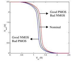
**Figure 5.11** Impact of device variations on static CMOS inverter VTC. The "good" device has a smaller oxide thickness (- 3nm), a smaller length (-25 nm), a higher width (+30 nm), and a smaller threshold (-60 mV). The opposite is true for the "bad" transistor.
