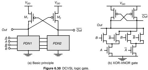
The resulting circuit exhibits a rail-to-rail swing, and the static power dissipation is eliminated: in steady state, none of the stacked pull-down networks and load devices are simultaneously conducting. However, the circuit is still ratioed since the sizing of the PMOS devices relative to the pull-down devices is critical to functionality, not just perfor-
