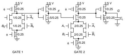
Figure 6.16 DOMINO logic circuit.
