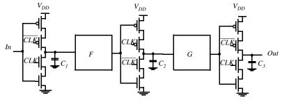
Figure 7.42 Pipelined datapath using C<sup>2</sup>MOS latches.
