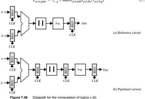
(7.7) $T_{min,pipe} = t_{c-q} + \max(t_{pd,add}, t_{pd,abs}, t_{pd,log})$
