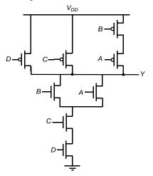
Figure 6.1 CMOS combinational logic gate.
