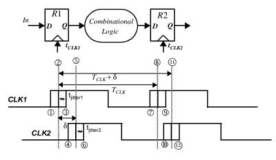
Figure 10.12 Sequential circuit to study the impact of skew and jitter on *edge-triggered* systems. In this example, a positive *skew* ( $\delta$ ) is assumed.
