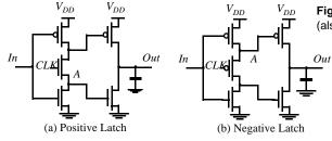
Figure 7.32Simplified TSPC latch(also called split-output).
