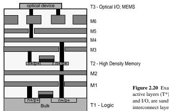
**Figure 2.20** Example of true 3D integration. Extra active layers (T\*), implementing high density memory and I/O, are sandwiched between the metal interconnect layers (M\*).
