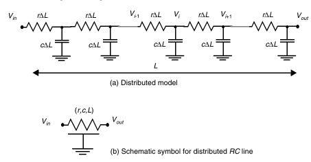
Figure 4.14 Distributed RC line wire-model and its schematic symbol.
