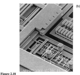
The damascene process (from Geppert98]): process steps (a), and microphotograph of interconnect after removal of insulator (b)
