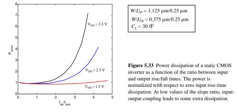
At a supply voltage of 2.5 V and thresholds around 0.5 V, an input/output slope ratio of 2 is needed to cause a 10% degradation in dissipation.
