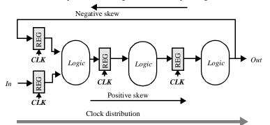
Figure 10.9 Datapath structure with feedback.
