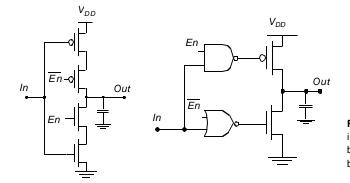
**Figure 9.11** Two possible implementations of a tri-state buffer. En = 1 enables the buffer.
