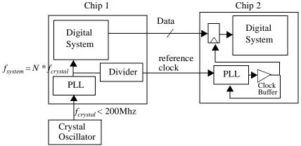
Figure 10.56 Applications of Phase Locked Loops (PLL).
