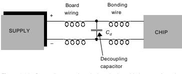
**Figure 9.24** Decoupling capacitors isolate the board inductance from the bonding wire and pin inductance.
