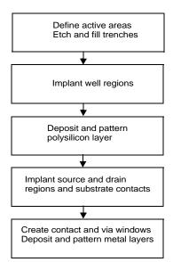
Figure 2.6 Simplified process sequence for the manufacturing of a ndual-well CMOS circuit.
