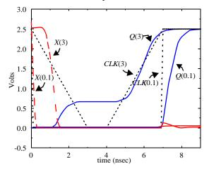
**Figure 7.28** Transient response of  $C^2MOS$  FF for 0.1 nsec and 3 nsec clock rise (fall) times assuming *In* = 1.
