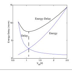
**Figure 5.36** Normalized delay, energy, and energy-delay plots for CMOS inverter in 0.25 µm CMOS technology.
