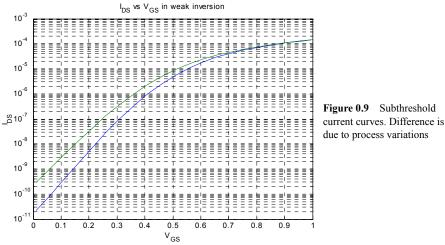
Also assume that the transistors are within the same circuit configurations as Figure 0.10 in If the in put voltages are both  $V_{in} = 0.2V$ . What would be the respective durations to discharge the load of  $C_L = 1pF$  attached to the drains of these devices.
