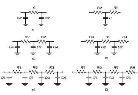
Figure 4.26 Simulation models for distributed RC line.
