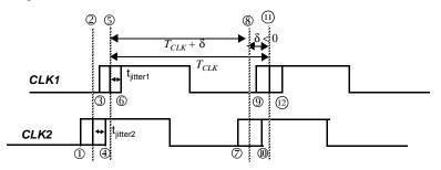
Figure 10.13 Consider a negative clock *skew* ( $\delta$ ) and the *skew* is assumed to be larger than the *jitter*.
