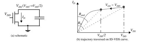
Figure 3.26 Discharging a capacitor through an NMOS transistor: Schematic (a) and *I*-V trajectory (b). The instantaneous resistance of the transistor equals  $(V_{DS}/I_D)$  and is visualized by the angle with respect to the y-axis.
