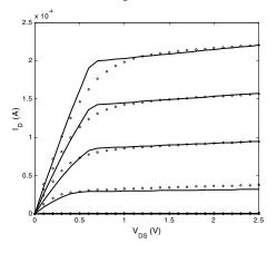
**Figure 3.24** Correspondence between simple model (solid line) and SPICE simulation (dotted) for minimumsize NMOS transistor ( $W_d$ =0.375 µm,  $L_d$ =0.25 µm). Observe the discrepancy in the transition zone between resistive and velocity saturation.
