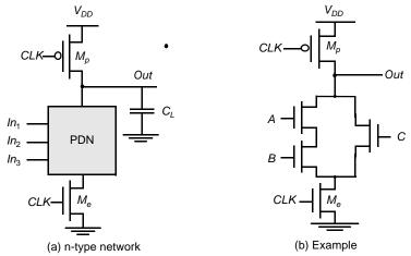
tion of this circuit is divided into two major phases: *precharge* and *evaluation*, with the mode of operation determined by the *clock signal CLK*.
