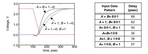
Figure 6.9 Example showing the delay dependence on input patterns.
