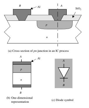
Figure 3.1 Abrupt *pn*-junction diode and its schematic symbol.
