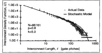
**Figure 4.27** Distribution of wire lengths in an advanced microprocessor as a function of the gate pitch.
