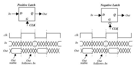
Figure 7.3 Timing of positive and negative latches.
