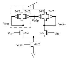
and R comes from the variable resistor that is the load for the delay cell. Below is a circuit schematic of a typical delay cell.
