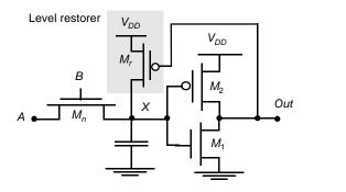
Figure 6.39 Level-restoring circuit.
