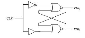
**Figure 7.22** Circuitry for generating a two-phase non-overlapping clock.
