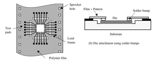
(a) Polymer tape with imprinted wiring pattern
