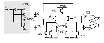
Figure 9.33 Differential reducedswing interconnect system using an dditional supply rail at the driver. The receiver is a clocked differential flip-flop [Burd00].
