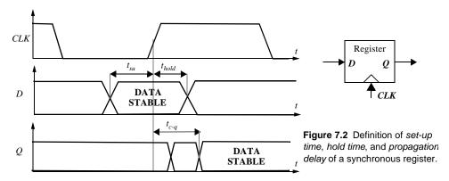
ing that the *set-up* and *hold*-times are met, the data at the D input is copied to the Q output after a worst-case propagation delay (with reference to the clock edge) denoted by  $t_{c-q}$ .
