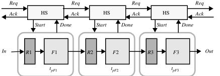
Figure 10.32 Self-timed, pipelined datapath.
