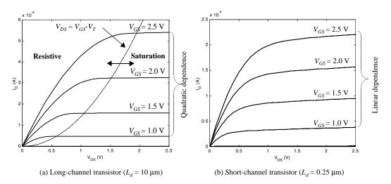
Figure 3.19 I-V characteristics of long- and a short-channel NMOS transistors in a 0.25  $\mu$ m CMOS technology. The (*W/L*) ration of both transistors is identical and equals 1.5
