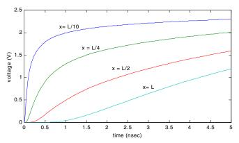
Figure 4.15 Simulated step response of resistive-capacitive wire as a function of time and place.
