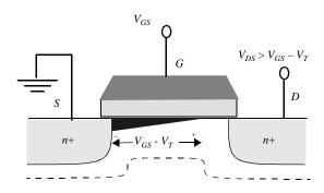
Figure 3.16 NMOS transistor under pinch-off conditions.
