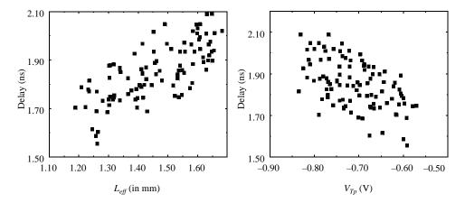
**Figure 3.38** Distribution plots of speed of adder circuit as a function of varying device parameters, as obtained by a Monte Carlo analysis. The circuit is implemented in a 2  $\mu$ m (nominal) CMOS technology (*courtesy of Eric Boskin, UCB, and ATMEL corp.*).
