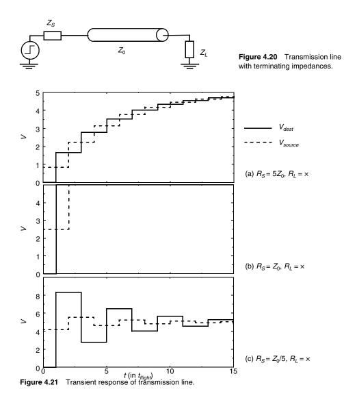
Only a small fraction of the incoming signal  $V_{in}$  is injected into the transmission line. The amount injected is determined by the resistive divider formed by the source resistance and the characteristic impedance  $Z_0$ .
