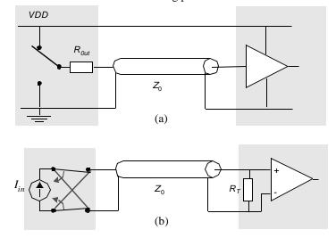
Figure 9.36 Voltage- versus current-mode transmission systems. The latter has the advantage of higher noise immunity with respect to supply noise.
