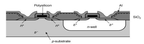
Figure 2.1 Cross section of an n-well CMOS process.
