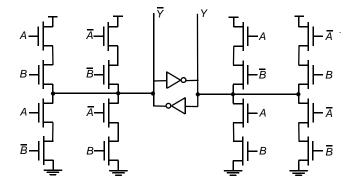
Figure 6.9 Cascoded Logic Styles.
