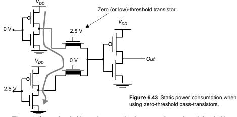
The use of zero-threshold transistors can be dangerous due to the subthreshold currents that can flow through the pass-transistors, even if  $V_{GS}$  is slightly below  $V_T$ . This is demonstrated in Figure 6.43, which points out a potential sneak dc-current path. While these leakage paths are not critical when the device is switching constantly, they do pose a significant energy-overhead when the circuit is in the idle state.
