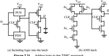
Figure 7.31 Adding logic to the TSPC approach.
