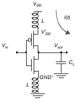
Figure 9.21 Inductive coupling between external and internal supply voltages.
