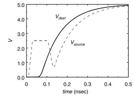
Figure 4.24 Capacitively terminated transmission line:  $R_S =$ 50  $\Omega$ ,  $R_L = \infty$ ,  $C_L = 2$  pF,  $Z_0 = 50 \Omega$ ,  $t_{flight} = 50$  psec.
