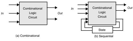
Figure 6.1 High level classification of logic circuits.
