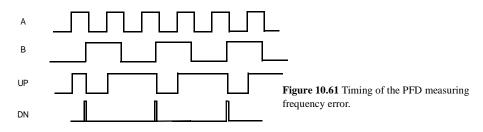
The circuit also acts as a frequency detector, providing a measure of the frequency error (Figure 10.61). For the case when A is at a higher frequency than B, the PFD generates a lot more UP pulses (with the average proportional to the frequency difference),
