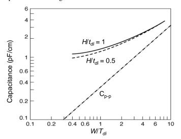
**Figure 4.5** Capacitance of interconnect wire as a function of  $(W/t_{di})$ , including fringing-field effects (from [Schaper83]). Two values of  $H/t_{di}$  are considered. Silicon-dioxide with  $\varepsilon_r = 3.9$  is used as dielectric.
