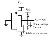
**Figure 5.34** Sources of leakage currents in CMOS inverter (for  $V_{in} = 0$  V).
