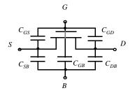
Figure 3.33 MOSFET capacitance model.
