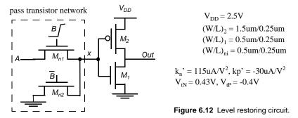
Consider the circuit of Figure 6.12. Assume the inverter switches ideally at  $V_{DD}/2$ , neglect body effect, channel length modulation and all parasitic capacitance throughout this problem.
