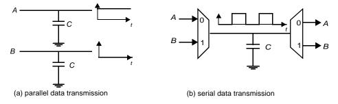
Figure 6.25 Parallel versus time-multiplexed data busses.
