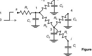
approximative model of a resistive-capacitive wire. The Elmore delay of this chain network can be derived with the aid of Eq. (4.13):
