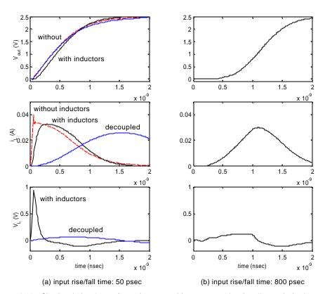
**Figure 9.22** Simulated signal waveforms for output driver connected to bonding pads for input rise/fall times of 50 psec (a) and 800 psec (b), respectively. The waveforms in (a) show the results when (1) no inductors are present in the power distribution network (ideal case); (b) in the presence of inductors; and (c) with added decoupling capcitance of 200 pF.
