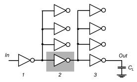
**Figure 5.22** Inverter network, in which each gate has a fanout of 4 gates, distributing a single input to 16 output signals in a tree-like fashion.
