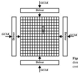
**Figure 10.20** Grid structures allow a low skew distribution and physical design flexibility at the cost of power dissipation [Bailey00].
