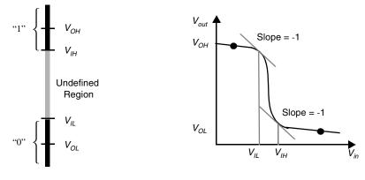
(a) Relationship between voltage and logic levels Figure 1.12 Mapping logic levels to the voltage domain. (b) Definition of  $V_{IH}$  and  $V_{IL}$
