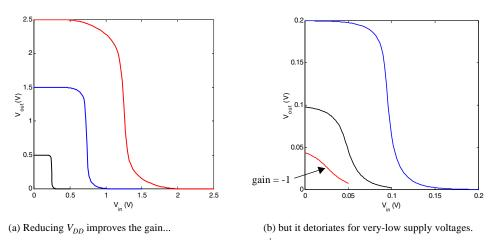
Figure 5.12 VTC of CMOS inverter as a function of supply voltage (0.25 µm CMOS technology).
