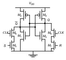
Figure 7.8 CMOS clocked SR flip-flop.
