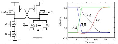
**Figure 6.31**Transient response of a simple AND/NAND DCVSL gate.  $M_1$  and  $M_2$  1 $\mu$ m/0.25 $\mu$ m,  $M_3$  and  $M_4$  are 0.5 $\mu$ m/0.25 $\mu$ m and the cross-coupled PMOS devices are 1.5 $\mu$ m/0.25 $\mu$ m.
