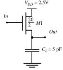
Figure 5.6 Circuit diagram with annotated W/L ratios
