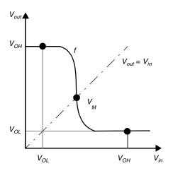
Figure 1.11 Inverter voltage-transfer characteristic.
