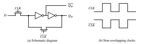
Figure 7.13 Multiplexer-based NMOS latch using NMOS-only pass transistors.
