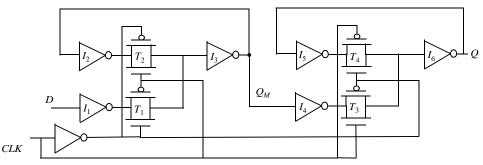
Figure 7.15 Master-slave positive edge-triggered register using multiplexers.
