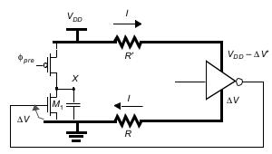
**Figure 9.13** Ohmic voltage drop on the supply rails reduces the noise margins.
