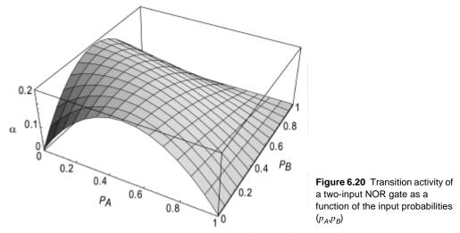
Figure 6.20 shows the transition probability as a function of  $p_a$  and  $p_b$ . Observe how this graph degrades into the simple inverter case when one of the input probabilities is set to 0. From this plot, it is clear that understanding the signal statistics and their impact on switching events can be used to significantly impact the power dissipation.
