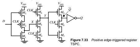
**WARNING:** Similar to the  $C^2MOS$  latch, the TSPC latch malfunctions when the *slope of the clock* is not sufficiently steep. Slow clocks cause both the NMOS and PMOS clocked transistors to be on simultaneously, resulting in undefined values of the states and race conditions. The clock slopes should therefore be carefully controlled. If necessary, local buffers must be introduced to ensure the quality of the clock signals.
