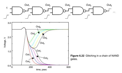
logic block to the next can cause spurious transitions, called *glitches, critical races, or dynamic hazards*, to occur: a node can exhibit multiple transitions in a single clock cycle before settling to the correct logic level.
