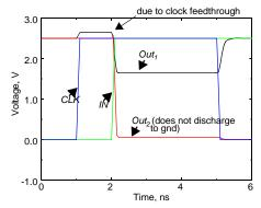
Figure 6.63 Clock feedthrough effect.
