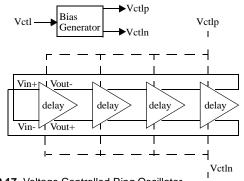
Figure 0.17 Voltage Controlled Ring Oscillator
