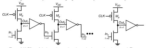
**Figure 6.66** Effect of ripple precharge when the evaluation transistor is removed. The circuit also exhibits static power dissipation.
