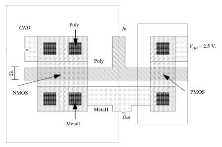
Figure 5.1 CMOS inverter layout.
