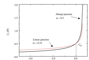
**Figure 3.8** Junction capacitance (in  $fF/\mu m^2$ ) as a function of the applied bias voltage.
