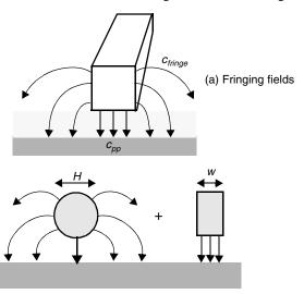
**Figure 4.4** The fringing-field capacitance. The model decomposes the capacitance into two contributions: a parallel-plate capacitance, and a fringing capacitance, modeled by a cylindrical wire with a diameter equal to the thickness of the wire.
