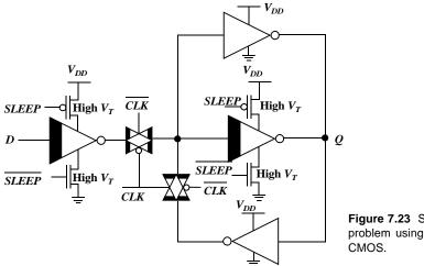
**Figure 7.23** Solving the leakage problem using multiple-threshold CMOS.
