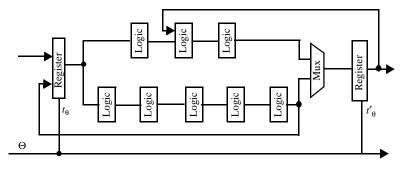
Figure 0.1 Sequential circuit.
