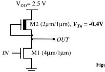
Figure 5.5 A depletion load NMOS inverter
