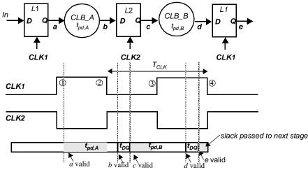
Figure 10.28 Example of slack-borrowing.
