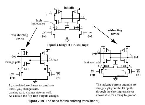
their value after the positive edge of *CLK* has occurred, resulting in either  $L_3$  or  $L_4$  being left in a high-impedance state with a logical low voltage level stored on the node. Without the leakage path that node would be susceptible to charging by leakage currents. The latch could then actually change state prior to the next rising edge of *CLK*! This is best illustrated graphically, as shown in Figure 7.39.
