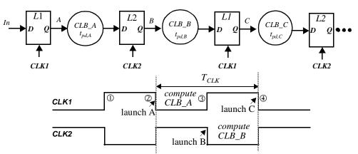
Figure 10.26 Latch-based design in which transparent latches are separated by combinational logic.
