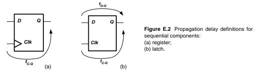
The characterization of the  $t_{C-Q}(t_{D-Q})$  delay is fairly straightforward. It consists of a delay measurement between the 50% transitions of *Clk* (*D*) and *Q*, for different values of the input slopes and the output loads.
