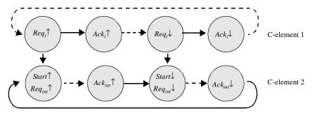
**Figure 10.45** State transition diagram for pipeline stage 1. The nodes represent the signaling events, while the arrows express dependencies. Arrows in dashed lines express actions in either the preceding or following stage.
