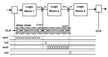
Figure 10.46 Application of self-timing for glitch reduction.
