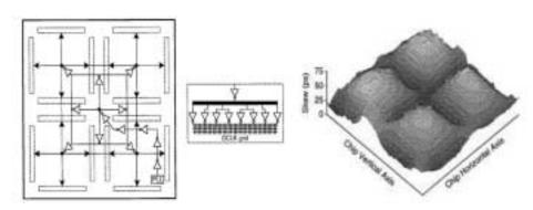
Figure 10.25 Global clock-distribution network in a window-pane structure.
