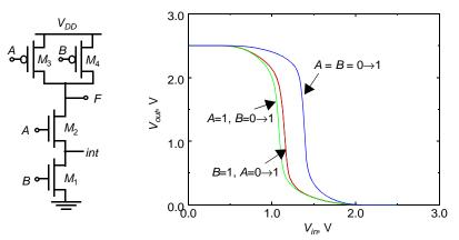
Figure 6.7 The VTC of a two-input NAND is data-dependent. NMOS devices are  $0.5\mu$ m/ $0.25\mu$ m while the PMOS devices are sized at  $0.75\mu$ m/ $0.25\mu$ m.
