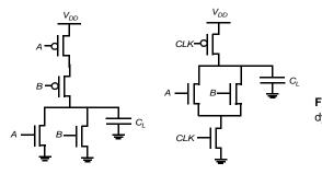
Figure 6.55 Static NOR versus n-type dynamic NOR.
