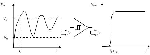
Figure 7.47 Noise suppression using a Schmitt trigger.
