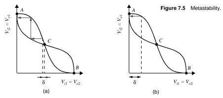
On the other hand, *A* and *B* are stable operation points, as demonstrated in Figure 7.5b. In these points, the **loop gain is much smaller than unity.** Even a rather large deviation from the operation point is reduced in size and disappears.
