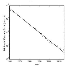
**Figure 3.39** Evolution of (average) minimum channel length of MOS transistors over time. Dots represent observed or projected (2000 and beyond) values. The continuous line represents a scaling scenario that reduces the minimum feature with a factor 2 every 5 years.
