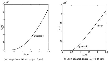
**Figure 3.20** NMOS transistor  $I_D$ - $V_{GS}$  characteristic for long and short-channel devices (0.25 µm CMOS technology). W/L = 1.5 for both transistors and  $V_{DS} = 2.5$  V.
