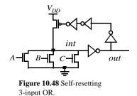
shown in Figure 10.48 [Bernstein98]. Assume that all inputs are low, and *int* is initially precharged. If A goes high, *int* will fall, causing out to go high. This causes, the gate to precharge. When the PMOS precharge device is active, the inputs must be in a reset state to avoid contention.
