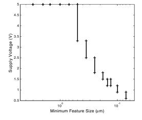
Figure 3.40 Evolution of min and max supplyvoltage in digital integrated circuits as a function of feature size. All values for 0.15 micron and below are projected.
