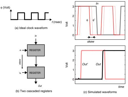
Figure 1.7 Impact of clock misalignment.
