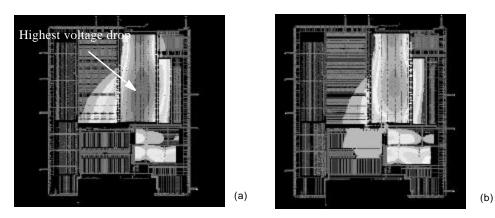
**Figure 9.15** Simulated IR voltage drop in power-distribution network of two versions of a complex digital integrated circuit. The gray-scale is used to indicate the severeness of the voltage drop. Adding an extra strap to the upper layers of the power network (b) helps to address the large voltage trop in the upper right module in the initial design (a).
