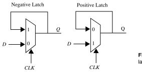
Figure 7.11 Negative and positive latches based on multiplexers.
