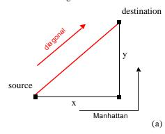
Figure 9.18 Manhattan versus diagonal routing.
