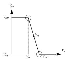
**Figure 5.2** A different approach to derive  $V_{IL}$  and  $V_{IH}$ .
