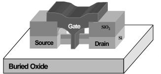
**Figure 3.41** FinFET dual-gated transistor with 25 nm channel length [Hu99].
