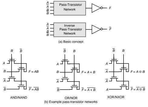
Figure 6.37 Complementary pass-transistor logic (CPL).
