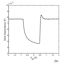
**Figure 3.31** Simulating the gate capacitance of an MOS transistor; (a) circuit configuration used for the analysis, (b) resulting capacitance plot for minimum-size NMOS transistor in  $0.25 \,\mu$ m technology.
