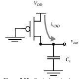
**Figure 5.25** Equivalent circuit during the low-to-high transition.
