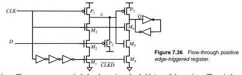
ister. The *transparency* period also determines the *hold time* of the register. The window must be wide enough for the input data to propagate to the Q output. In this particular circuit, the *set-up time* can be negative. This is the case if the transparency window is longer than the delay from input to output. This is attractive, as data can arrive at the register even after the clock goes high, which means that time is borrowed from the previous cycle.
