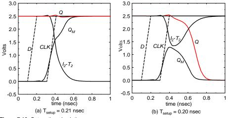
Figure 7.16 Set-up time simulation.
