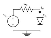
Figure 3.7 A simple diode circuit.
