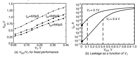
**Figure 6.72** Voltage Scaling  $(V_{DD}/V_T \text{ on delay and leakage})$
