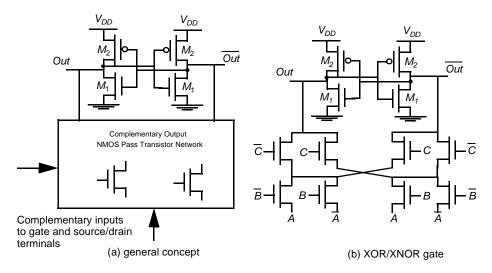
Figure 6.42 Swing-restored pass transistor logic [Parameswar96].
