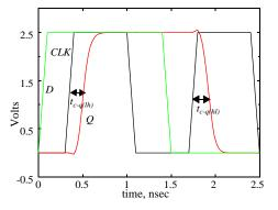
Figure 7.17 Simulation of propagation delay.
