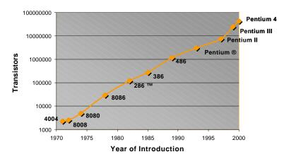
Figure 1.3 Historical evolution of microprocessor transistor count (from [Intel01]).
