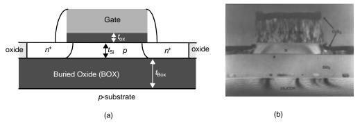
Figure 2.19 Silicon-on-insulator process- schematic diagram (a) and SEM cross-section (b).
