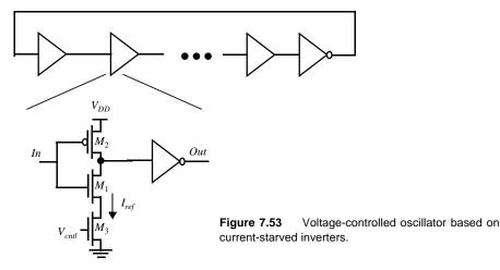
output. This can result in significant short-circuit current. This is resolved by feeding its output into a CMOS inverter or better yet a Schmitt trigger. An extra inverter is needed at the end to ensure that the structure oscillates.
