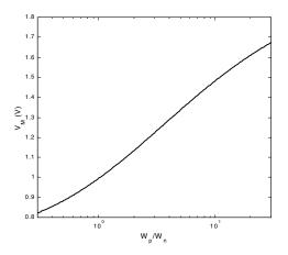
Figure 5.7 Simulated inverter switching threshold versus PMOS/NMOS ratio (0.25  $\mu$ m CMOS,  $V_{DD}$  = 2.5 V)
