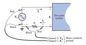
FIG. 26.7 Determining  $\mathbf{Z}_i$  using an oscilloscope.
