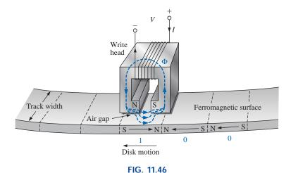
Hard disk storage using a U-shaped electromagnet write head.
