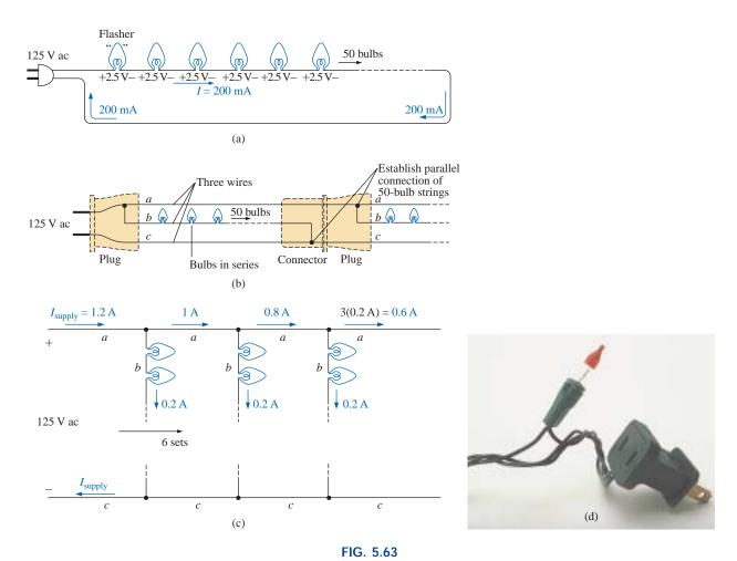
(a) Single-set wiring diagram; (b) special wiring arrangement; (c) redrawn schematic; (d) special plug and flasher unit.
