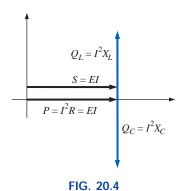
Power triangle for the series resonant circuit at resonance.
