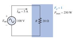
FIG. 14.30 Purely resistive load with  $F_p = 1$ .
