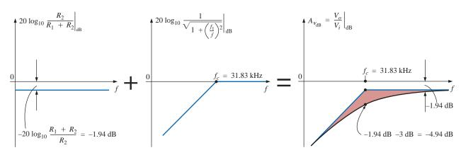
$$\begin{array}{c|c} & \textbf{FIG. 23.59} \\ Obtaining \ a \ dB \ plot \ of \ A_{V_{\text{dB}}} = \left. \frac{V_o}{V_i} \right|_{\text{dB}} \end{array}$$
