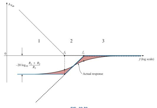
FIG. 23.72  $A_{v_{\rm dB}}$  versus frequency for the high-pass filter with limited attenuation of Fig. 23.68.
