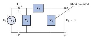
FIG. 26.40 Determining  $y_{11}$ .
