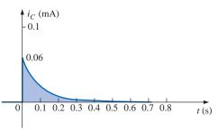
FIG. 24.21  $v_C$  and  $i_C$  for the network of Fig. 24.20.
