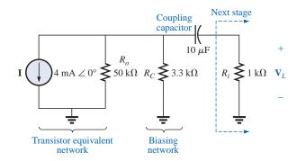
FIG. 16.10 Basic transistor amplifier.
