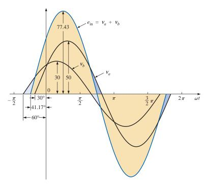
FIG. 14.66 Solution to Example 14.31.
