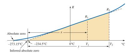
FIG. 3.14 Effect of temperature on the resistance of copper.
