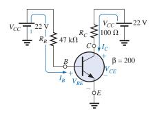
FIG. 18.92 dc equivalent of the transistor network of Fig. 18.91.
