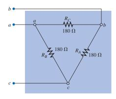
**FIG. 8.79** The  $\Delta$  equivalent for the Y of Fig. 8.78.
