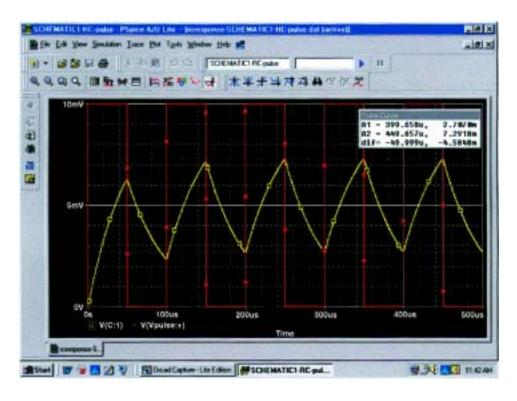
FIG. 24.50 Plot of  $v_C$  for the circuit of Fig. 24.47 with  $t_p = \tau = T/2$ .
