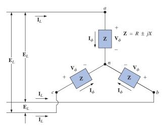
FIG. 22.22 Y-connected balanced load.
