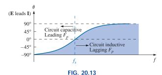
Phase plot for the series resonant circuit.
