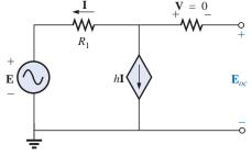
FIG. 18.77 Determining  $\mathbf{E}_{oc}$  for the network of Fig. 18.75.
