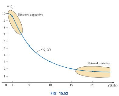
The magnitude of the voltage  $V_C$  versus frequency for the circuit of Fig. 15.45.
