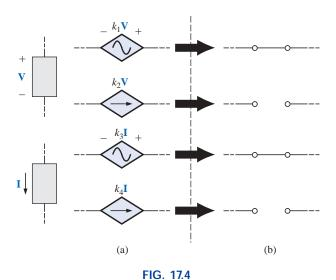
Conditions of V = 0 V and I = 0 A for a controlled source.
