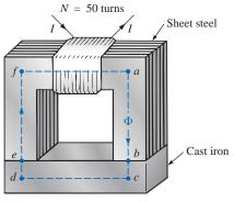
$\begin{array}{l} l_{ab} = l_{cd} = l_{ef} = l_{fa} = 4 \text{ in.} \\ l_{bc} = l_{de} = 0.5 \text{ in.} \\ \text{Area (throughout)} = 1 \text{ in.}^2 \\ \Phi = 3.5 \times 10^{-4} \, \text{Wb} \end{array}$
