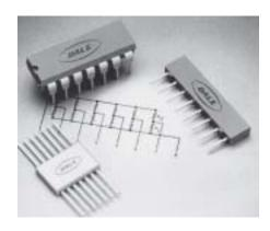
FIG. 3.22 Thick-film resistor networks. (Courtesy of Dale Electronics, Inc.)
