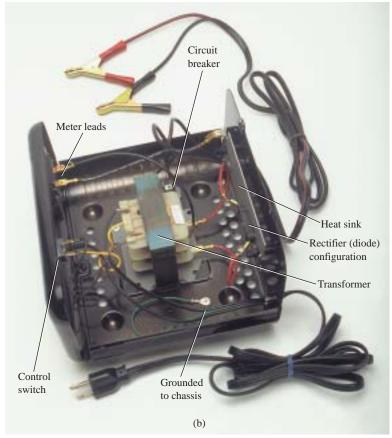
**FIG. 2.30**Battery charger: (a) external appearance; (b) internal construction.
