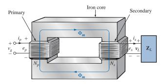
FIG. 21.4 *Iron-core transformer.*
