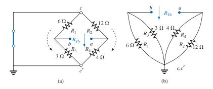
FIG. 9.46 Solving for  $R_{Th}$  for the network of Fig. 9.45.
