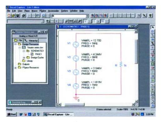
FIG. 25.28 Using PSpice to apply four terms of the Fourier expansion of a 10-V square wave to a load resistor of 1 k  $\Omega$ .
