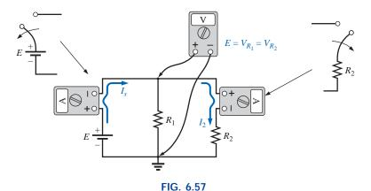
Setting up meters to measure the voltage and currents of a parallel network.
