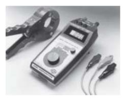
FIG. 19.31 Clamp-on power-factor meter. (Courtesy of the AEMC Corporation.)
