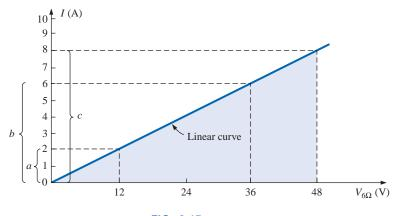
FIG. 9.15 Plotting I versus V for the 6- $\Omega$  resistor.
