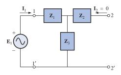
FIG. 26.28 Determining  $\mathbf{z}_{11}$ .
