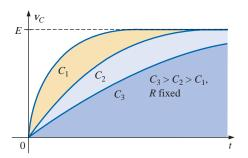
FIG. 10.33 Effect of C on the charging phase.
