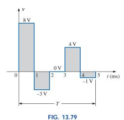
Waveform with five pulses to be analyzed by the C++ program of Fig. 13.78.
