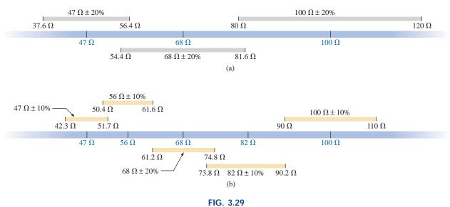
Guaranteeing the full range of resistor values for the given tolerance: (a) 20%; (b) 10%.
