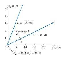
FIG. 14.22  $X_L$  versus frequency.
