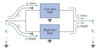
FIG. 23.38 Stop-band filter.
