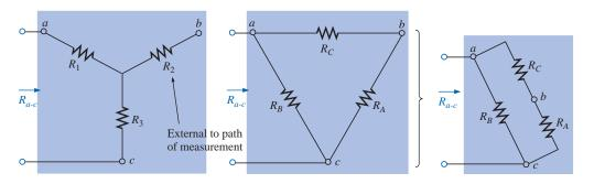
FIG. 8.74 Finding the resistance  $R_{a-c}$  for the Y and  $\Delta$  configurations.
