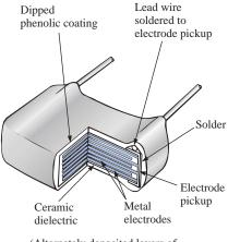
(Alternately deposited layers of ceramic dielectric material and metal electrodes fired into a single homogeneous block)
