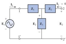
FIG. 26.30 Determining  $\mathbf{z}_{21}$ .
