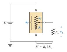
**FIG. 7.38** *Loaded potentiometer.*
