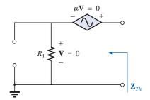
FIG. 18.51 Determining  $\mathbf{Z}_{Th}$  incorrectly.
