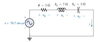
FIG. 15.35 Series R-L-C ac circuit.
