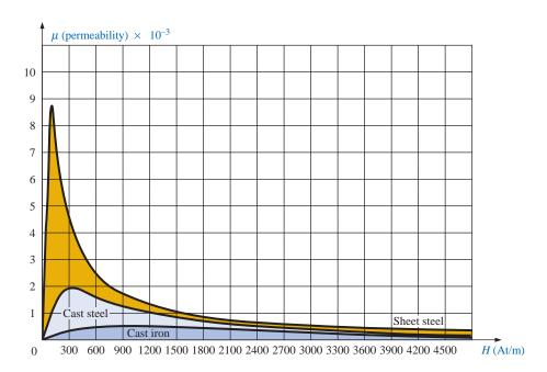
FIG. 11.19 Variation of  $\mu$  with the magnetizing force.
