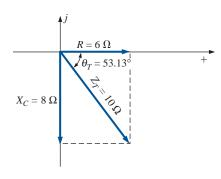
FIG. 15.32 Impedance diagram for the series R-C circuit of Fig. 15.30.
