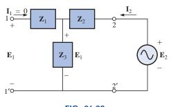
FIG. 26.29 Determining  $\mathbf{z}_{12}$ .
