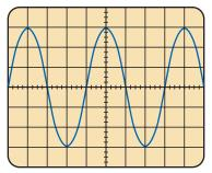
Vertical sensitivity = 50 mV/div.Horizontal sensitivity =  $10 \mu \text{s/div.}$
