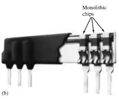
FIG. 10.14 Monolithic chip capacitors. (Courtesy of Vitramon, Inc.)
