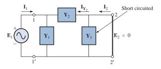
FIG. 26.42 Determining  $y_{21}$ .
