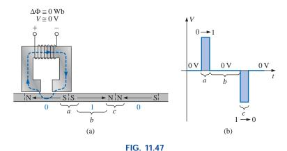
Reading the information off a hard disk using a U-shaped electromagnet.
