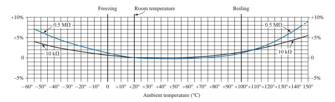
FIG. 3.19 Curves showing percentage temporary resistance changes from +20°C values. (Courtesy of Allen-Bradley Co.)
