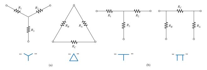
FIG. 8.72 The Y(T) and  $\Delta(\pi)$  configurations.
