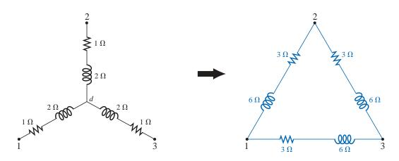
FIG. 17.53 Converting the Y configuration of Fig. 17.50 to a  $\Delta$ .
