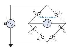
FIG. 17.45 Capacitance comparison bridge.
