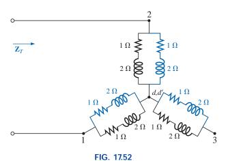
Substituting the Y configuration of Fig. 17.51 into the network of Fig. 17.50.
