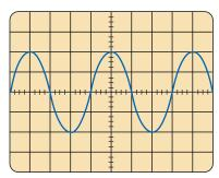
Vertical sensitivity = 0.1 V/div.Horizontal sensitivity =  $50 \mu\text{s/div.}$
