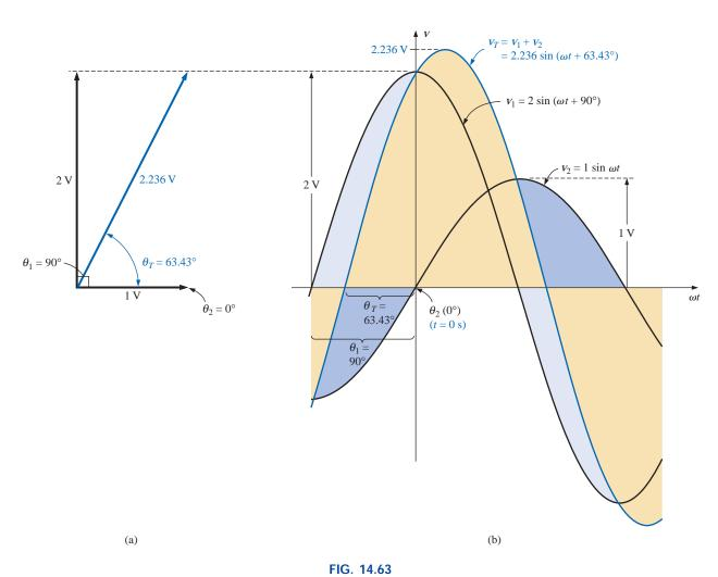
(a) The phasor representation of the sinusoidal waveforms of Fig. 14.63(b); (b) finding the sum of two sinusoidal waveforms of  $v_1$  and  $v_2$ .
