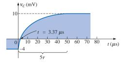
FIG. 24.23  $V_C$  for the network of Fig. 24.22.
