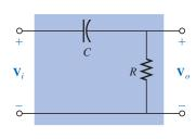
FIG. 23.19 High-pass filter.
