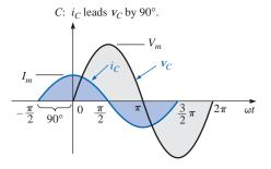
FIG. 14.12 The current of a purely capacitive element leads the voltage across the element by 90°.
