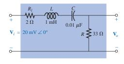
FIG. 23.35 Series resonant pass-band filter for Example 23.8.
