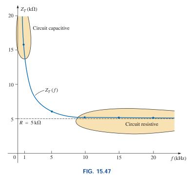
The magnitude of the input impedance versus frequency for the circuit of Fig. 15.45.
