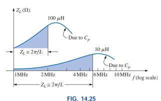
Z<sub>L</sub> versus frequency for the practical inductor equivalent of Fig. 14.24.
