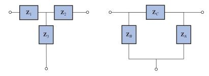
FIG. 17.47 The T and  $\pi$  configurations.
