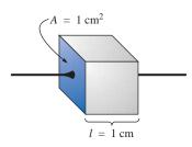
FIG. 3.11 Defining  $\rho$  in ohm-centimeters.
