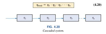
**EXAMPLE 4.13** Find the overall efficiency of the system of Fig. 4.19 if  $\eta_1 = 90\%$ ,  $\eta_2 = 85\%$ , and  $\eta_3 = 95\%$ .
