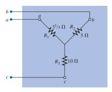
FIG. 8.77 The Y equivalent for the  $\Delta$  of Fig. 8.76.
