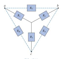
FIG. 17.46  $\Delta$ -Y configuration.
