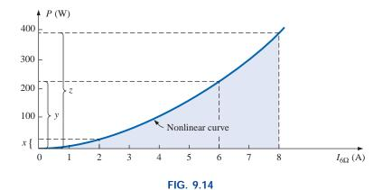
Plotting the power delivered to the 6- $\Omega$  resistor versus current through the resistor.
