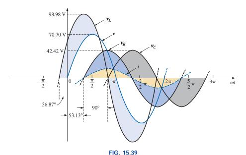
Waveforms for the series R-L circuit of Fig. 15.35.
