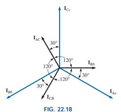
The phasor diagram of the currents of a three-phase,  $\Delta$ -connected generator.
