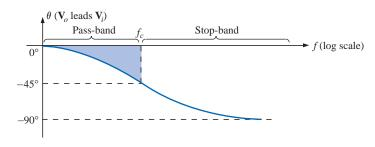
FIG. 23.13 Angle by which  $V_o$  leads  $V_i$ .
