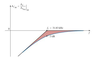
FIG. 23.58 dB plot for A' v for the high-pass filter of Fig. 23.55.
