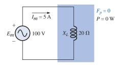
FIG. 14.31 Purely inductive load with  $F_p = 0$ .
