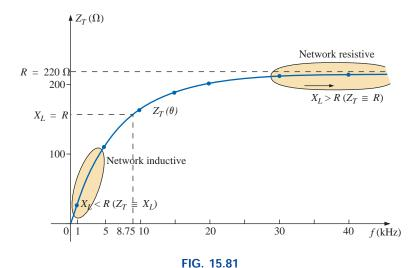
The magnitude of the input impedance versus frequency for the network of Fig. 15.79.
