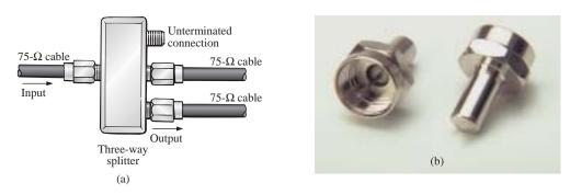
FIG. 16.27 Signal splitting: (a) three-way splitter; (b) F-type 75- $\Omega$  coax terminator.
