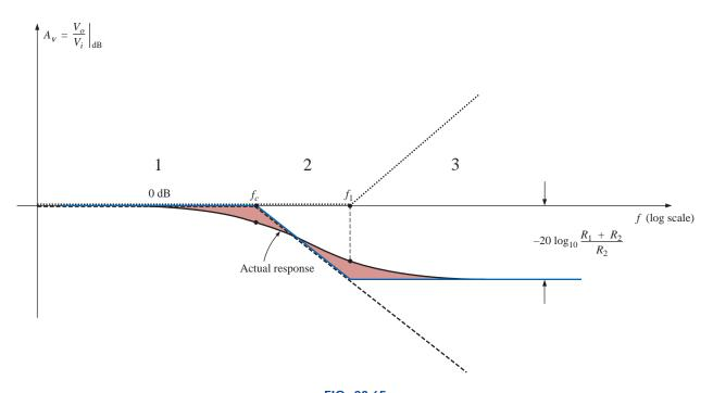
FIG. 23.65  $A_{V_{\rm dB}}$  versus frequency for the low-pass filter with limited attenuation of Fig. 23.62.
