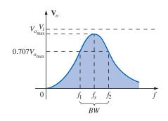
FIG. 23.33 Series resonant pass-band filter.
