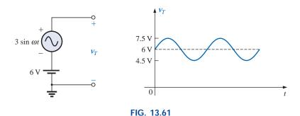
Generation and display of a waveform having a dc and an ac component.
