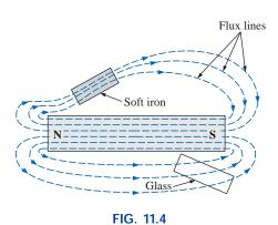
Effect of a ferromagnetic sample on the flux distribution of a permanent magnet.
