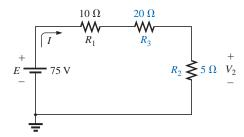
FIG. 5.20 Circuit of Fig. 5.19 with R<sub>2</sub> and R<sub>3</sub> interchanged.
