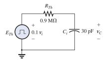
FIG. 24.39 Thévenin equivalent for  $C_i$  of Fig. 24.38.
