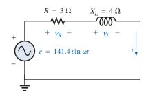
FIG. 15.26 Series R-L circuit.
