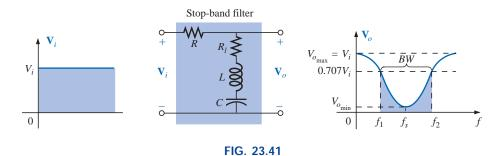
Stop-band filter using a series resonant circuit.
