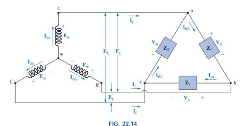
Y-connected generator with a  $\Delta$ -connected load.
