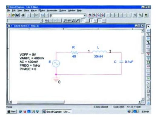
FIG. 20.42 Series resonant circuit to be analyzed using PSpice.
