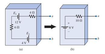
FIG. 9.25 The effect of applying Thévenin's theorem.
