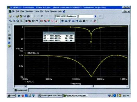
FIG. 23.97 *dB and magnitude plot for the voltage across*  $R_L$  *of the network of Fig. 23.95.*
