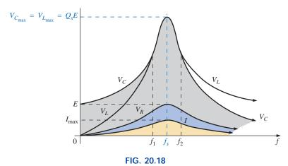
$V_R$ ,  $V_L$ ,  $V_C$ , and I for a series resonant circuit where  $Q_s \ge 10$ .
