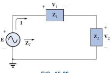
FIG. 15.25 Series ac circuit.
