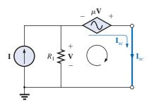
FIG. 18.52 Determining  $I_{sc}$  for the network of Fig. 18.50.
