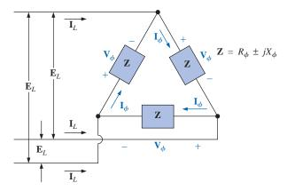
FIG. 22.24  $\Delta$ -connected balanced load.
