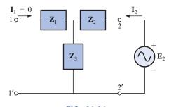
**FIG. 26.31** *Determining* **z**<sub>22</sub>.
