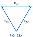
Demonstrating that the vector sum of the phase voltages of a three-phase generator is zero.
