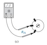
FIG. 9.56 Determining  $R_{Th}$  experimentally.
