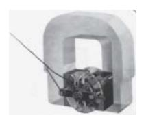
FIG. 7.42 d'Arsonval analog movement. (Courtesy of Weston Instruments, Inc.)
