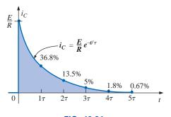
FIG. 10.31  $i_C$  versus t during the charging phase.
