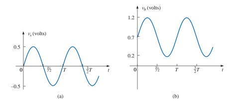
FIG. 18.96 Applied signal: (a) at the source; (b) at the base of the transistor.
