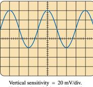
Vertical sensitivity = 20 mV/div. Horizontal sensitivity = 10  $\mu$ s/div.
