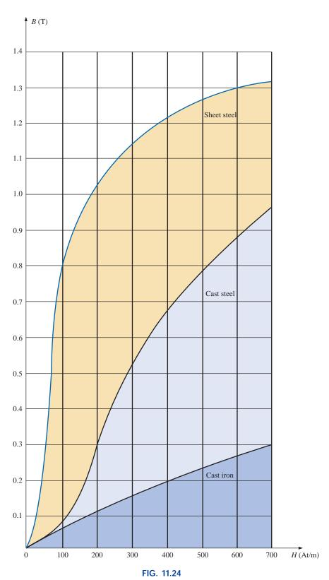
Expanded view of Fig. 11.23 for the low magnetizing force region.
