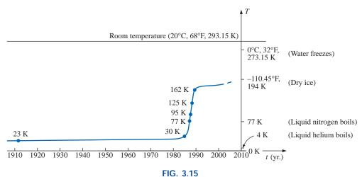
Rising temperatures of superconductors.
