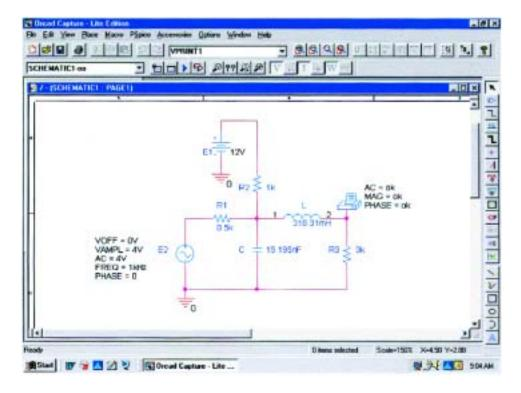
FIG. 18.97 Using PSpice to apply superposition to the network of Fig. 18.12.
