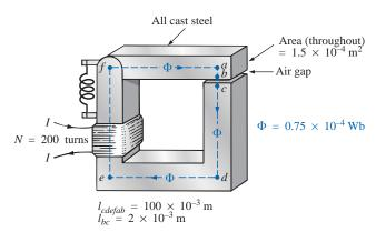
FIG. 11.36 Relay for Example 11.6.
