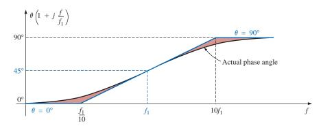
**FIG. 23.66** *Phase angle for*  $(1 + j (f/f_1))$ .
