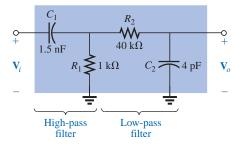
FIG. 23.30 Pass-band filter.
