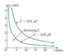
FIG. 14.23  $X_C$  versus frequency.
