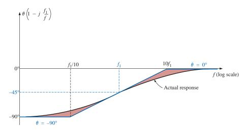
**FIG. 23.73** *Phase angle for*  $(1 - j (f_1/f))$ .
