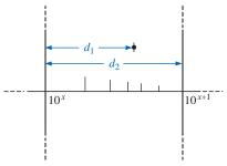
FIG. 23.3 Finding a value on a log plot.
