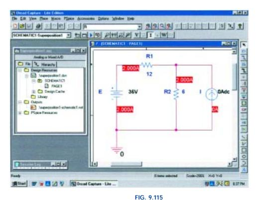
Using PSpice to determine the contribution of the 36-V voltage source to the current through  $R_2$ .
