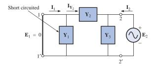
FIG. 26.41 Determining  $y_{12}$ .
