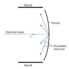
FIG. 12.56 Secondary emission from and protective measures for a TV or PC monitor.
