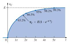
FIG. 10.32  $V_C$  versus t during the charging phase.
