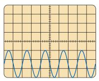
Vertical sensitivity = 10 mV/div. Horizontal sensitivity = 0.2 ms/div.
