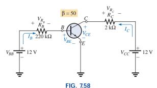
dc bias levels of a transistor amplifier.
