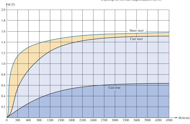
**FIG. 11.23** *Normal magnetization curve for three ferromagnetic materials.*
