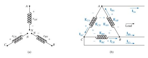
FIG. 22.16 Δ-connected generator.
