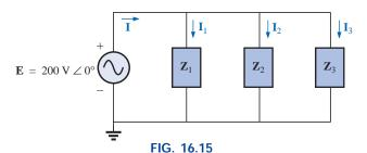
$Network\ of\ Fig.\ 16.14\ following\ the\ assignment\ of\ the\ subscripted\ impedances.$
