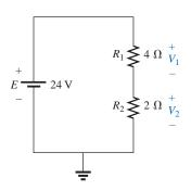
FIG. 5.49 Circuit of Fig. 5.48 redrawn.
