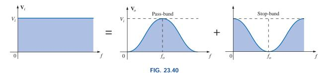
Demonstrating how an applied signal of fixed magnitude can be broken down into a pass-band and stop-band response curve.
