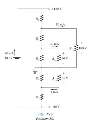
\*30. Determine the voltage divider supply resistors for the configuration of Fig. 7.93. Also determine the required wattage rating for each resistor, and compare their levels.
