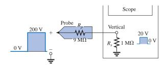
FIG. 24.36 ×10 attenuator probe.
