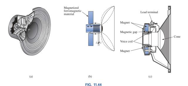
Coaxial high-fidelity loudspeaker: (a) construction; (b) basic operation; (c) cross section of actual unit. (Courtesy of Electro-Voice, Inc.)
