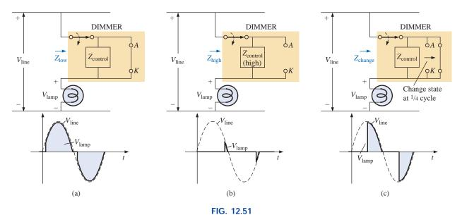
Basic operation of the dimmer of Fig. 12.50: (a) full voltage to the lamp; (b) approaching the cutoff point for the bulb; (c) reduced illumination of the lamp.
