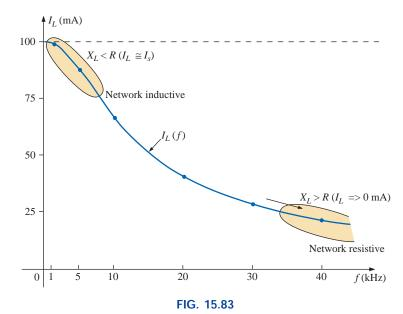
The magnitude of the current  $I_L$  versus frequency for the parallel R-L network of Fig. 15.79.
