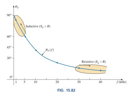
The phase angle of the input impedance versus frequency for the network of Fig. 15.79.
