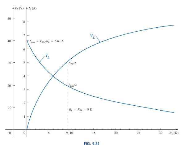
$V_L$  and  $I_L$  versus  $R_L$  for the network of Fig. 9.79.
