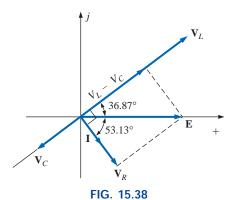
Phasor diagram for the series R-L-C circuit of Fig. 15.35.
