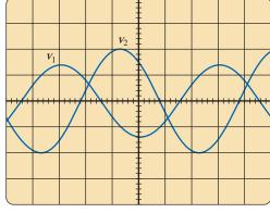
Vertical sensitivity = 2 V/div. Horizontal sensitivity =  $10 \mu \text{s/div}$ .
