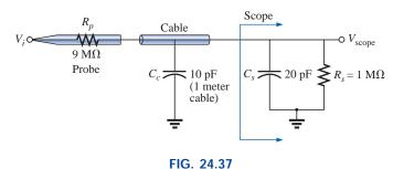
Capacitive elements present in an attenuator probe arrangement.
