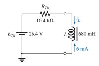
FIG. 12.37 Thévenin equivalent circuit for the network of Fig. 12.36 for  $t \ge 0$  s.
