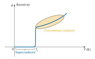
FIG. 3.16 Defining the critical temperature  $T_c$ .
