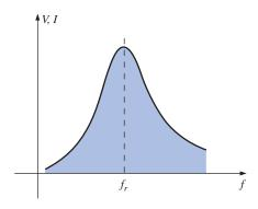
FIG. 20.1 Resonance curve.
