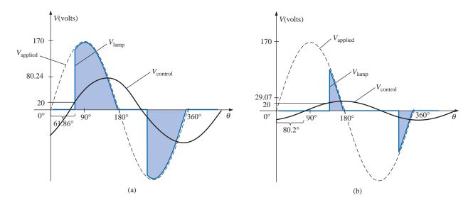
**FIG. 15.108**Light dimmer of Fig. 12.49: (a) rheostat set at 33 k $\Omega$ ; (b) rheostat set at 200 k $\Omega$ .
