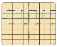
Vertical sensitivity = 10 mV/div.Horizontal sensitivity =  $10 \mu \text{s/div.}$
