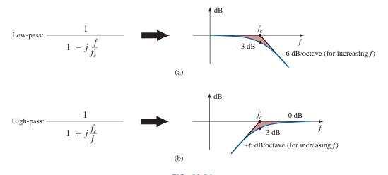
FIG. 23.54 dB response of (a) low-pass filter and (b) high-pass filter.
