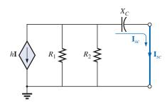
FIG. 18.48 Determining the short-circuit current for the network of Fig. 18.46.
