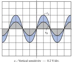
$e_g$ : Vertical sensitivity — 0.2 V/div.  $v_{R_s}$ : Vertical sensitivity — 10 mV/div.
