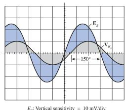
$E_g$ : Vertical sensitivity = 10 mV/div.  $V_{R_s}$ : Vertical sensitivity = 1 mV/div. (b)
