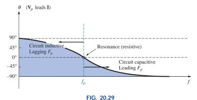
Phase plot for the parallel resonant circuit.
