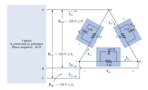
FIG. 22.20 Example 22.3:  $\Delta$ - $\Delta$  system.
