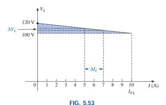
$V_L$  versus  $I_L$  for a dc generator with  $R_{int} = 2 \Omega$ .
