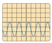
Vertical sensitivity = 0.2 V/div. Horizontal sensitivity =  $50 \mu\text{s/div}$ .
