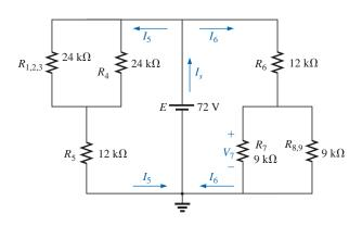
FIG. 7.23 Network of Fig. 7.22 redrawn.
