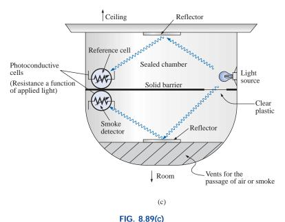
Wheatstone bridge smoke detector: (c) internal construction.
