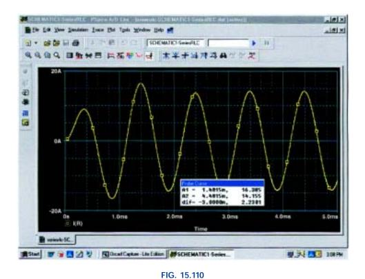
A plot of the current for the circuit of Fig. 15.109 showing the transition from the transient state to the steady-state response.
