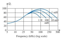
FIG. 20.6  $Q_l$  versus frequency for a series of inductors of similar construction.
