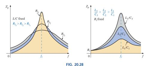
Effect of  $R_b$ , L, and C on the parallel resonance curve.
