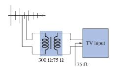
FIG. 21.9 Television impedance matching transformer.
