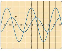
$\label{eq:Vertical sensitivity} Vertical sensitivity = 0.5 \ V/div.$  Horizontal sensitivity = 0.2 ms/div. (I)
