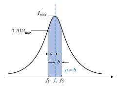
FIG. 20.16 Approximate series resonance curve for  $Q_s \ge 10$ .
