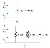
**25.** Find the total admittance and impedance of the circuits of Fig. 15.135. Identify the values of conductance and susceptance, and draw the admittance diagram.
