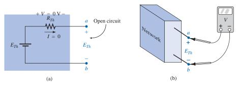
FIG. 9.55 Determining  $E_{Th}$  experimentally.
