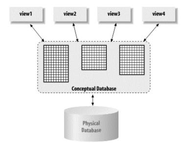
At the lowest level of the structure is the *physical database*, which consists of the raw data existing on a physical object, such as a hard disk. At this level, the data has no logical meaning, as related to the database. However, the data does have a very definite physical structure to allow efficient access. In other words, the data is more than just a string of bits.
