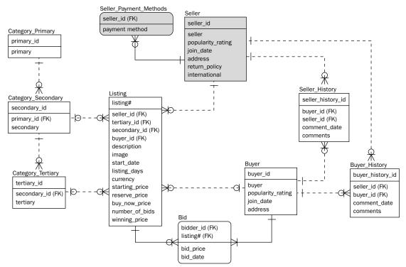
Figure 10-20: Applying 4NF to the OLTP database model.
