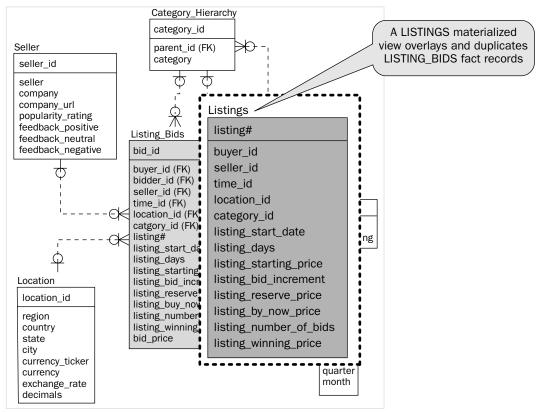
Figure 11-5: Refining facts and dimensions using materialized views to replace fact hierarchical structures.
