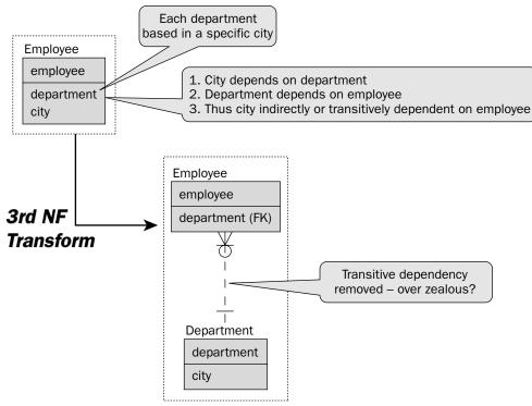
Figure 4-26: 3NF transitive dependency separation from one table to a new table.
