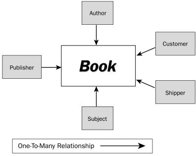
Figure 6-17: A data warehouse database model star schema.
