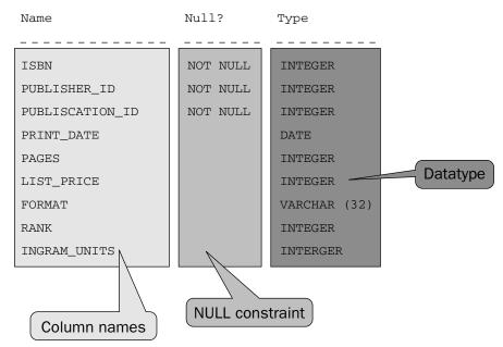
Figure 3-5: The vertical structure of a table showing fields, constraints and datatypes.
