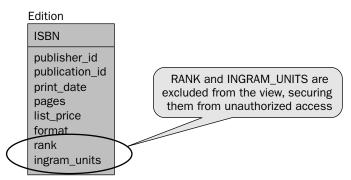
Figure 8-2: Views can be used to provide restricted access.
