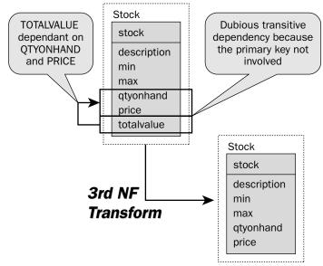
Figure 4-27: 3NF transformation to remove calculated fields.
