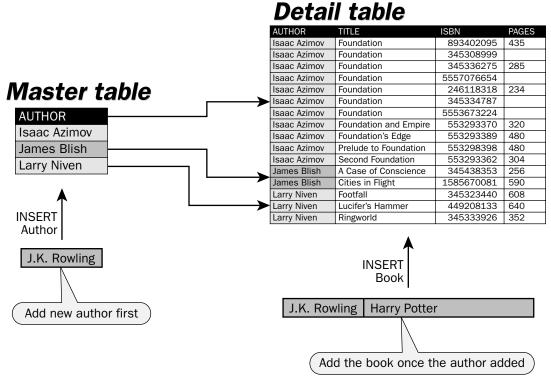
Figure 4-1: Insert anomaly occurs when detail record added with no master record.
