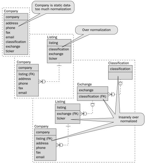
Figure 6-11: Denormalization of 2NF into a single static table.
