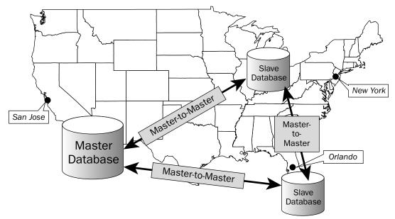
Figure 13-8: Replication can be both master-to-slave and master-to-master.
