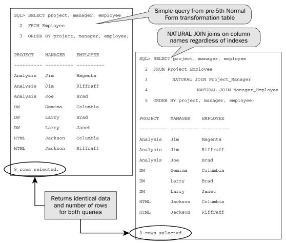
Figure 4-44: 5NF transformations must return records identical to the pre-5NF transformation when joined.
