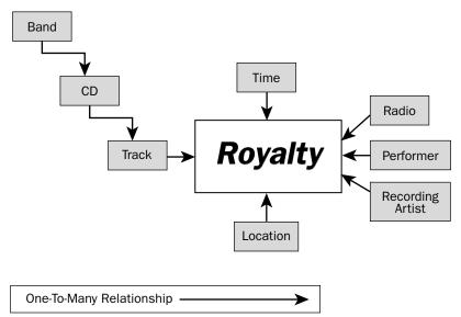
Figure 7-13: A data warehouse snowflake schema.
