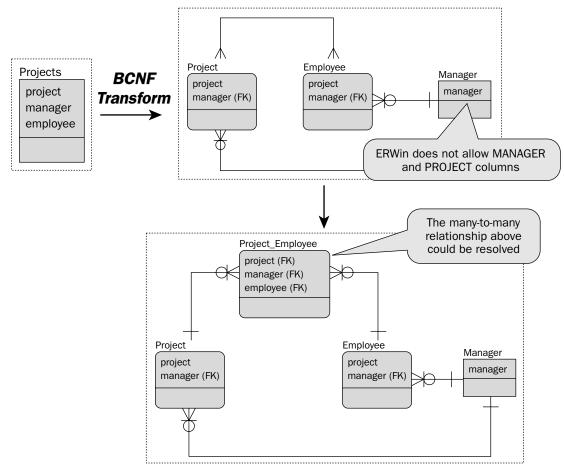
Figure 4-34: A common type of BCNF transformation example.
