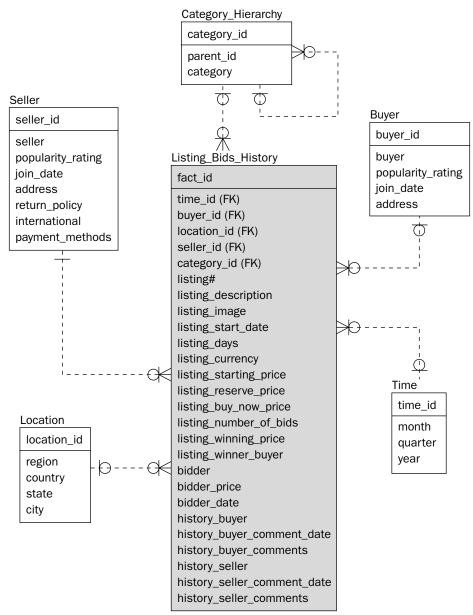
Figure 10-12: The data warehouse database model ERD.
