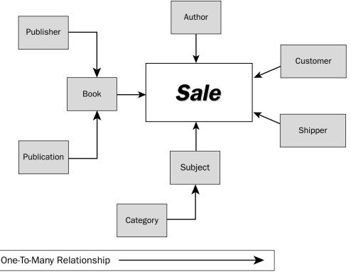
A more simplistic equivalent diagram to that of Figure 7-4 is shown by the snowflake schema in Figure 7-5.
