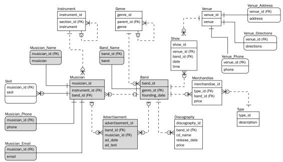
Figure 10-31: Refining the database model with normalization.
