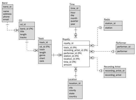
Figure 7-14: A data warehouse snowflake schema ERD.
