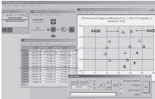
Figure 8.4 Scatterplot output of the symbolic descriptions stored in the enviro SODAS file, such that the Euclidean distance between the points preserves the dissimilarity values computed by the DISS module.
