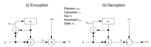
Figure 6.1: General model of a synchronous stream cipher.
