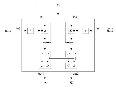
**Figure 9.4:** Compression function of MDC-2 hash function. E = DES.
