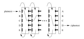
Figure 7.4: A rotor-based machine.
