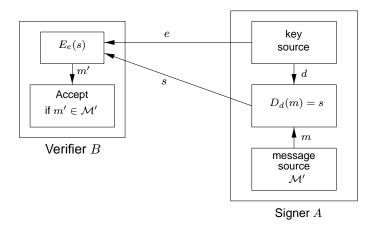
Figure 1.14: A digital signature scheme with message recovery.
