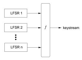
Figure 6.8: A nonlinear combination generator. f is a nonlinear combining function.
