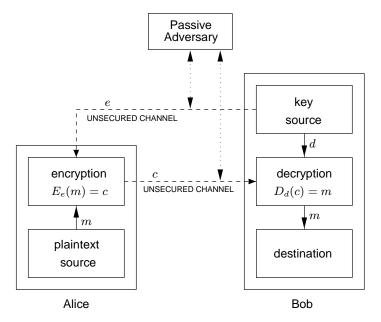
**Figure 1.11:** Encryption using public-key techniques.
