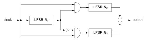
**Figure 6.12:** The alternating step generator.
