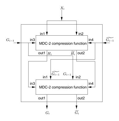
Figure 9.5: Compression function of MDC-4 hash function
