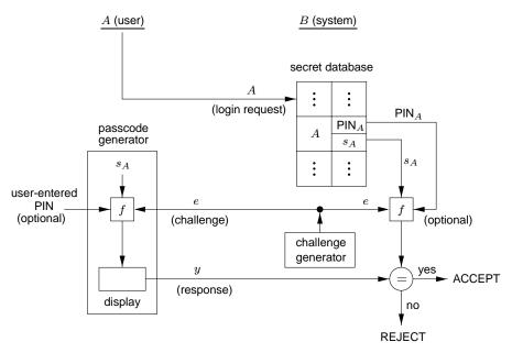
**Figure 10.3:** Functional diagram of a hand-held passcode generator.  $s_A$  is A's user-specific secret. f is a one-way function. The (optional) PIN could alternatively be locally verified in the passcode generator only, making g independent of it.
