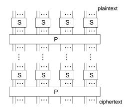
Figure 7.7: Substitution-permutation (SP) network.
