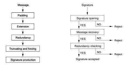
Figure 11.5: Signature and verification processes for ISO/IEC 9796.
