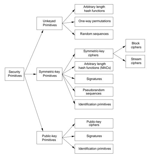
Figure 1.1: A taxonomy of cryptographic primitives.
