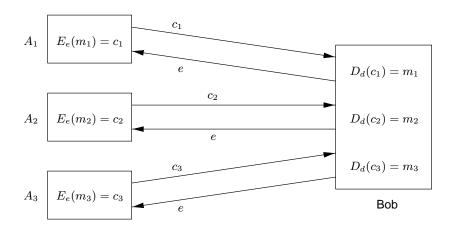
Figure 1.12: Schematic use of public-key encryption.
