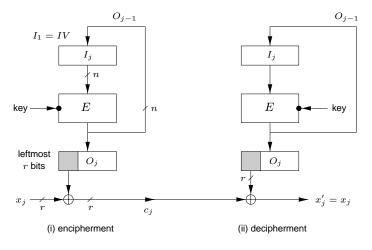
**Figure 7.1:** Common modes of operation for an n-bit block cipher.
