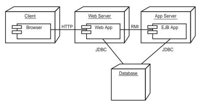
FIGURE 13.1 An N-tier application deployment diagram.
