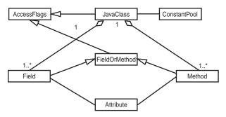
FIGURE 17.2 Class diagram of BCEL's main classes.
