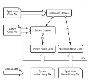
FIGURE 14.1 The JVM from a class loading perspective.
