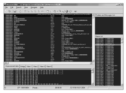
**FIGURE 18.1** PE Explorer showing the disassembled code of getPhysicalTotal().
