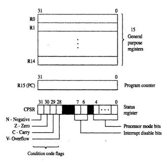
Figure 3.1 ARM register structure,
