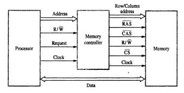
Figure 5.11 Use of a memory controller.
