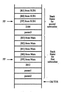
Figure 2.29 Stack frames for Figure 2.28.
