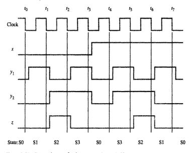
Figure A.51 Timing diagram for the circuit in Figure A.50.
