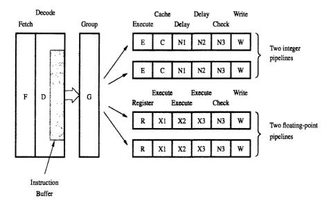
Figure 8.24 Pipeline organization of the UltraSPARC II processor.
