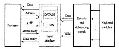
Figure 4.28 Keyboard to processor connection.
