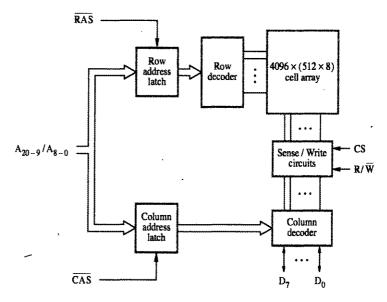
Figure 5.7 Internal organization of a 2M × 8 dynamic memory chip.
