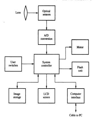
Figure 9.2 A simplified block diagram of a digital camera.
