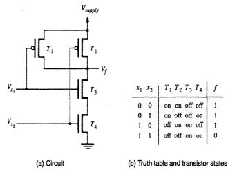
Figure A.17 CMOS realization of a NAND gate.
