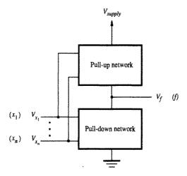
Figure A.16 Structure of a CMOS circuit.
