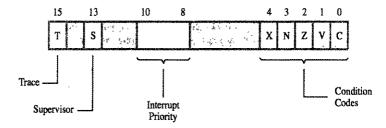
Figure 4.14 Processor status register in the 68000 processor.
