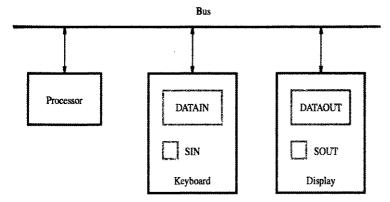
Figure 2.19 Bus connection for processor, keyboard, and display.
