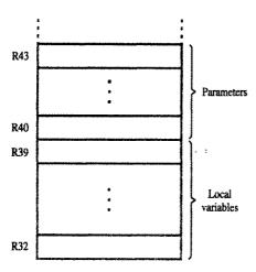
(a) Active register area in the main program after execution of Alloc 8,4
