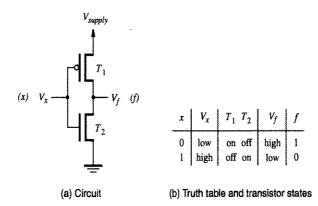
Figure A.15 CMOS realization of a NOT gate.
