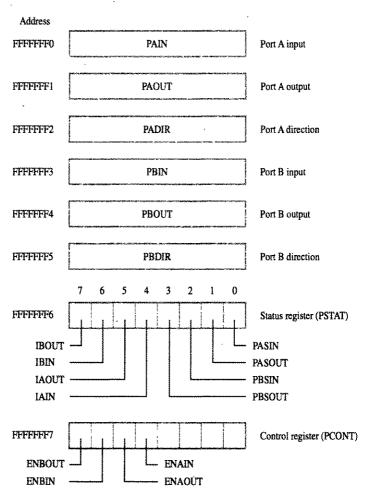
Figure 9.6 Parallel interface registers.
