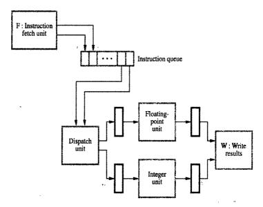
Figure 8.19 A processor with two execution units.
