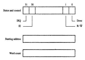
Figure 4.18 Registers in a DMA interface.
