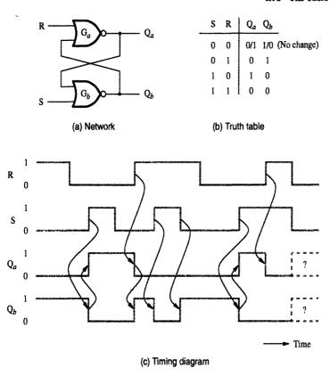
Figure A.24 A basic latch implemented with NOR gates.
