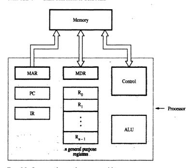
Figure 1.2 Connections between the processor and the memory.
