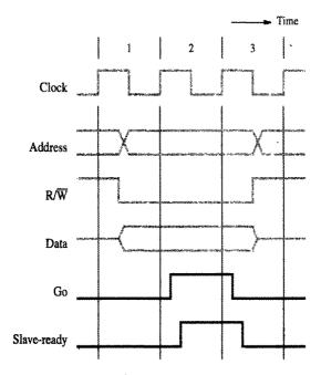
Figure 4.36 Timing for the output interface in Figure 4.35.
