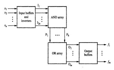
Figure A.40 A block diagram for a PLD.
