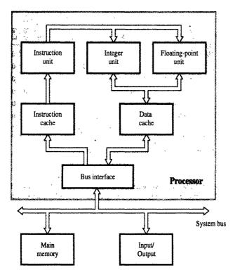
Figure 7.14 Block diagram of a complete processor.
