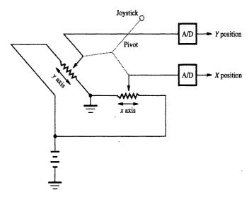
Figure 10.1 Joystick, using potentiometers as position transducers.
