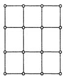
Figure 12.8 A 2-dimensional mesh network.
