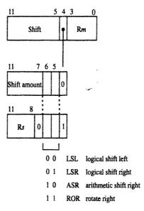
Figure B.3 ARM shift operations on operand 2 (Figure B.2) or address offset (Figure B.5) contained in register Rm.
