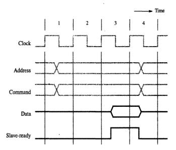
Figure 4.25 An input transfer using multiple clock cycles.
