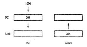
Figure 2.24 Subroutine linkage using a link register.
