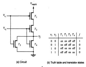
Figure A.18 CMOS realization of a NOR gate.
