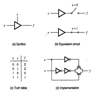
Figure A.22 Tri-state buffer.
