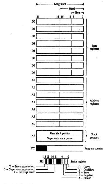
Figure 3.18 The 68000 register structure.
