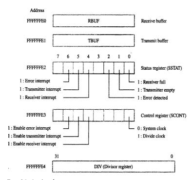
Figure 9.8 Serial interface registers.
