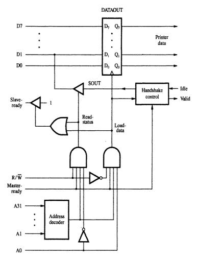
Figure 4.32 Output interface circuit.
