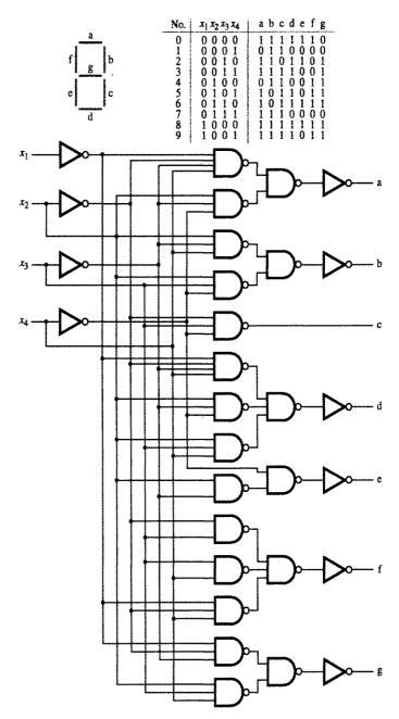
Figure A.37 A BCD to seven-segment display decoder.
