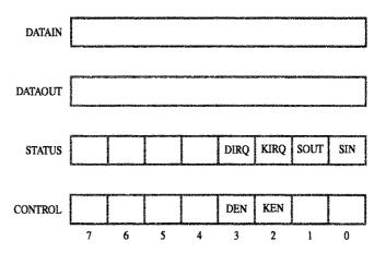
Figure 4.3 Registers in keyboard and display interfaces.
