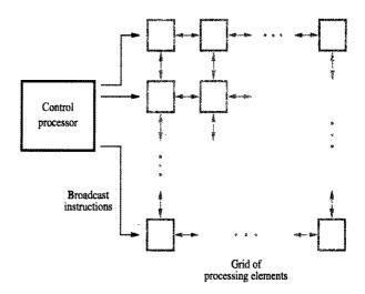
Figure 12.1 An array processor.
