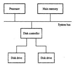
Figure 5.31 Disks connected to the system bus.
