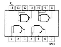
(b) Schematic of an integrated circuit providing four 2-input NAND gates
