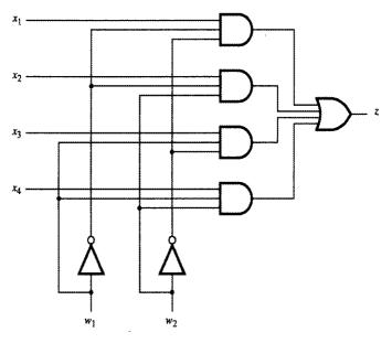
Figure A.38 A four-input multiplexer.
