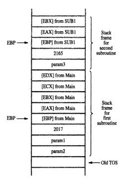
Figure 3.48 IA-32 stack frames for Figure 3.47.
