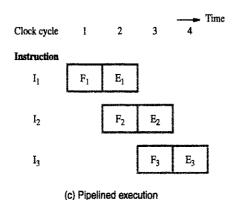
Figure 8.1 Basic idea of instruction pipelining.
