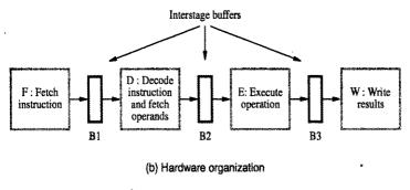
Figure 8.2 A 4-stage pipeline.
