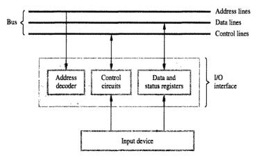
Figure 4.2 I/O interface for an input device.
