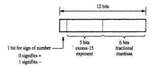
Figure P6.2 Floating-point format used in Problem 6.25.
