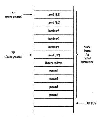
Figure 2.27 A subroutine stack frame example.
