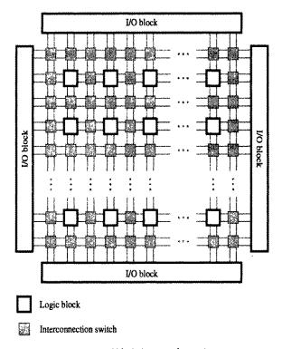
Figure A.46 A conceptual block diagram of an FPGA.
