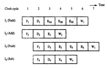
Figure 8.20 An example of instruction execution flow in the processor of Figure 8.19, assuming no hazards are encountered.
