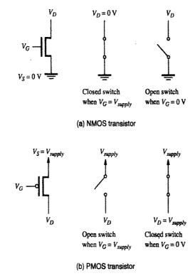
Figure A.14 NMOS and PMOS transistors in logic circuits.
