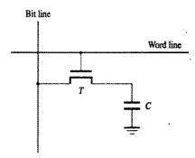
Figure 5.6 A single-transistor dynamic memory cell.
