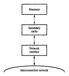
Figure 12.12 A processor node for the multiprocessor organization in Figure 12.2.
