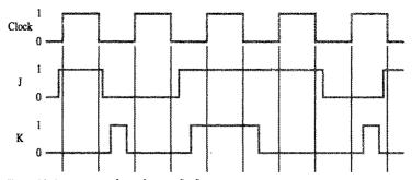
Figure PA.4 Input waveforms for a JK flip-flop.
