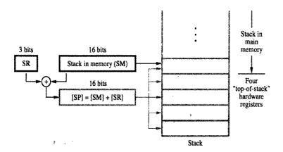
Figure 11.10 Top-of-stack structure in the HP3000.
