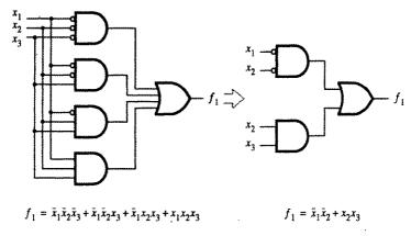
Figure A.4 A logic network for f<sub>1</sub> of Table A.1 and an equivalent minimal network.
