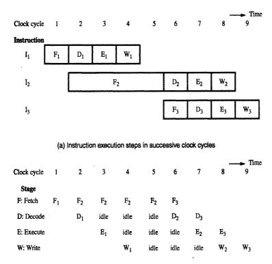
(b) Function performed by each processor stage in successive clock cycles
