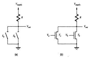
Figure A.12 A transistor circuit implementation of a NOR gate.
