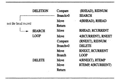
Figure 2.38 A subroutine for deleting a record from a linked list.
