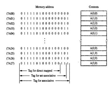
Figure 5.18 An array stored in the main memory.
