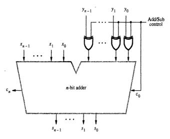
Figure 6.3 Binary addition-subtraction logic network.
