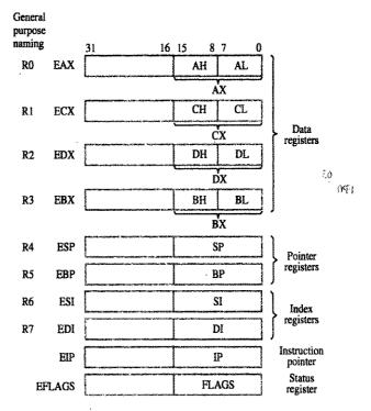
Figure 3.38 Compatibility of the IA-32 register structure with earlier Intel processor register structures.
