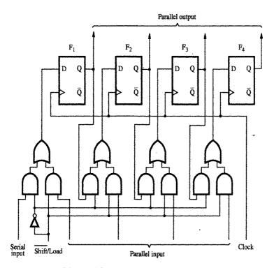
Figure A.34 Parallel-access shift register.
