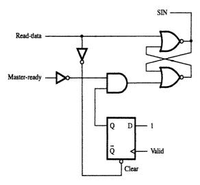
Figure 4.30 Circuit for the status flag block in Figure 4.29.
