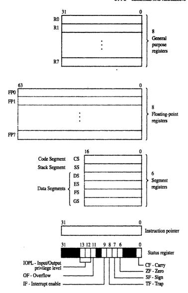
Figure 3.37 | A-32 register structure.
