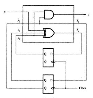
Figure A.50 Implementation of the up/down counter.
