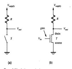
Figure A.11 An inverter circuit.
