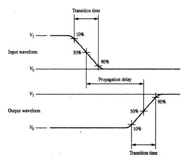
Figure A.21 Definition of propagation delay and transition time.
