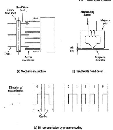
Figure 5.29 Magnetic disk principles.
