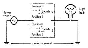
(a) Light bulb controlled by two switches
