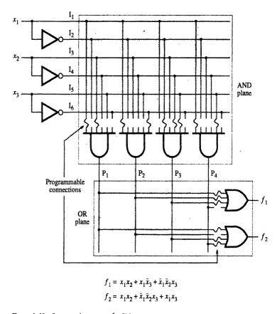
Figure A.41 Functional structure of a PLA.
