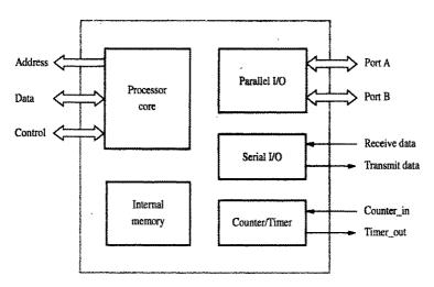
Figure 9.4 An example microcontroller.
