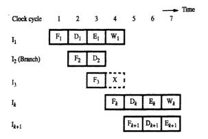
(b) Branch address computed in Decode stage
