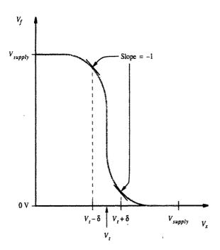
Figure A.20 The voltage transfer characteristic for the CMOS inverter.
