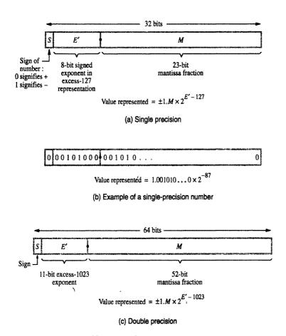
Figure 6.24 IEEE standard floating-point formats.
