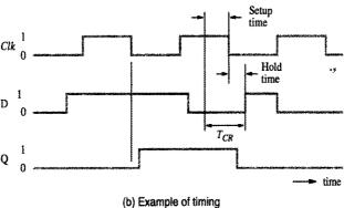
Figure A.29 A negative edge-triggered D flip-flop.
