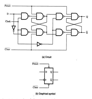
Figure A.32 Master-slave D flip-flop with Preset and Clear.
