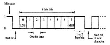
Figure 10.3 Asynchronous serial character transmission.
