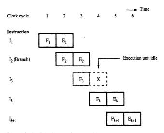
Figure 8.8 An idle cycle caused by a branch instruction.
