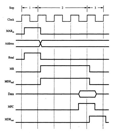
Figure 7.5 Timing of a memory Read operation.
