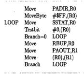
Figure 9.13 Possible compiled code for the program segment in Figure 9.12.
