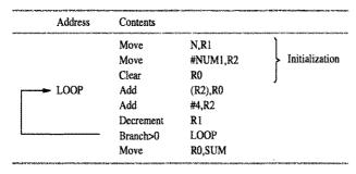
Figure 2.12 Use of indirect addressing in the program of Figure 2.10.
