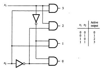
Figure A.36 A two-input to four-output decoder.
