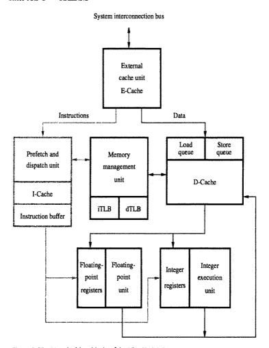
Figure 8.23 Main building blocks of the UltraSPARC II processor.
