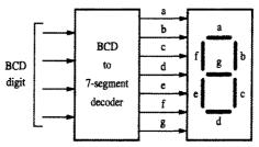
Figure P9.1 A 7-segment display with a BCD decoder.
