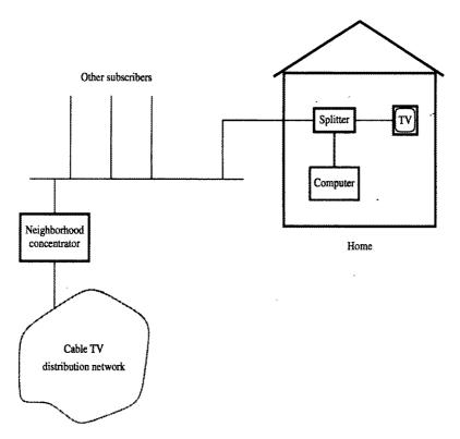
Figure 10.6 A cable-modern connection.
