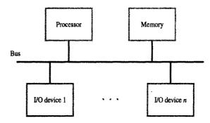
Figure 4.1 A single-bus structure.
