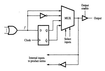
Figure A.44 An example of the output of a PAL element.
