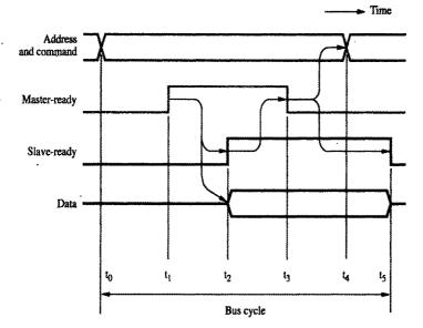
Figure 4.26 Handshake control of data transfer during an input operation.
