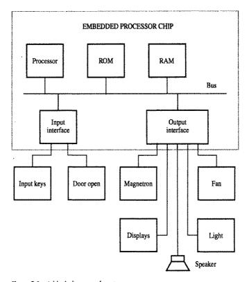
Figure 9.1 A block diagram of a microwave oven.
