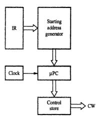
Figure 7.16 Basic organization of a microprogrammed control unit.
