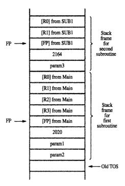
Figure 3.13 ARM stack frames for Figure 3.12.
