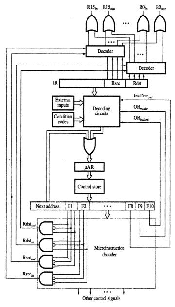
Figure 7.25 Some details of the control-signal-generating circuitry.
