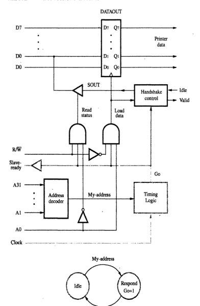
Figure 4.35 A parallel port interface for the bus of Figure 4.25, with a state-diagram for the timing logic.
