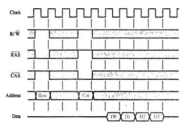
Figure 5.9 Burst read of length 4 in an SDRAM.
