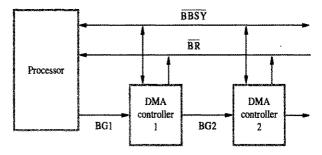
Figure 4.20 A simple arrangement for bus arbitration using a daisy
