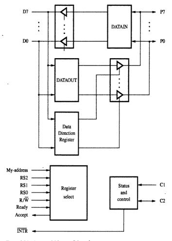
Figure 4.34 A general 8-bit parallel interface.
