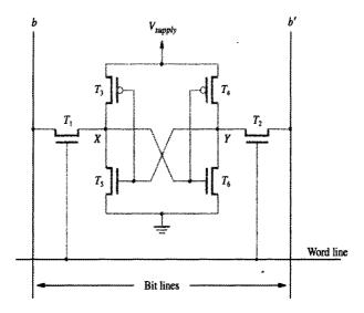
Figure 5.5 An example of a CMOS memory cell.
