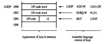
[PC] = 1006 when branch address is computed Branch address = 1006 - 6 = 1000
