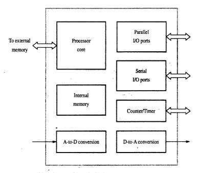
Figure 9.3 A block diagram of an embedded processor.
