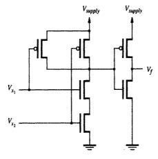
Figure A.19 CMOS realization of an AND gate.
