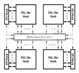
Figure A.45 Structure of a complex programmable logic device (CPLD).
