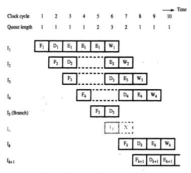
Figure 8.11 Branch timing in the presence of an instruction queue. Branch target address is computed in the D stage.
