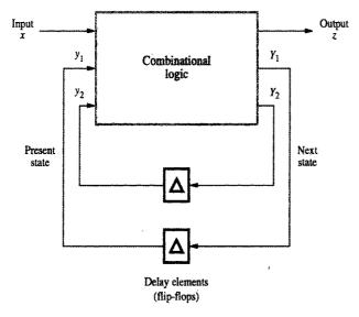
Figure A.52 A formal model of a finite state machine.
