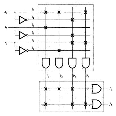
Figure A.42 A simplified sketch of the PLA in Figure A.41.
