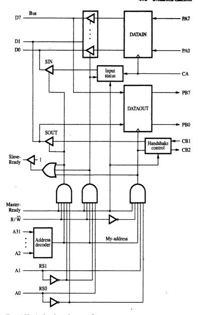
Figure 4.33 Combined input/output interface circuit.
