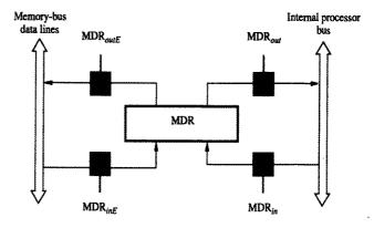
Figure 7.4 Connection and control signals for register MDR.
