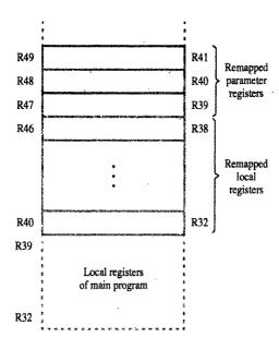
(b) Active register area in the subroutine after execution of Alloc 7,3
