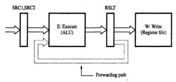
(b) Position of the source and result registers in the processor pipeline
