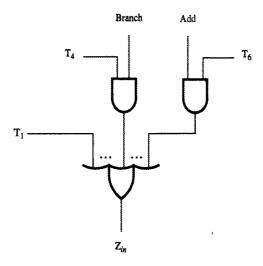
Figure 7.12 Generation of the Z<sub>in</sub> control signal for the processor in Figure 7.1.
