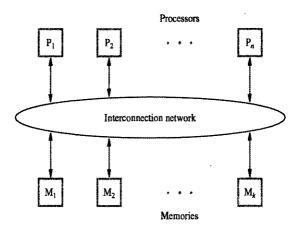
Figure 12.2 A UMA multiprocessor.
