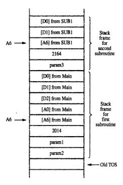
Figure 3.31 68000 stack frames for Figure 3.30.
