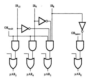
Figure 7.26 Control circuits, for bit-ORing (part of the decoding circuits in Figure 7.25).
