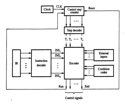
Figure 7.11 Separation of the decoding and encoding functions.
