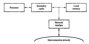
Figure 12.13 Node structure for the multiprocessor organization in Figure 12.3.
