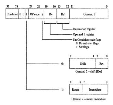
Figure 8.2 ARM arithmetic, logic, compare, test, and move instructions.
