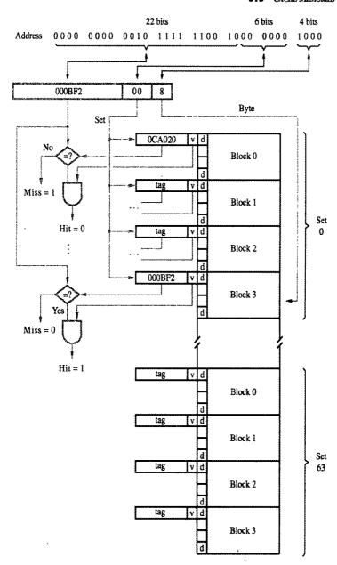
Figure 5.23 Data cache organization in the 68040 microprocessor.
