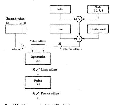
Figure 11.2 Address generation in the IA-32 architecture.
