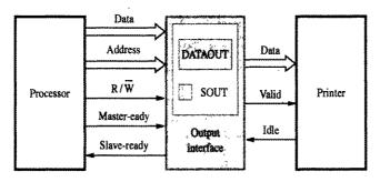
Figure 4.31 Printer to processor connection.
