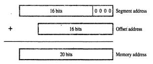
Figure 11.1 Generation of a memory address in the 8086 processor.
