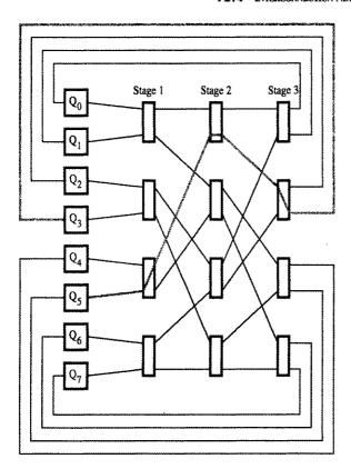
Figure 12.6 Multistage shuffle network.
