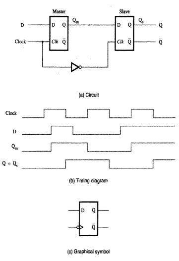
Figure A.28 Master-slave D flip-flop.
