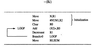
Figure 2.16 The Autoincrement addressing mode used in the program of Figure 2.12.
