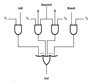
Figure 7.13 Generation of the End control signal.
