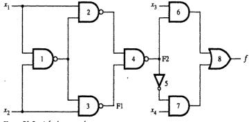
Figure PA.3 A faulty network.
