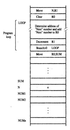
Figure 2.10 Using a loop to add n numbers.
