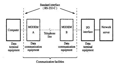
Figure 10.2 Remote connection to a network.
