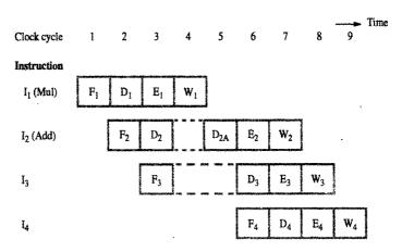
Figure 8.6 Pipeline stalled by data dependency between D<sub>2</sub> and W<sub>1</sub>.
