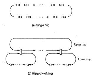
Figure 12.10 A ring-based interconnection network.
