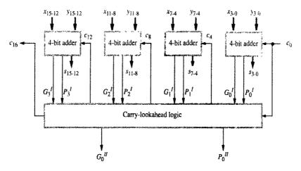
Figure 6.5 16-bit carry-lookahead adder built from 4-bit adders (see Figure 6.4b).
