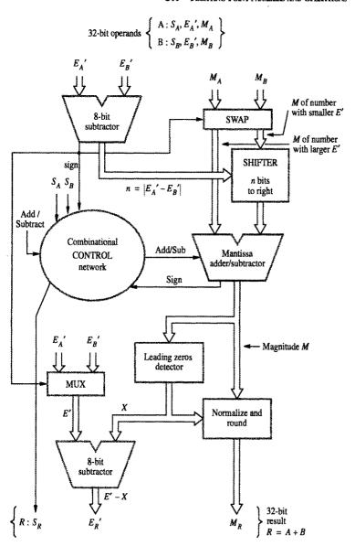
Figure 6.26 Floating-point addition-subtraction unit.
