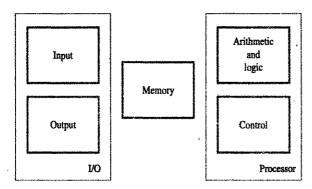
Figure 1.1 Basic functional units of a computer.
