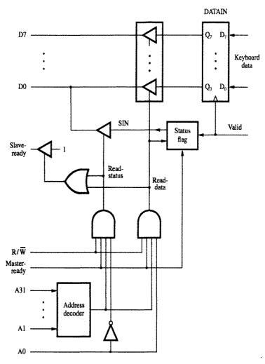
Figure 4.29 Input interface circuit.
