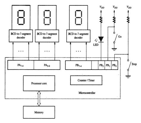
Figure 9.19 The reaction-timer circuit.
