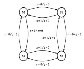
Figure A.47 State diagram of a mod-4 up/down counter that detects the count of 2.
