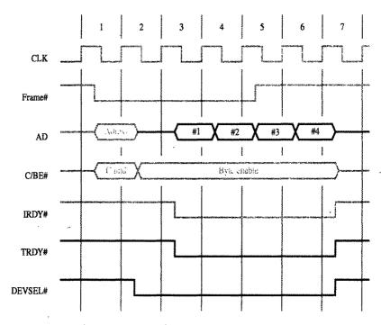
Figure 4.40 A read operation on the PCI bus.
