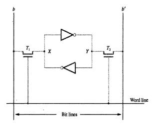
Figure 5.4 A static RAM cell.
