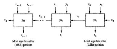
(b) An n-bit ripple-carry adder
