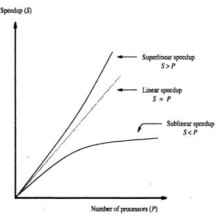
Figure 12.21 Speedup curves in multiprocessor systems.
