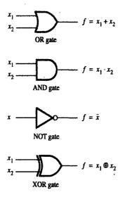
Figure A.2 Standard logic gate symbols.
