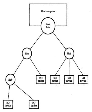
Figure 4.43 Universal Serial Bus tree structure.
