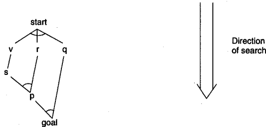
Figure 5.9 Data-driven search in a production system.
