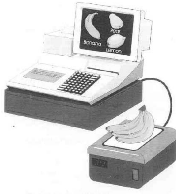
Figure 16.1: Designer's sketch of final supermarket system. (Likely produce items are displayed in case human interaction is needed.) Courtesy of R. Bolle and J. Connell.
