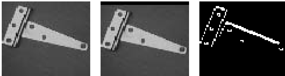
Figure 1.10: Images of a moving part (left and center) and a difference image (right) that captures the boundary of the part.
