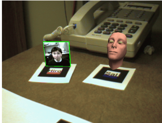
Figure 15.6: An application of augmented reality techniques to teleconferencing (courtesy of the University of Washington HIT Lab).
