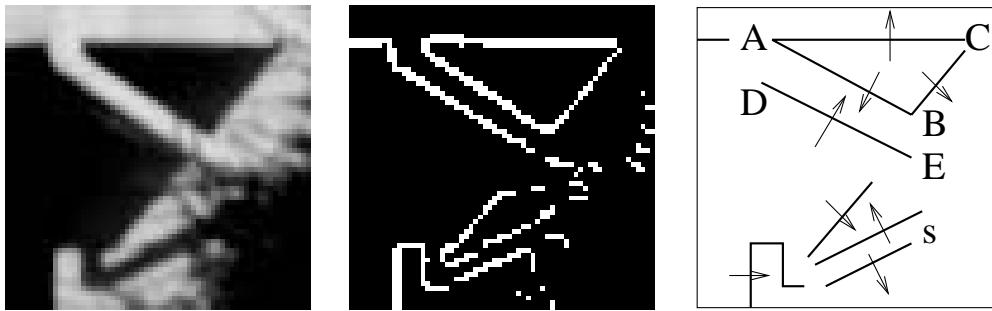
Figure 10.28: (Left) Region of an image of a house showing a downspout and strong shadows; (center) the highest 10% gradient magnitudes computed by the Prewitt 3x3 operator; (right) sketch of ribbons and corners evident.
