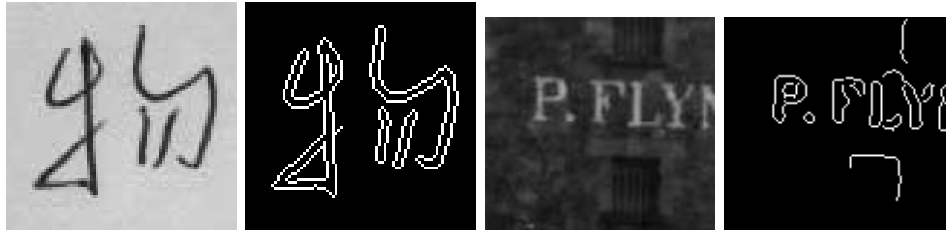
Figure 10.16: Identifying regions corresponding to symbols on surfaces is often easy because they are created with good contrast. These results were obtained by applying only the Canny operator: (left set) character carefully written with ink on paper; (right set) weathered signage on a brick wall.
