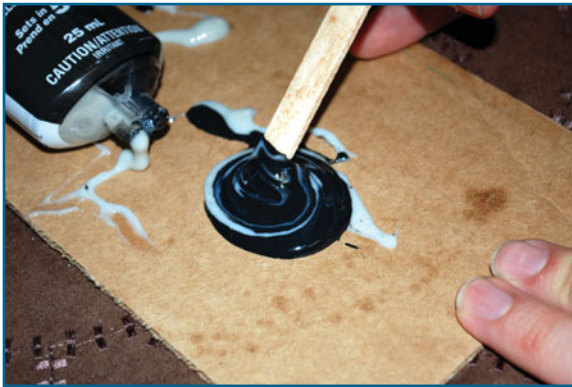
Figure 3.8 Mixing the two-part epoxy glue.
