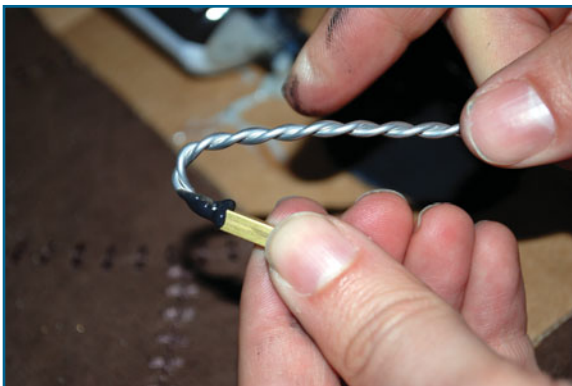
Figure 3.10 Gluing wires into the K&S tubes.
