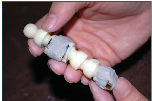
Figure 3.11 Affixing the socket tubes to the armature with epoxy putty.
