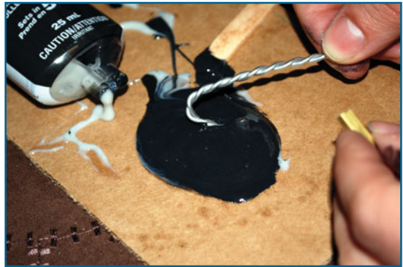
Figure 3.9 Dipping wires into the epoxy glue.
