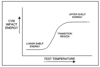
Figure 6-7 Schematic CVN transition curve
