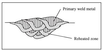
Figure 6-3 Grain refinement in multiple pass weld
