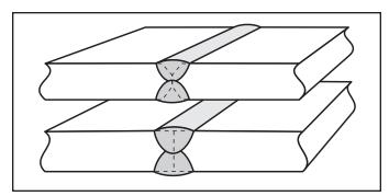
Figure 3-2 Joints requiring substantial penetration
