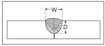
Figure 9-3 Bead shape induced cracking
