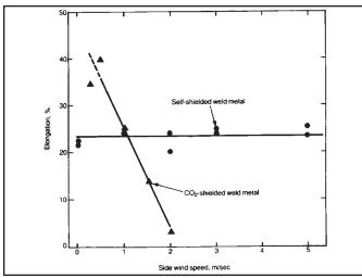
*Figure 3-4a* Comparison of the effect of side wind on tensile elongation of: (a) CO<sub>2</sub>-shielded and (b) self shielded ferritic steel weld metals. (source: Self-Shielded Arc Welding. T. Boniszewski, 1992.)
