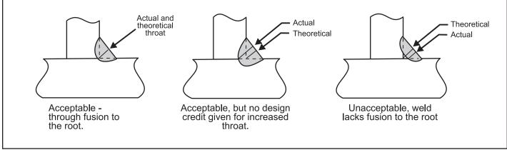
Figure 3-3 Fillet weld requirements
