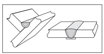
Figure 3-1 Joints requiring substantial fill
