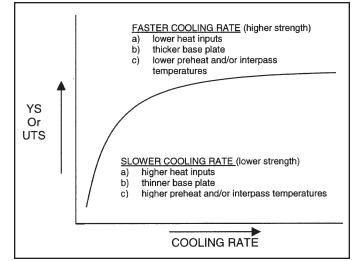
Figure 6-6 Strength related to cooling rate
