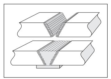
Figure 9-2 Buttering layers
