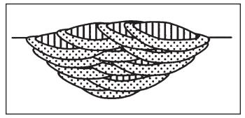
Figure 6-4 Grain refinement for flat weld beads
