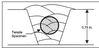
Figure 6-5 Typical tensile specimen location
