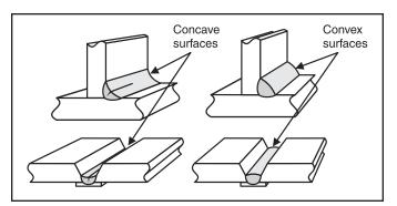
Figure 9-4 Surface profile induced cracking
