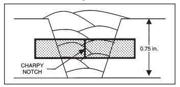
Figure 6-8 Typical CVN specimen location
