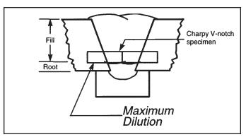
Figure 6-9 Locations of CVN test specimens
