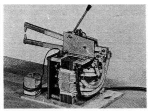
A 6-V. battery provides automatic operation of the relay. Relay also can be operated manually. Drawing below shows the wiring diagram of welding unit
