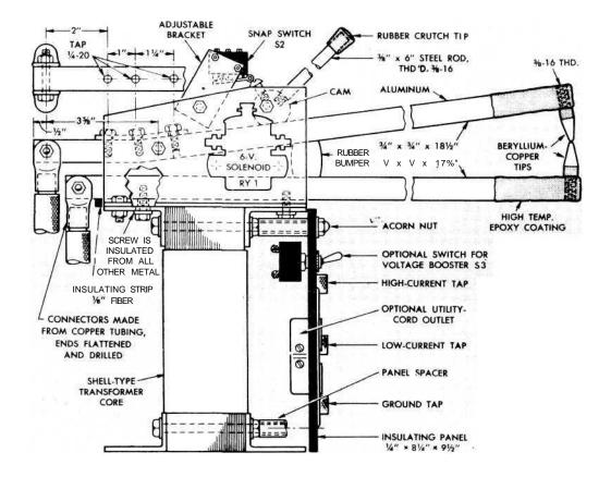
and the cross-sectional area of the main center leg should be at least 6 sq. in. or slightly more. There also should be about 2 in. of space separating the legs so there will be room for the coils.
