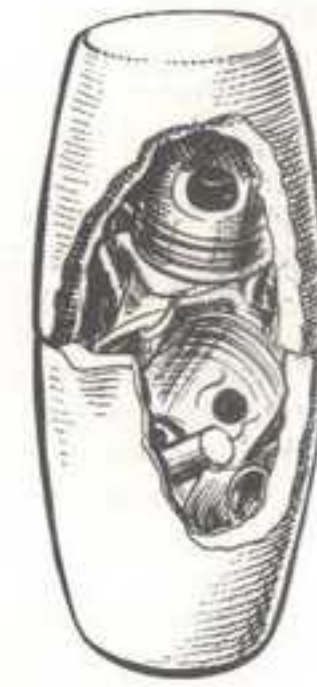
Fig. 4. Enabling a greater bulk of metal to be included in the initial charge.
