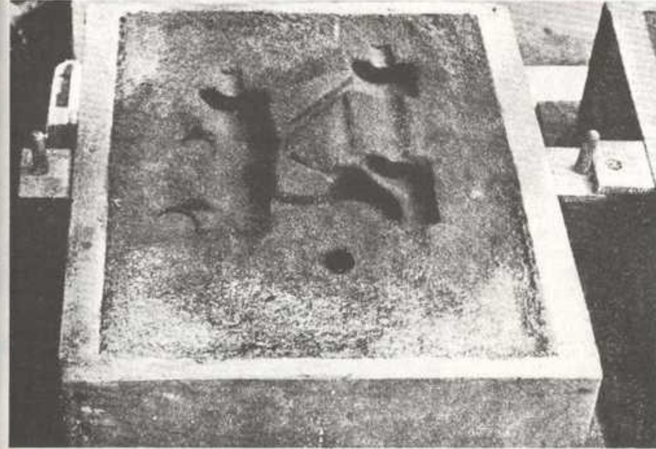
Above, The impression in the drag with cores in position. Below, the impression in the cope.
