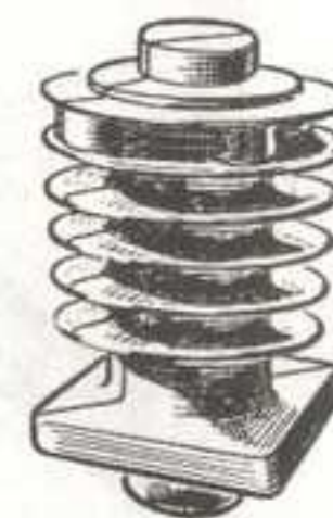
Fig. 77. Pattern of finned cylinder for moulding in oilsand.
