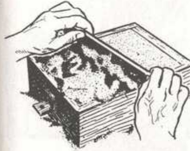
Fig. 59. Strickling away the surplus sand.
