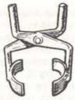
Fig. 83. An ideal type of crucible tongs.
