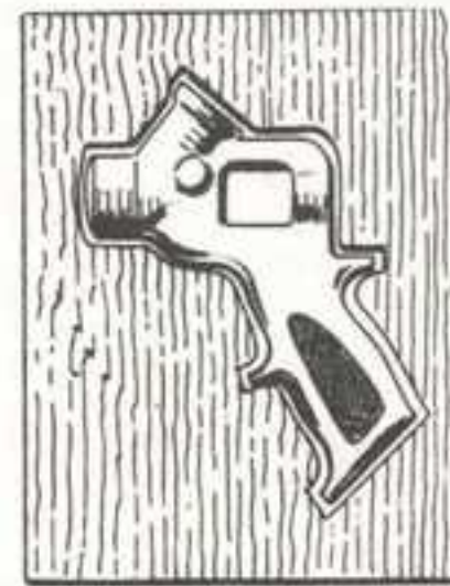
Fig. 41. A template used for moulding pattern.
