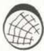
Fig. 44. Building up a section with plastic wood.
