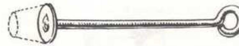
Fig. 91. A "bot" stick with a dotted indication of the shape of the "bot."
