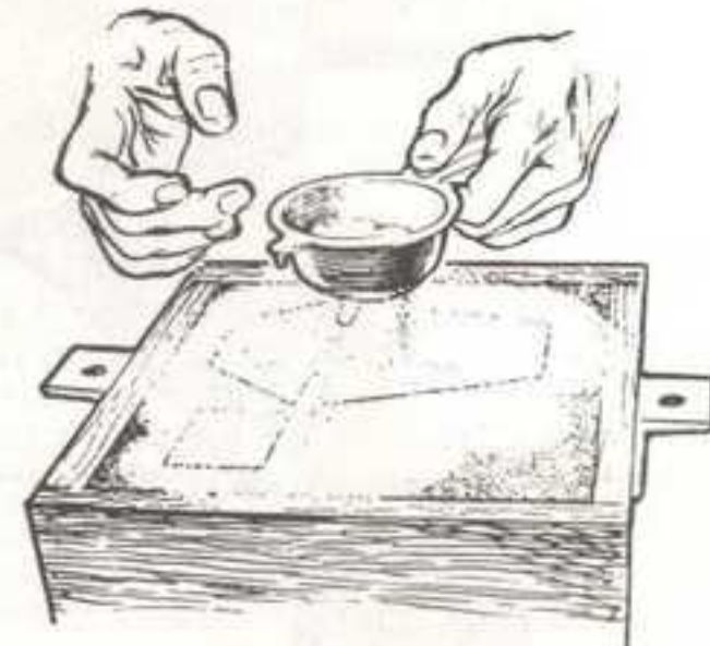
Fig. 61. Dusting with parting powder.
