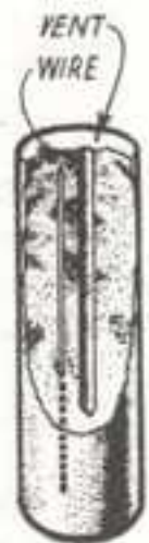
Fig. 46. Showing how a sand core can be vented and also reinforced with wire.
