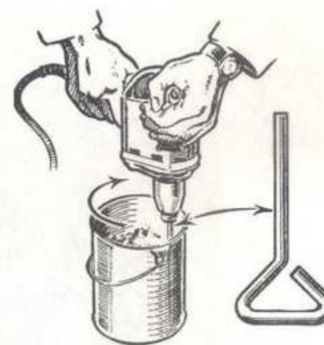
Fig. 14. The use of a portable electric drill for the mixing or "milling" of oil sand.
