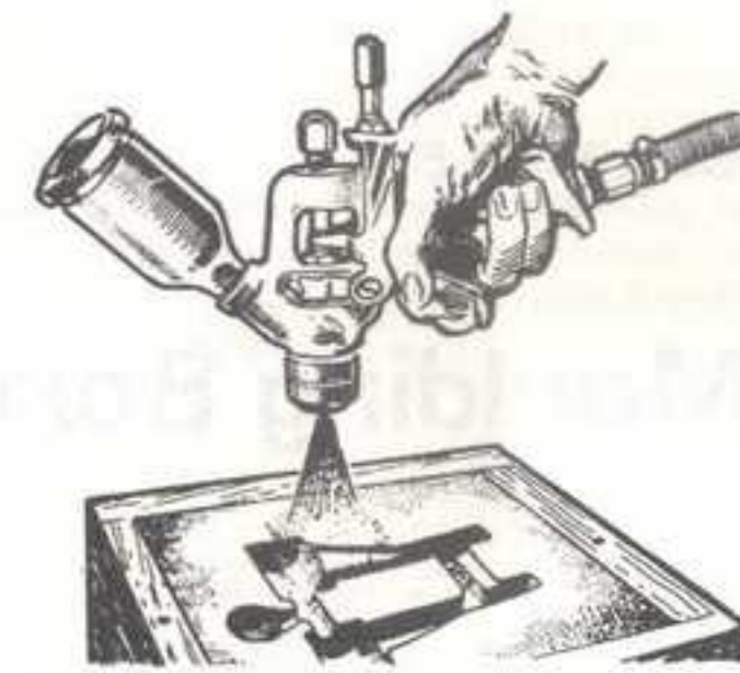
Fig. 15. The use of a spray gun for the application of refractory dressings to the mould.
