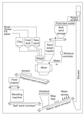
Figure 12.3 Flow diagram for a typical green sand plant. (From Foundryman, March 1998, p. 102. Courtesy Foundry and Technical Liaison Ltd.)
