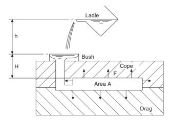
Figure 1.1 Opening forces of moulds.
