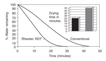
Figure 16.2 Drying comparison, RHEOTEC RDT versus conventional coating.
