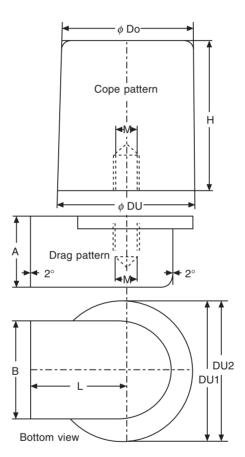
Figure 19.21 Sleeve pattern for a floating sleeve. The cavity created by means of the cope sleeve pattern ensures location of the feeder sleeve while closing the mould.
