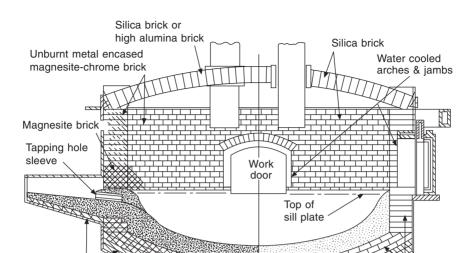
**Figure 10.1** Schematic diagram of an arc furnace showing typical refractories used in acid and basic practices. (From Jackson, W.J. and Hubbard, M.W., Steelmaking for Steelfounders, 1979, SCRATA. Courtesy CDC.)
