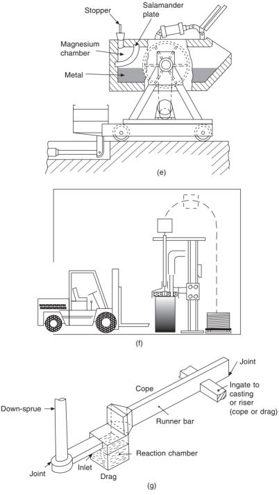
Figure 6.1 Treatment methods for making ductile iron. (a) Sandwich treatment. (b) Pour-over treatment. (c) Tundish cover ladle. (d) Plunging treatment. (e) GF Fischer converter. (f) IMPREX cored-wire treatment station (g) In-mould system.
