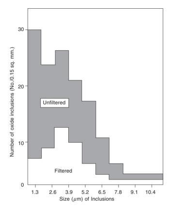
Figure 18.7 Histogram comparing the cleanliness of an unfiltered and filtered Al-killed steel (sulphides not included in total number of inclusions).
