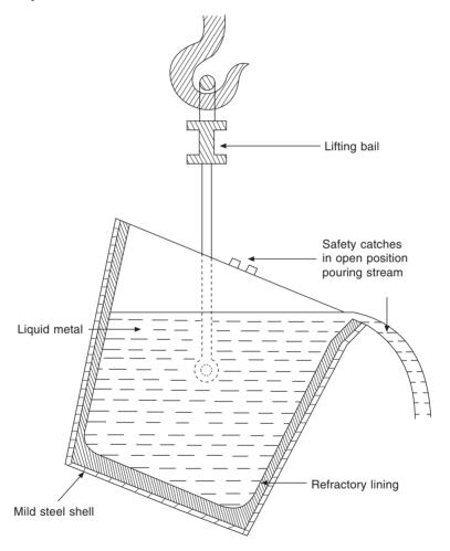
Figure 11.6a Section through a lip pour ladle. (From Jackson, W.J. and Hubbard, M.W., Steelmaking for Steelfounders, 1979, SCRATA. Courtesy CDC.)
