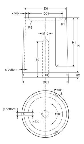
Figure 19.23 Sleeve pattern for shell mould application.
