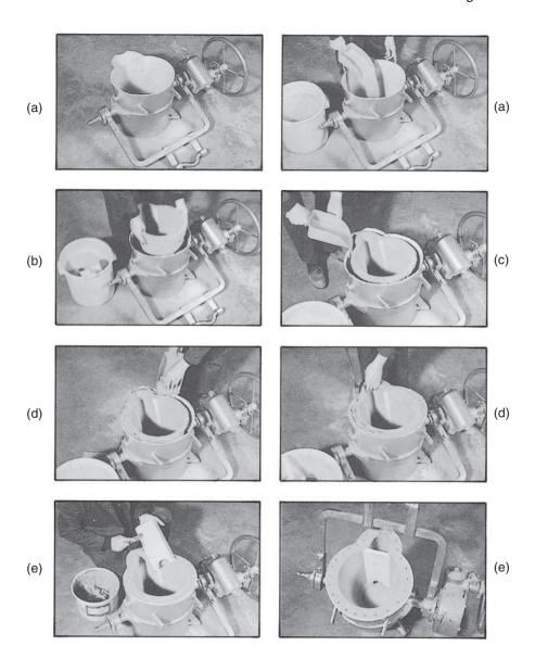
Figure 11.1 Installation of the KALTEK one-piece ladle liner
