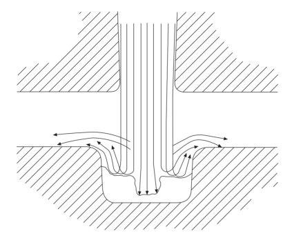
Figure 18.4 Flat bottomed sump located at sprue base minimises turbulent metal flow. (From Blackburn C.S. and Blair B. 35th SCRATA Conference, May 1992, Courtesy CDC.)
