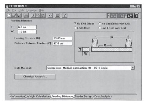
Figure 19.31 FEEDERCALC feeding distance screen.
