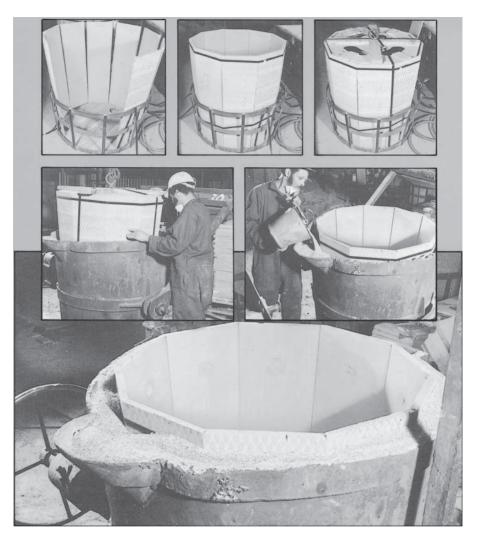
Figure 11.2 Panel ladle made using KALTEK boards.
