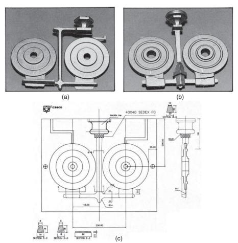
Figure 17.18 Use of a SEDEX filter in vertically parted moulds. (a) unfiltered; (b) filter placed at base of sprue; (c) filter placed in pouring bush.
