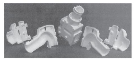
**Figure 15.2** Sections of patterns are glued together to form complex shapes.
