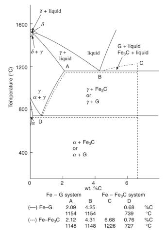
**Figure 2.1** The iron–carbon phase diagram. (From Elliott, R., Cast Iron Technology, 1988, Butterworth-Heinemann, reproduced by permission of the publishers.)
