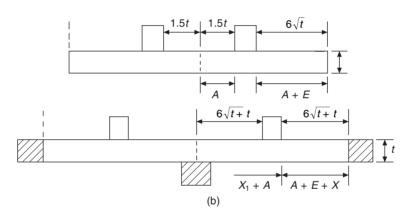
Figure 19.4 Feeding distance in steel castings. (a) Plate (width: thickness >5:1. (b) Bar (width: thickness < 5:1).
