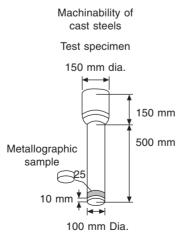
Figure 18.8 Machinability test piece.
