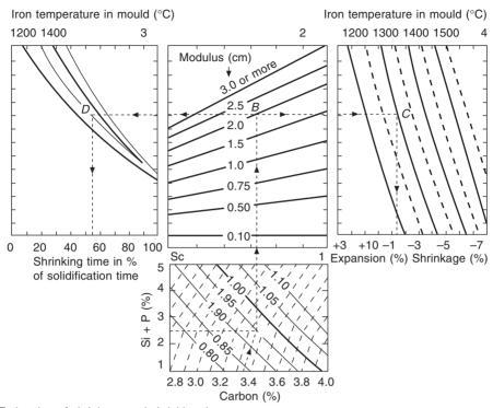
Estimation of shrinkage and shrinking time from Analysis, casting modulus and metal temperature in the mould.
