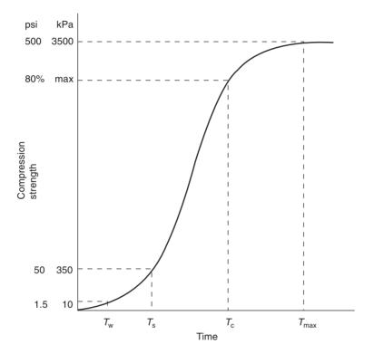
Figure 13.1 Typical hardening curve for self-hardening sand:
