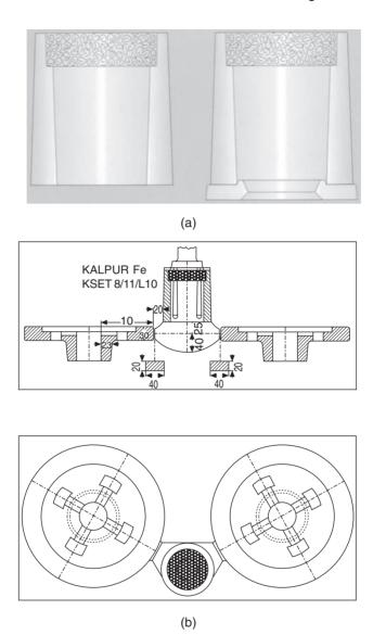
Figure 19.17 (a) KALPUR insert filter feeder units with upper filter location for horizontally parted automatic moulding lines. Without breaker core for direct pouring through a side feeder. With breaker core for direct pouring through a top feeder. (b) KALPUR Fe Insert side feeder used for feeding two ductile iron case covers.
