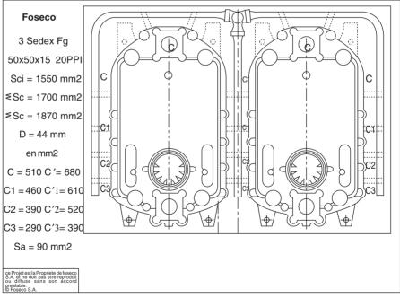
**Figure 17.17** Use of a SEDEX filter with compact running system to cast 2 boiler castings/flask: (a) one casting/flask; (b) two castings/flask.
