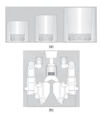
**Figure 19.18** (a) KALPUR pouring cup filter-feeder units with lower filter position for vertically parted moulding lines. (b) KALPUR pouring technique used on a DISAMATIC moulding line for casting ductile iron hydraulic arms.
