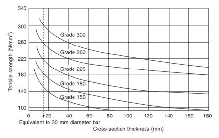
**Figure 3.1** Variation of tensile strength with section thickness for several grades of iron. (Data supplied by CDC.)
