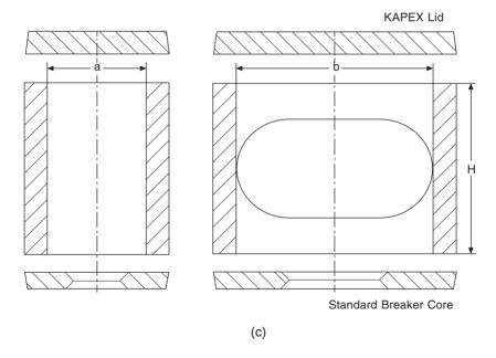
Figure 19.14 (a) KALMINEX cylindrical feeder sleeve with breaker core and KAPEX lid. (b) KALMINEX TA sleeve. (c) KALMINEX oval sleeve.
