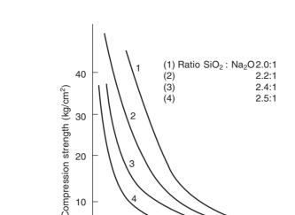
The effect of 24 hour storage of cores gassed for different times as a function of silicate ratio.
