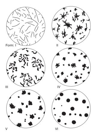
Figure 3.4 (a) Reference diagrams for the graphite form (Distribution A). The diagrams show only the outlines and not the structure of the graphite.
