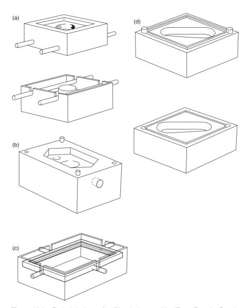
Figure 13.2 Typical designs of self-hardening moulds. (From Foundry Practice Today and Tomorrow, SCRATA Conference, 1975.) (a) Method of moulding-in steel tubes for ease of handling boxless moulds. (b) Sockets moulded into boxless moulds for ease of lifting, roll-over and closing. (c) Steel reinforcement frames for handling large boxless moulds. (d) Method of locating mould halves and preventing runout.
