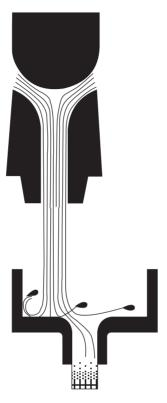
Figure 18.3 Simulation showing the elimination of metal splashing due to optimisation of pouring cup design.
