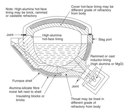
**Figure 4.4** A bath channel induction fumace, showing typical lining arrangement. (Reproduced by courtesy of CDC.)
