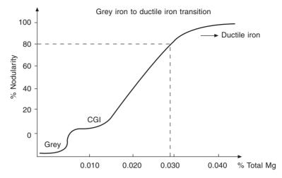
Figure 6.5 The effect of total Mg content on the transformation of graphite morphology from flake to compacted and ultimately to spheroidal graphite. (Courtesy SinterCast.)
