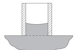
**Figure 19.2** Ideal feeder solidification pattern where all the heat from the feeder has been lost to the casting (schematic).
