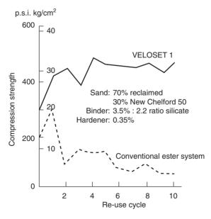
**Figure 14.5** *VELOSET reclamation, ultimate strength characteristics of reclaimed sand, compared with conventional ester process.*
