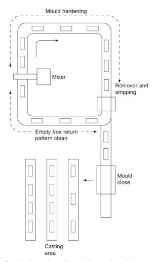
Figure 13.3 Foundry layout for self-hardening sand moulds.
