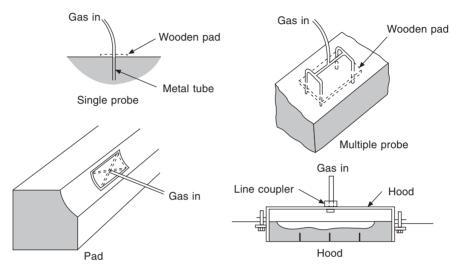
**Figure 14.2**  $CO_2$ -silicate process, methods of gas application.
