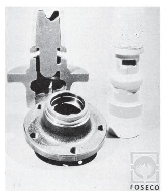
Figure 19.25 A ductile iron hub casting using a sleeve located in the central core. The sleeve is placed into the core print location and fits into the cope mould cavity created by the appropriate sleeve pattern.
