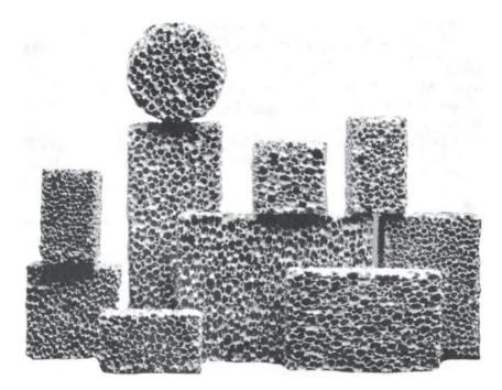
Figure 17.5 Ceramic foam filters.
