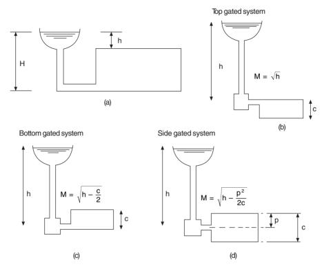
Figure 17.4 (a) The head of metal varies from H at the start of pour to h at the end. M is: (b)  $\sqrt{h}$  for a top gated system; (c)  $\sqrt{h-c/2}$  for a bottom gated system; (d)  $\sqrt{(h - p^2/2c)}$  for a side gated system.
