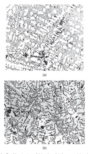
Figure 5.1 Graphite structure of (a) uninoculated grey cast iron (×100) and (b) inoculated grey cast iron (×100). (From BCIRA Broadsheet 161-4; reproduced by courtesy of CDC.)
