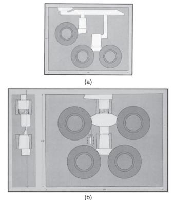
**Figure 17.25** Use of the KALPUR unit in vertically parted automatic moulding lines: (a) conventional layout; (b) using KALPUR.
