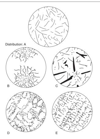
**Figure 3.4 (b)** Reference diagrams for the distribution of graphite (Form 1). The diagrams show only the outlines and not the structure of the graphite.
