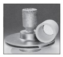
Figure 18.14 KALPUR unit used as a central feeder.
