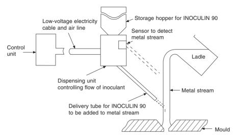
Figure 5.3 The principles involved in the MSI System 90.
