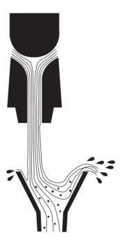
**Figure 18.2** Simulation of metal splashing due to incorrect alignment of nozzle and pouring cup.
