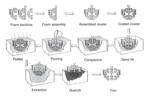
Figure 15.1 The lost foam casting process.
