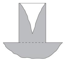
Figure 19.1 Solidification pattern of a feeder for a steel casting (schematic).
