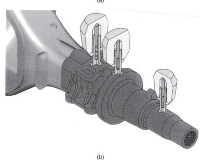
Figure 19.13 (a) The application of FEEDEX HD V-Sleeves to a ductile iron turbocharger casting. (b) VS-Spot feeder practice. The point feeding technique makes possible the production of high value, lightweight castings.
