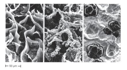
The transition of graphite morphology from flake to compacted to spheroidal shown by deep etched scanning electron micrographs. (Courtesy SinterCast.)
