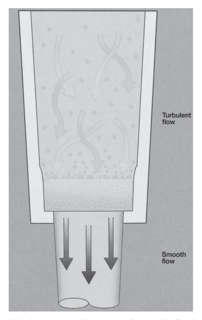
Figure 17.19 A schematic view of the cleaning and flow-smoothing effect of pouring directly through a KALPUR unit.
