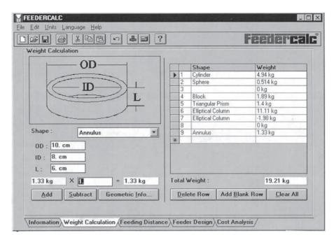
Figure 19.30 FEEDERCALC weight calculation screen.
