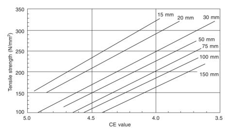
Relationship between tensile strength and carbon equivalent value for various bar diameters. (Data supplied by CDC.)
