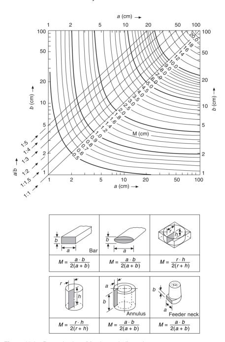
Figure 19.6 Determination of feeder neck dimensions.
