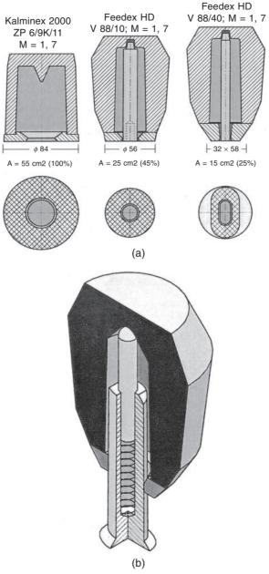
Figure 19.12 (a) The reduction of the feeder contact area which is possible when using the FEEDEX HD V-Sleeve with a suitable breaker core. (b) Sectioned spring loaded steel location pin for ram-up of a V-sleeve without a breaker core.
