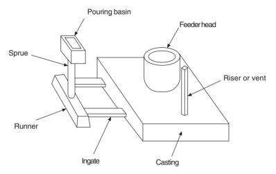
Figure 17.1 The basic components of a running system.
