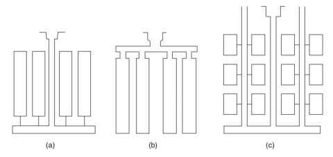
**Figure 17.3** Examples of vertically parted moulding systems: (a) A sprue/runner controlled system. (b) A runner/gate controlled system. (c) A multilevel system. (from Elliott, R., Cast Iron Technology, 1988, Butterworth-Heinemann, reproduced by permission of the publishers.)
