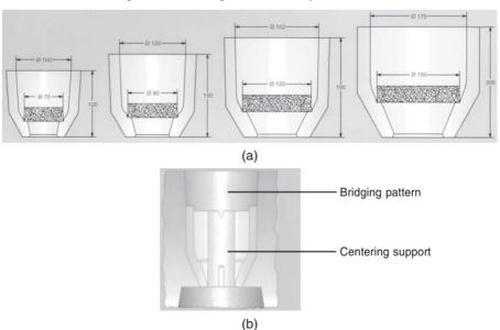
**Figure 19.19** (a) KALPUR ram-up filter feeder series for jobbing and simple moulding machine applications. (b) Ram-up principle with fixed centering support and a loose 'bridging' pattern to give the correct height.
