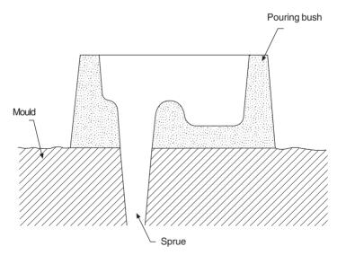
Figure 17.2 A properly designed pouring bush.
