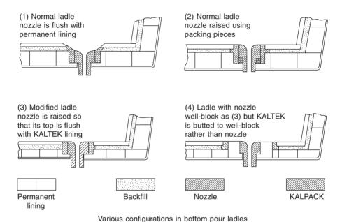
Figure 11.7 Methods of installing nozzles in bottom pour ladles.
