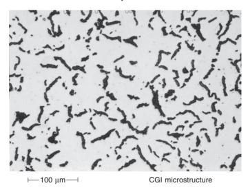
Figure 6.4 Structure of compacted graphite. (Courtesy SinterCast.)
