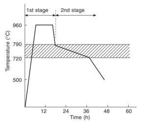
**Figure 7.1** Typical heat treatment cycle for a short cycle blackheart malleable iron. (From Elliott, R. (1988) Cast Iron Technology, Butterworth-Heinemann, reproduced by permission of the publisher.)
