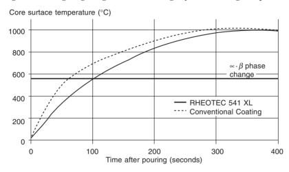
Figure 16.1 Illustration of the superior insulating behaviour of RHEOTEC XL coatings.
