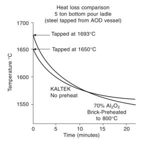
Figure 11.8 Heat loss comparison, 5 ton bottom pour ladle, KALTEK v. brick-lined.
