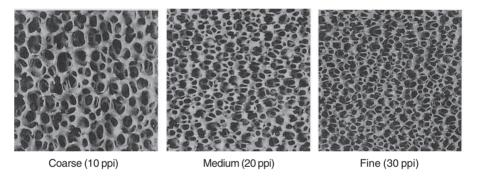
Figure 17.8 SEDEX filters of differing porosity.
