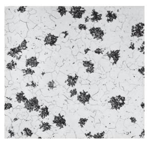
Figure 2.3 Malleable cast iron, 4% picral, ×100. (From BCIRA Broadsheet 138, reproduced by courtesy of CDC.)
