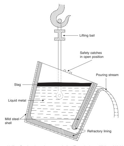
**Figure 11.6b** Section through a teapot ladle. (From Jackson, W.J. and Hubbard, M.W., Steelmaking for Steelfounders, 1979, SCRATA. Courtesy CDC.)
