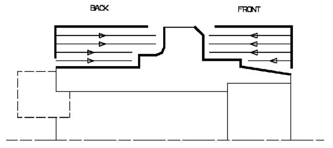
Orientation and Location settings determine the way the program closes the area to machine using radial, axial, axial-radial or radial-axial relimitation.
