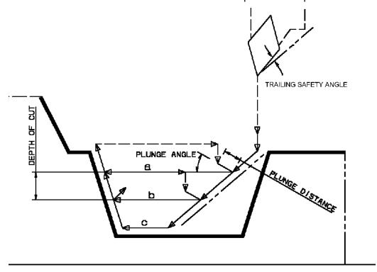
Example of one-way recessing. Note that Trailing angle is defined on the tool.
