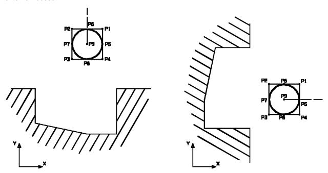
The tool output point is dependent on the machine axis system.
