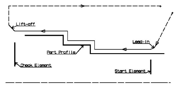
Use of start and end elements for profile finishing. Profile is machined from start element. Profile is extrapolated up to end element. Direct approach and radial-axial retract.
