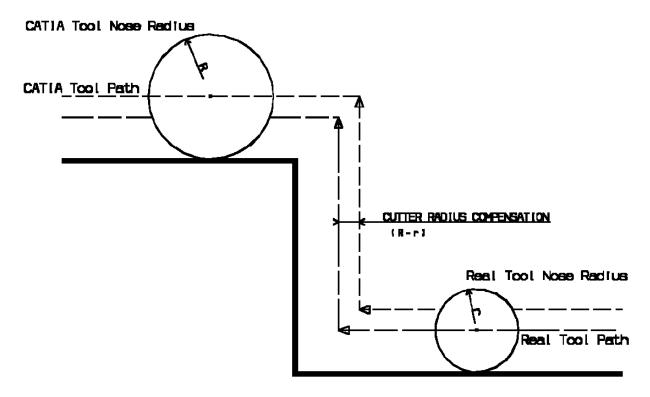
Cutter compensation for profile finishing
