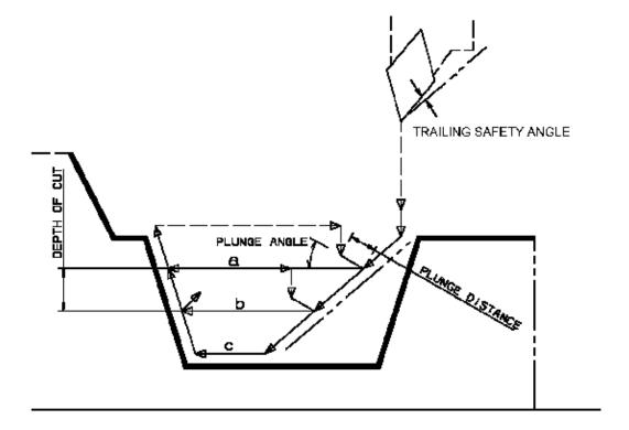
Example of recess with longitudinal external roughing. Note that Trailing angle is defined on the tool.
