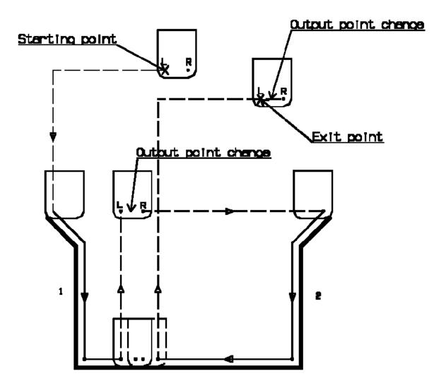
If the first flank to machine is flank 1, the tool motion is as follows:
