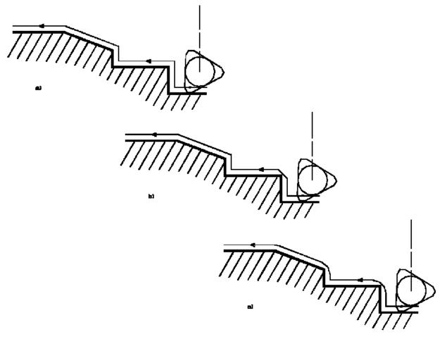
Corner processing options are also available to define how the entry and exit corners are to be machined. Entry and exit corners are defined by either a chamfer length, or a corner radius and corner angle.
