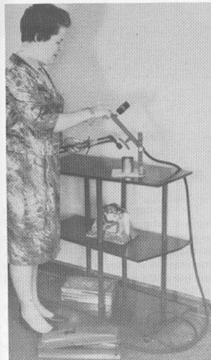
The pressure casting machine with a foot pump, set up to simulate the casting procedure.
