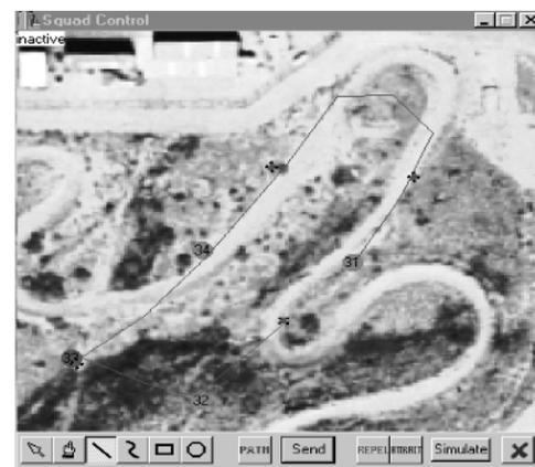
FIGURE 4-5 User interface for perimeter surveillance. The perimeter is marked in blue and miniature intrusion detection sensors are marked by circular numbered icons. An alarm is identified when the icon turns red. The vehicles closest to the intrusion attend to the alarm, while the others adjust their position around the perimeter to prepare for other possible alarms. SOURCE: Feddema et al. (2002). © 2002 IEEE.
