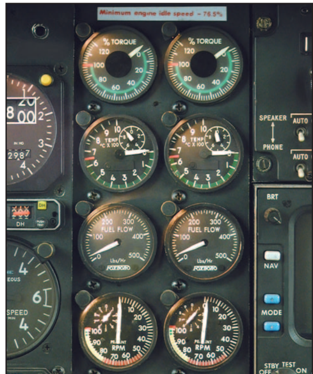
Figure 14-4. Powerplant instrumentation—fixed shaft turboprop engine.
