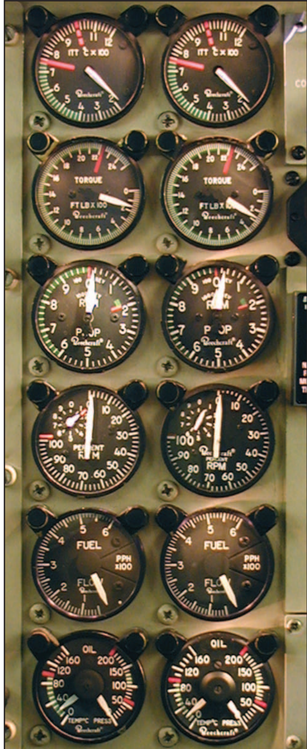
Figure 14-7. Engine instruments—split shaft/free turbine engine.
