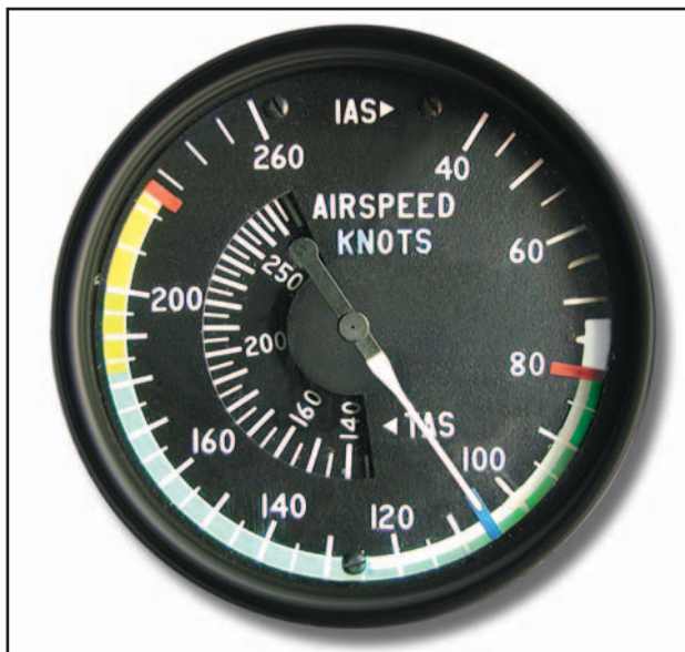
Figure 12-1. Airspeed indicator markings for a multiengine airplane.
