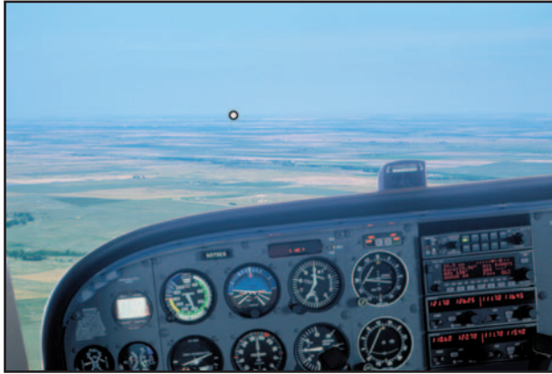
Figure 3-11. Visual reference for angle of bank.
