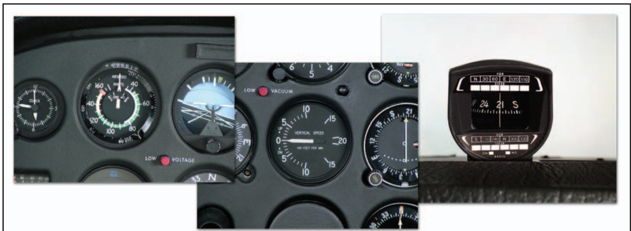
Figure 2-5. Airspeed indicator, VSI, and magnetic compass.
