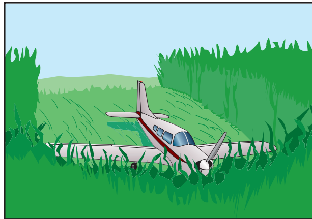
Figure 16-1. Using vegetation to absorb energy.
