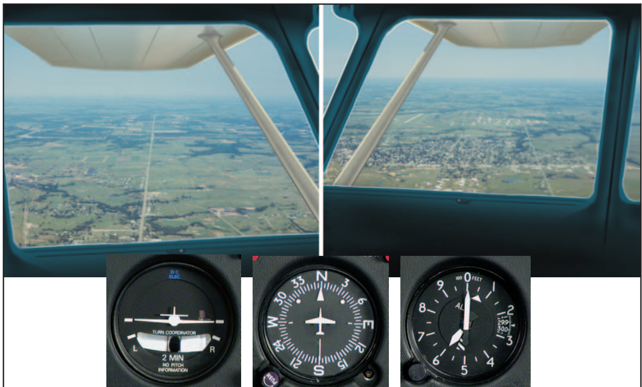
Figure 3-4. Wingtip reference for straight-and-level flight.
