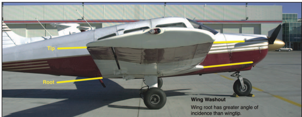
Figure 4-4. Wingtip washout.
