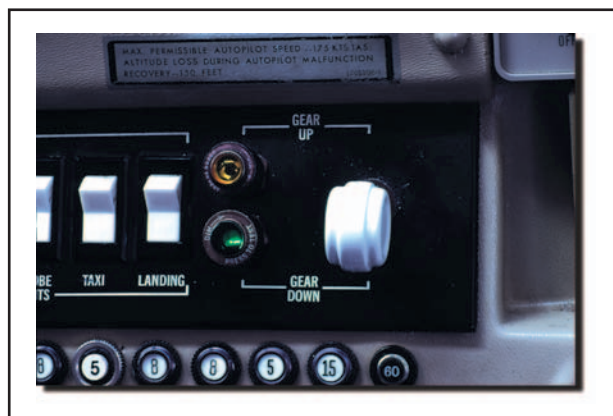
Figure 11-7. Typical landing gear switches and position indicators.
