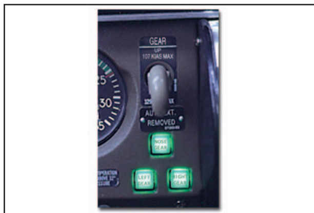
Figure 11-6. Typical landing gear switches and position indicators.
