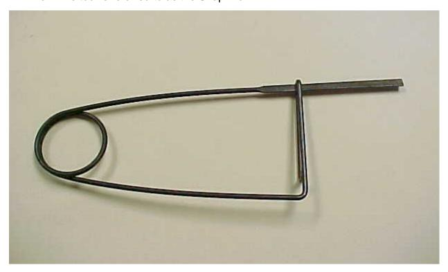
The tip of the tool has been flattened to allow the blade to be manageable inside the keyway.
