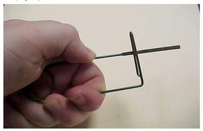
Once the coil has been compressed by pressing down on the wire, the wire is released. This action will snap the pins upward within the keyway simulating the action of a mechanical pick gun.
