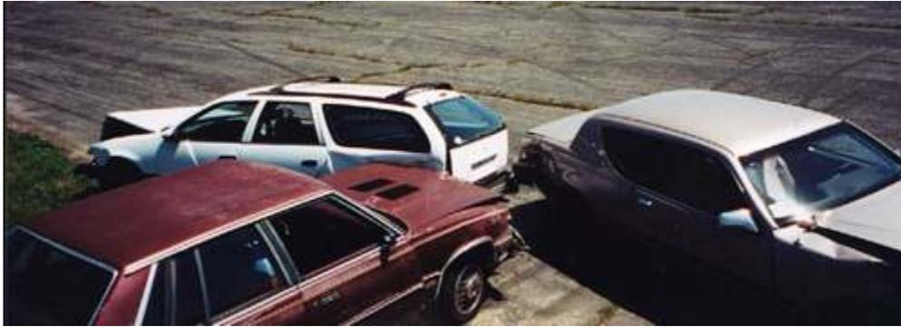
Vehicle placement is critical. You will need to place the frame of your car, the most solid part, directly into the axle of the barricade vehicle. You will begin to move the barricade since your car is able to build enough force to push the barricade cars out of the way. What is actually happening is that the amount of force that your car has generated is being applied to the only part of the barricade vehicle that is connected to the ground (tires).
