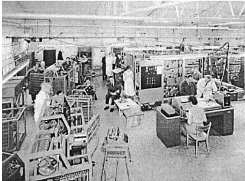
Figure 1 Assembly of Z22 in the Zuse KG factory in Bad Hersfeld (Germany)
