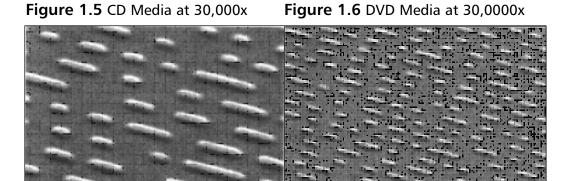
Note that the spacing of the pits and lands does not change across the radius of the disc. This means there is more information stored at the outer edge than there is at the inner edge. The track pitch is the distance between the "wraps" of the spiral. CDs can have a track pitch from 1,500 to 1,700 nm, or about two wavelengths.
