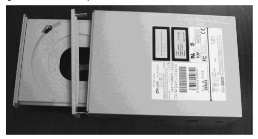
Figure A.2 Drive with Tray Out and Front Removed
