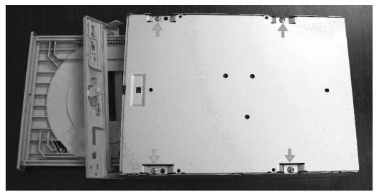
The next step is to turn the drive upside down and carefully remove the four screws that hold the outer casing on; put them with the front cover. These should be saved if you want to put the drive back together. Pull the top cover off of the drive very carefully. Do not bend the cover, which can damage the drive. Prying around the base of the drive with the straight-blade screwdriver can help.
