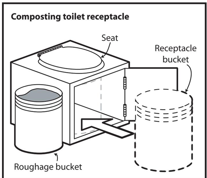
After each "deposit", add roughage to cover the feces and urine. This toilet does not require an airtight or fly-proof lid, since the roughage keeps out flies and cuts smells.
