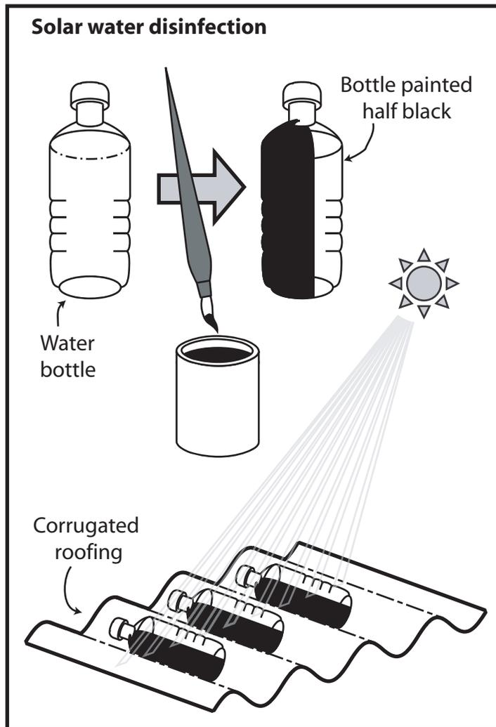
hour in the middle latitudes, it is safe. Placing the bottles on corrugated metal roofing will keep them in place and help to increase the temperature.
