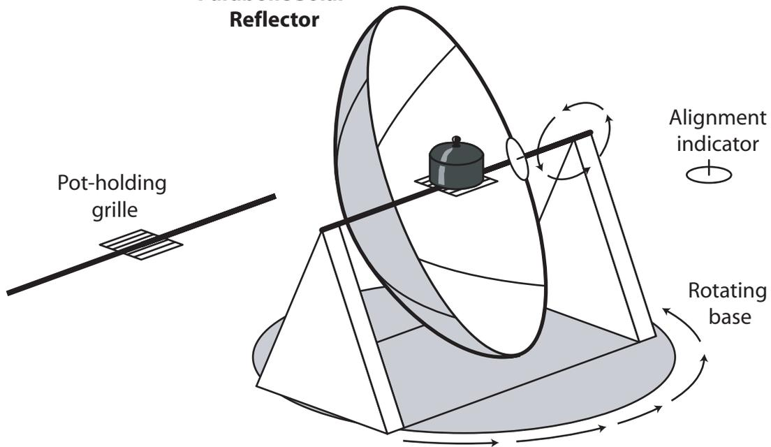
cator (which can be as simple as the circle with a post shown) will help you to line up your parabolic cooker with the sun. Just mount the post at  $90^\circ$  to the cooker. When the post casts no shadow, the collector is properly aligned.
