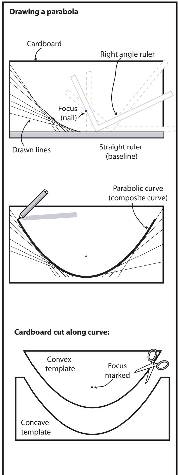
**Turning a parabola in clay to make a mold for reflectors**
