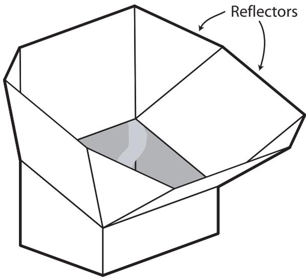
to access the food. You can use plywood for the main structure of the box, or any other improvised material.
