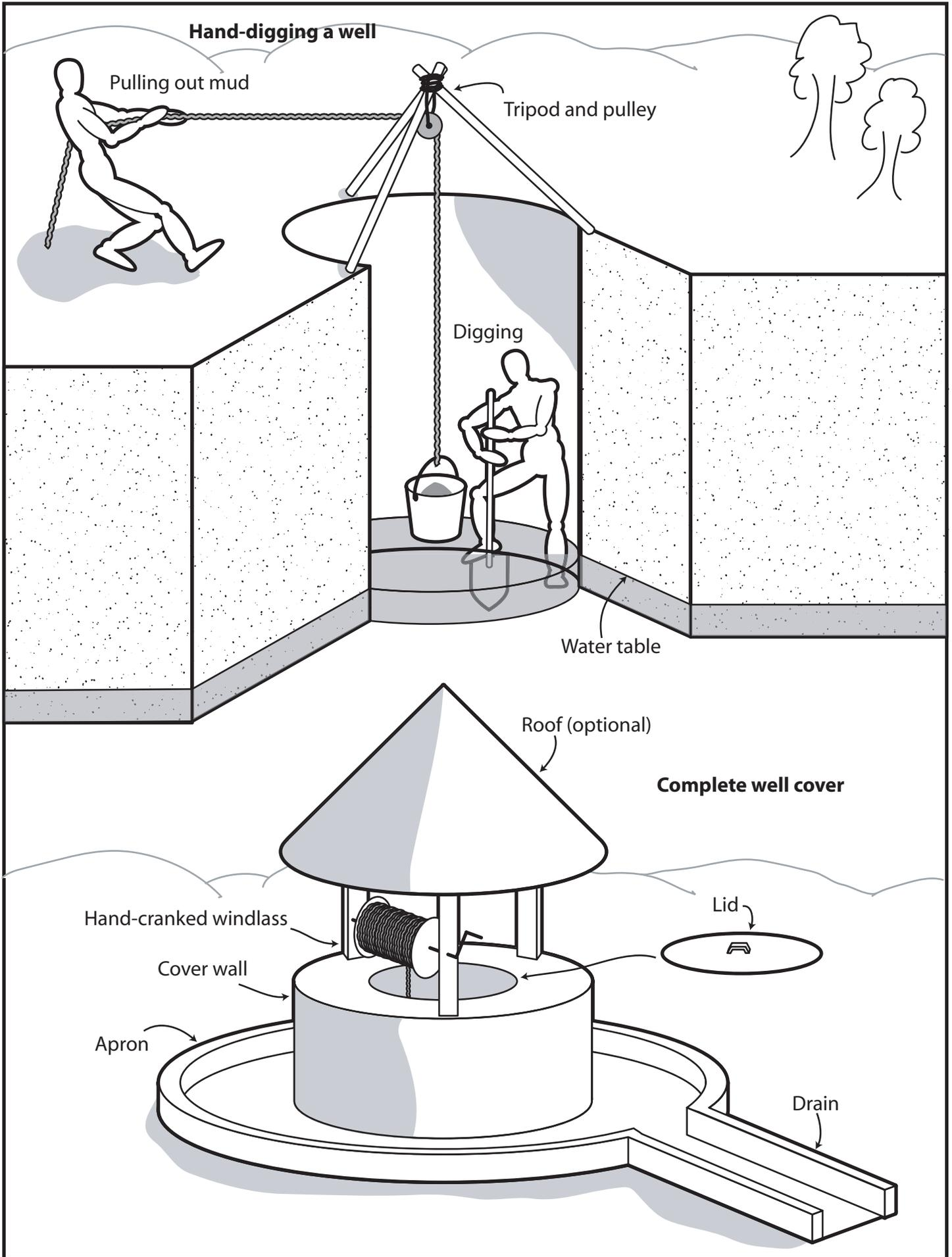
When finished, place a layer of gravel at the bottom of the well, if possible. It is generally suggested that you disinfect a well before using, or after possible contamination, with a chlorine solution (which you can make from bleach).
