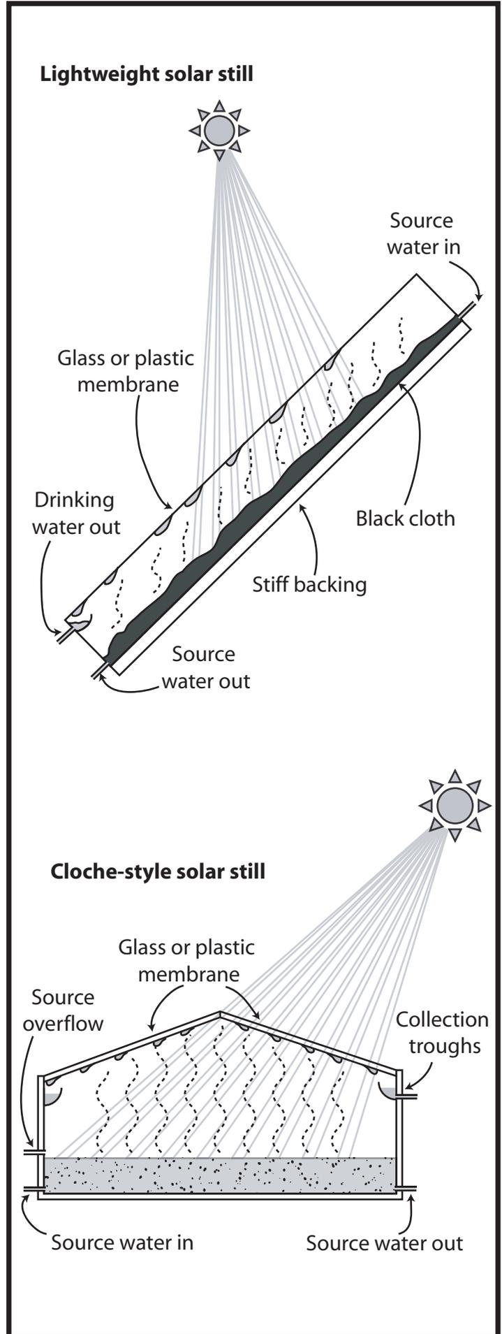
will heat up as much as possible in the sun. You may want to insulate underneath the source container if you are going to place the still on the ground. Then place a shallow trough along the lower edge to capture the condensed droplets as they slide down the glass.
