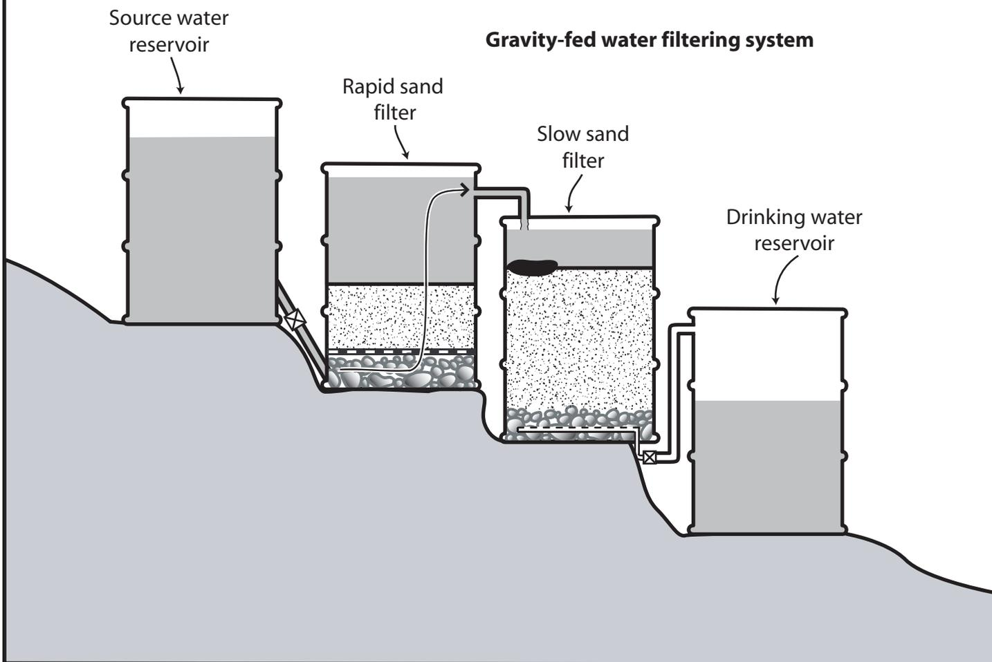
captures and “eats” organisms in the water. The schmutzdecke takes about one to two weeks to form, and so water coming from the filter before that should not be used for drinking.
