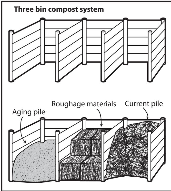
When starting a new humanure compost pile, put down at least 18 inches of roughage. This “sponge” will soak up any fluid leaching from the pile to prevent contamination.
