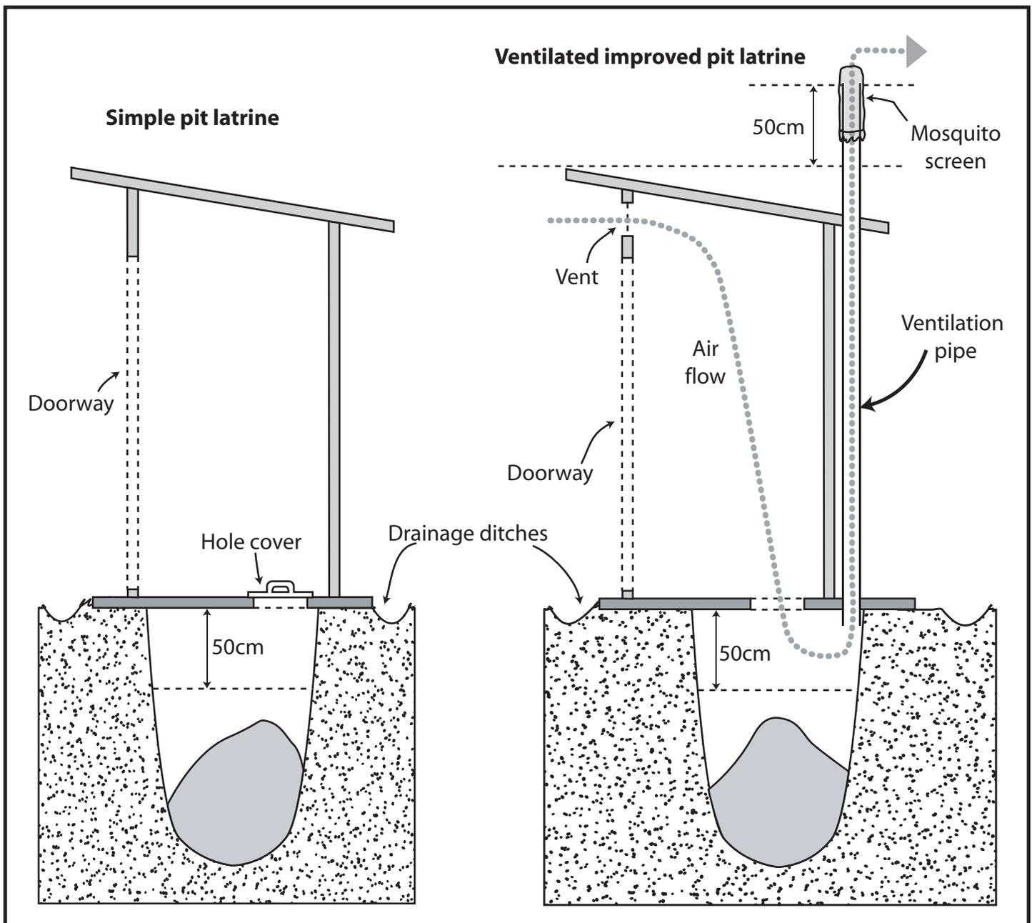
The pit/trench and VIP latrines can be constructed quickly and easily. They are relatively safe, provided that they are not close to a food or water source. Sanitation is aided by the fact that no one has to handle the feces and urine, the hole is simply refilled.
