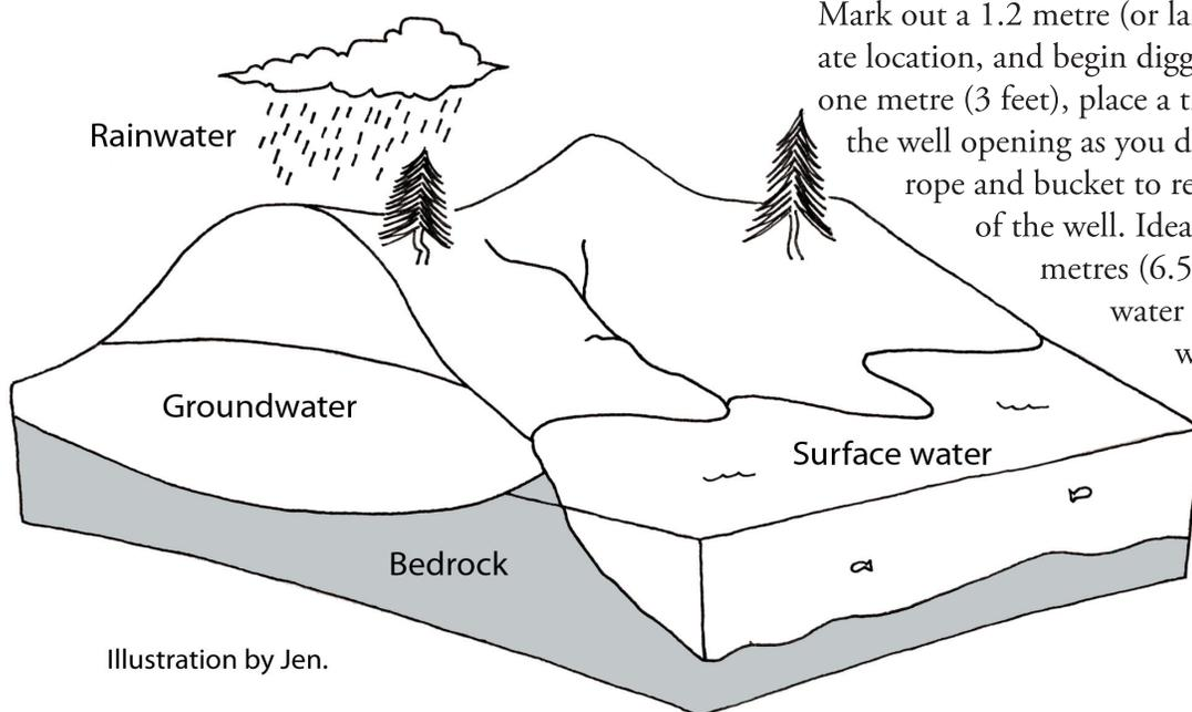
You can also place a well near a river (but at least 15 m away) which will be “recharged” by the river water. However, you should never place a well where it may be flooded by surface water, which could cause contamination.
