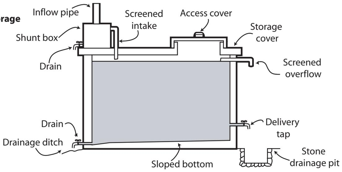
Single Tank Storage design based on a version from the *Sourcebook of Alternative Technologies for Freshwater Augmentation in Small Island Developing States*
