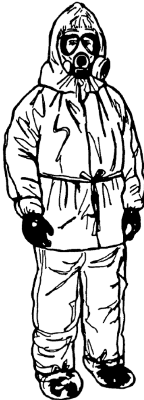
Figure 1-3. Contamination avoidance and liquid protective suit.
