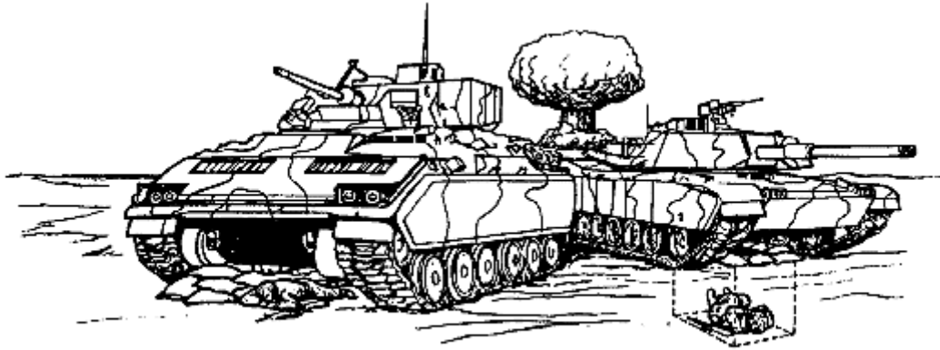
Figure 4-4. Tracked vehicle as expedient overhead cover.
