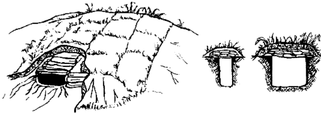
Figure 4-6. Sandbags protected with sod and earth cover.
