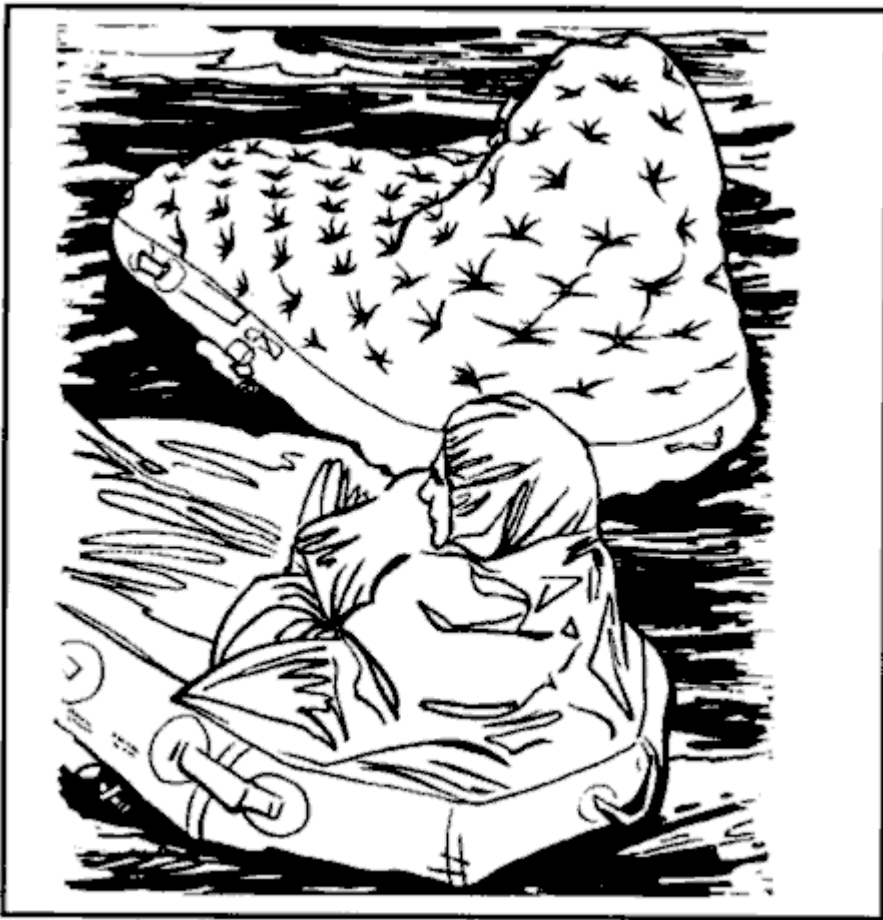
Figure 16-11. One-man raft with spray shield inflated.
