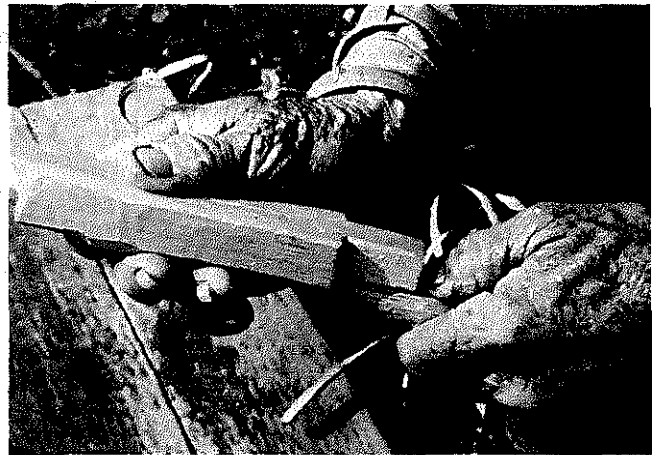
PLATE 193 . . . shows how far into the leg a round will sink, . . .
