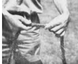
Spinner-feeder on right with bundle of material under his right arm feeds in material.
