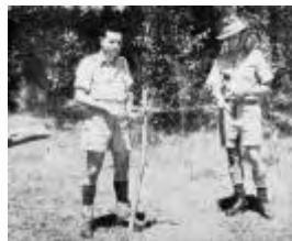
Spinner-feeder on right with bundle of material under his right arm feeds in material.
