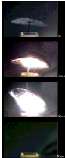
Fig. 1. Carbon sail lifting off of rectangular waveguide under 10 \text{ kW} microwave power at 2 gees (four frames, first at top) in vacuum chamber [5]. Sail heats up, lifts off, and in the bottom frame the sail has flown away.
