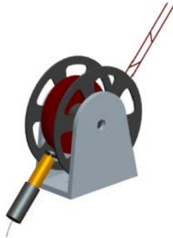
Figure 20: Schematic representation of the tether release mechanism with tether, reel and stepper motor.
