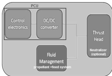
**Figure 1 Subsystems of an EP thruster.**
