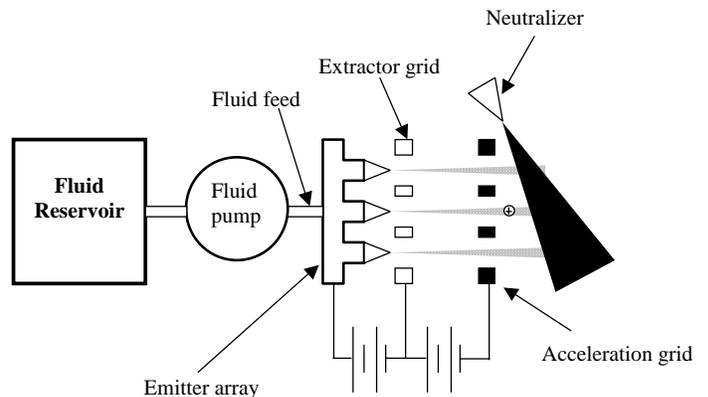
**Figure 6** Typical colloid thruster configuration.
