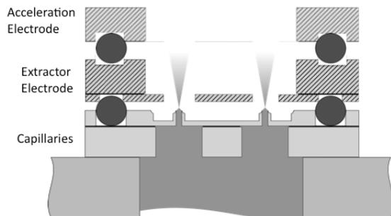
Figure 9 The highly integrated thruster design.
