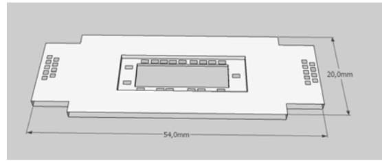
**Figure 11 Multilayer hybrid interface chip made in LTCC for mounting and connecting to the thruster cluster.**
