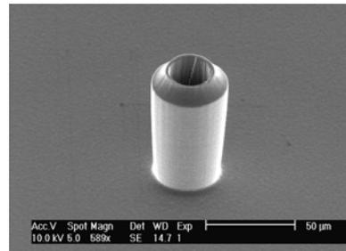
Figure 8 One single emitter, showing shape optimized to minimize liquid spillage. [12]
