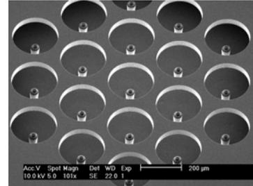
Figure 7 Thruster head design (EPFL), with each capillary centered under one extractor electrode. [12]
