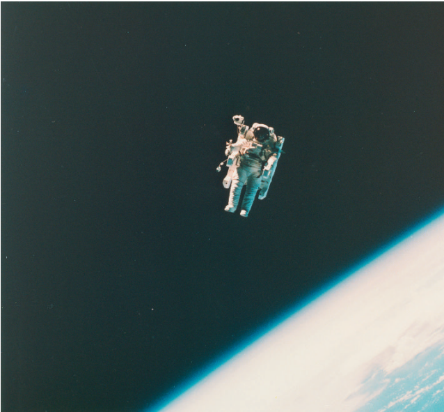
Fig. 7.8 Unprotected from space weather. The first untethered walk in space, on 7 February 1984, where there is no place to hide from Sun-driven storms. Astronaut Bruce McCandless II, a mission specialist, wears a 300-pound (136 kg) Manned Maneuvering Unit (MMU) with 24 nitrogen gas thrusters and a 35 mm camera. The MMU permits motion in space where the sensation of gravity has vanished, but it does not protect the astronaut from solar flares or coronal mass ejections. High-energy particles resulting from these explosions on the Sun could injure or even kill the unprotected astronaut. (Courtesy of NASA.)
