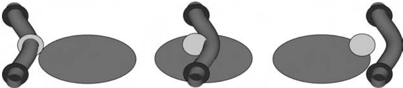
Fig. 2.12. Example of a flux tube crossing a nonideal region (gray) where the transport velocity of the magnetic flux \mathbf{w} differs from the plasma velocity \mathbf{v} while outside the nonideal region the plasma is ideal ( \mathbf{v} = \mathbf{w} ). The black and gray cross-sections are moving with the plasma velocity. The black cross-sections always remain in the ideal domain while the gray cross-section passes the nonideal region and is therefore later detached from the flux tube.
