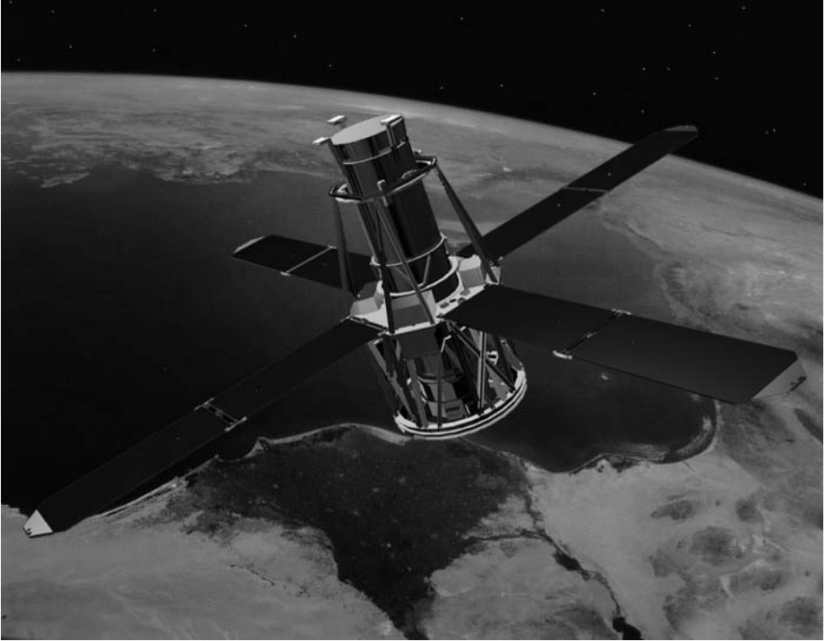
Figure 1.7: The Ramaty High Energy Solar Spectroscopic Imager (RHESSI) is a spinning spacecraft that contains a single instrument, a rotation-modulated collimator with 9 germanium-cooled detectors (courtesy of RHESSI Team).
