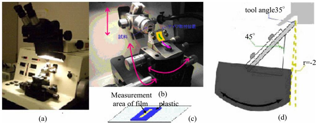
**Figure 2.** Preparation of sample. (a) picture of ultramicrotomes (b) the schematic of cutting process (c) sample schematic (d) knife and sample
