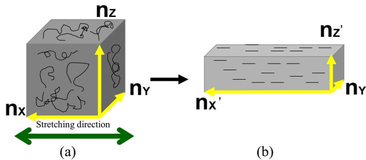
Figure 8. Schematic image of generation of birefringence.
