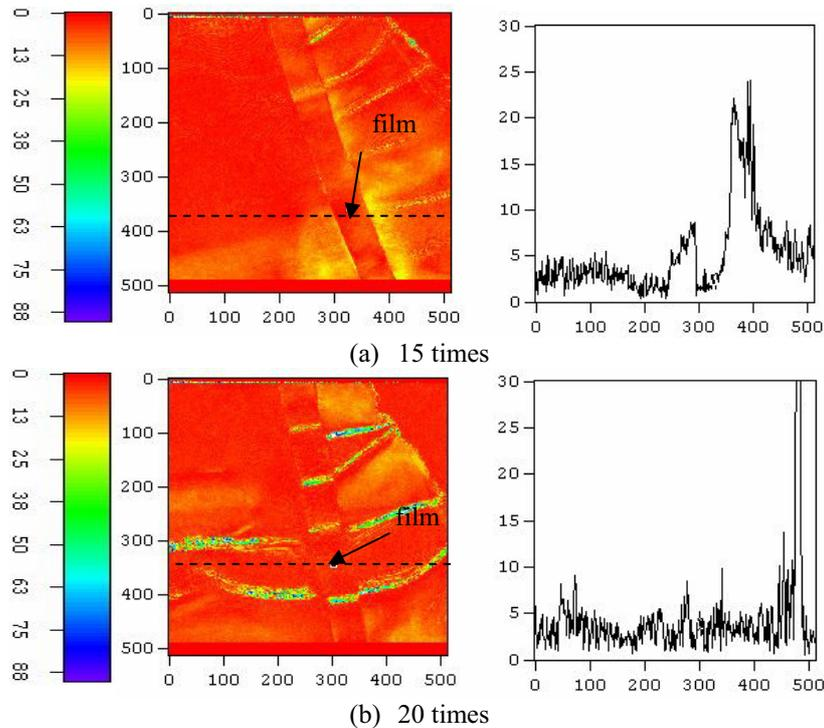
**Figure 3.** The effect brought in by cutting repeat count. (a) cutting 15 times and (b) cutting 20 times.
