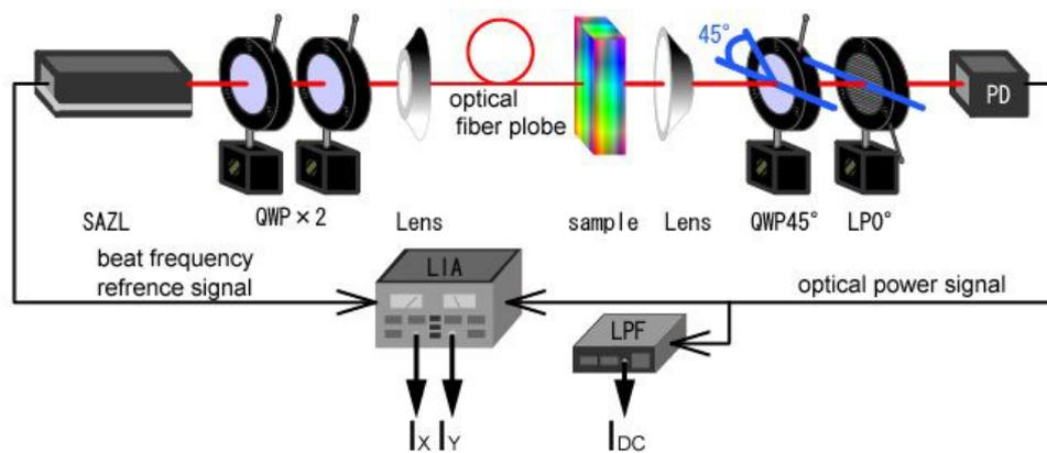
**Figure 1.** Schematic drawing of birefringence contrast scanning near-field optical microscope (B-SNOM): SAZL(Stabilized Axial Zeeman Laser); QWP(Quarter wave plate); PD(Photo detector); LPF(Low pass filter).
