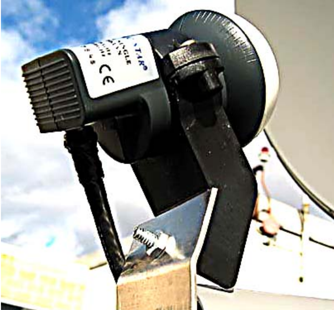
Figure 3. The connector should point down towards the ground and should be well taped to be sure water doesn't get into the connector or the attenuator to which it is attached.
