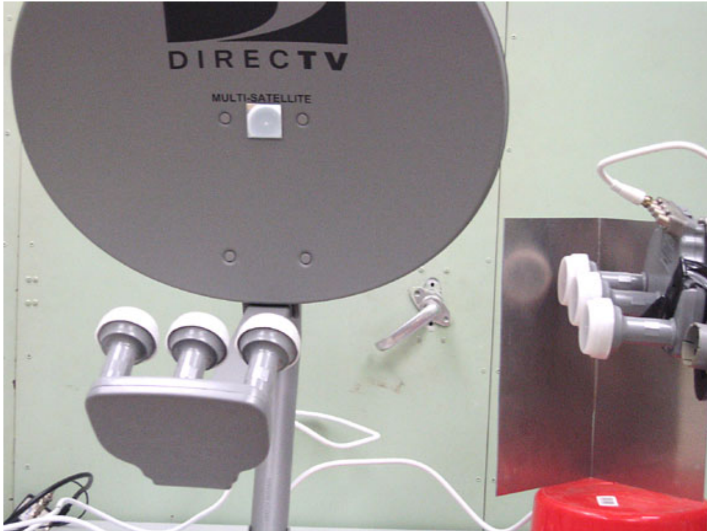
Figure 5. 2-element interferometer using DirecTV dish the view is from the CFL signal source. Note: the optical reflections of the active feed used as an initial alignment guide and LNB as a “reference” antenna.
