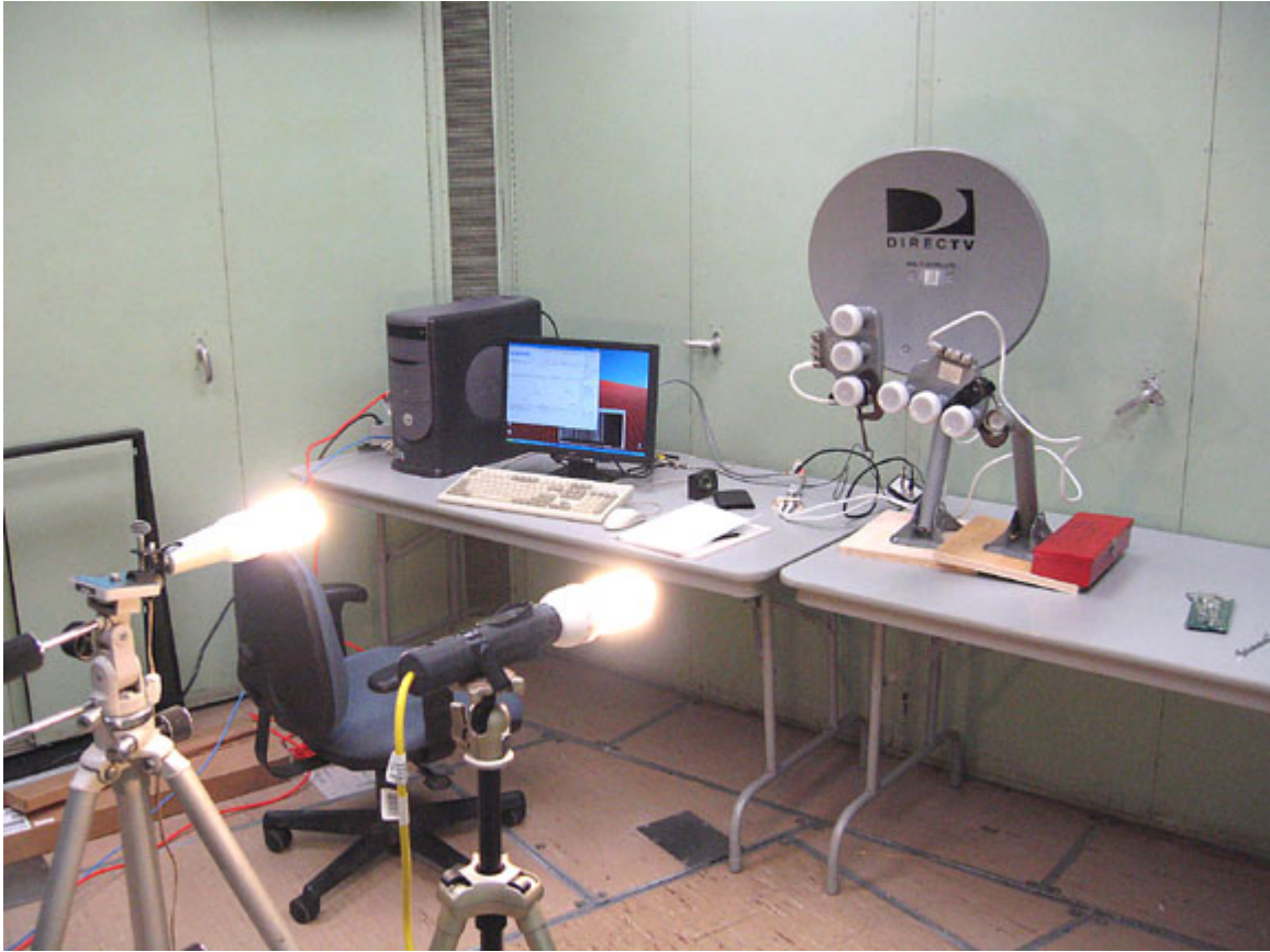
Figure 2. 2-element interferometer using LNBF's and CFL's as signal sources.
