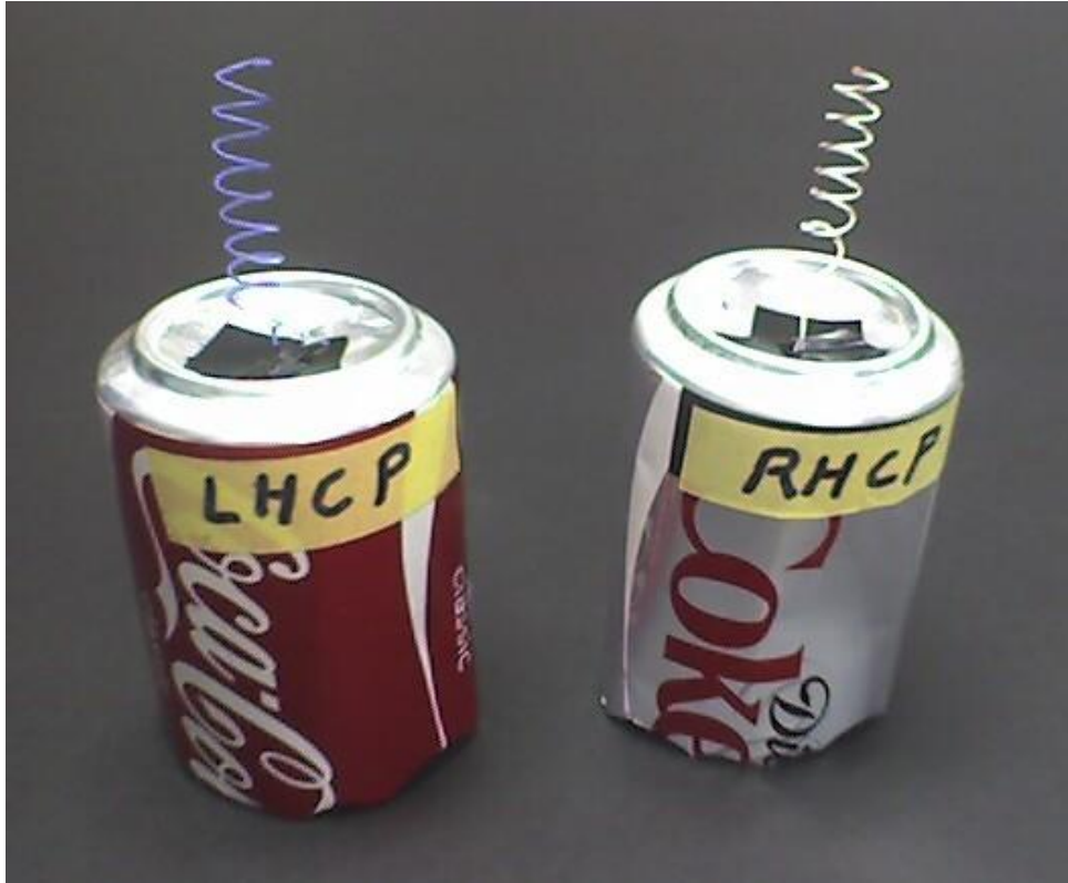
Figure 27. Standard sources of Left and Right Hand Circular Polarized Ku microwaves are used to set LNB reception for the desired signal polarization. Using the cans will cause overheating of the CFLs so experiments must be done quickly.
