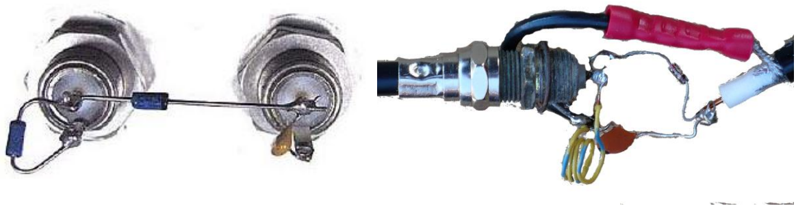
Figure 7. Photographs of two variations of the envelope detector.
