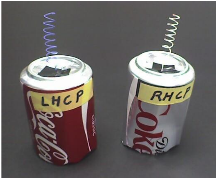
Figure 17. Cans should be chosen to fit over the CFLs and they should be labeled LHC and RHC to facilitate measurements.
